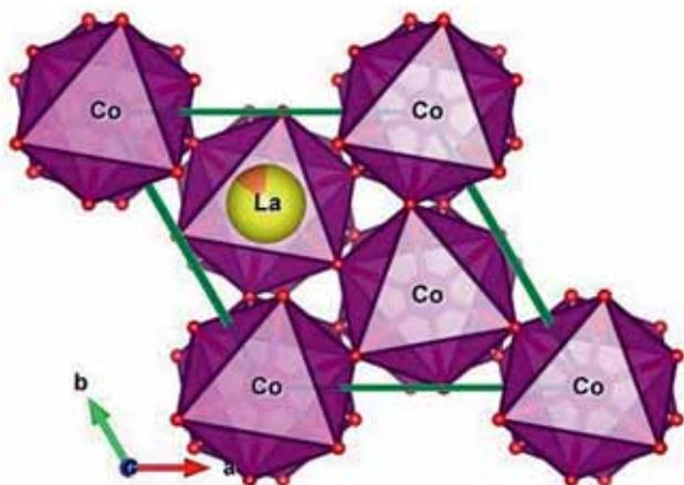
**Figure 3.** Crystal structure of  $\text{La}_{1-x}\text{Na}_x\text{CoO}_3$ .
