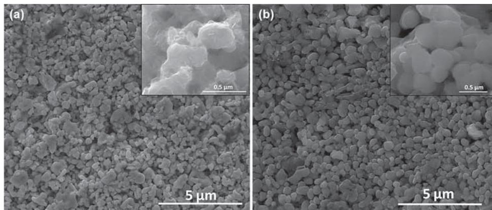
**Figure 5.** SEM images of (a) LNCO5 and (b) LNCO10 compositions.
