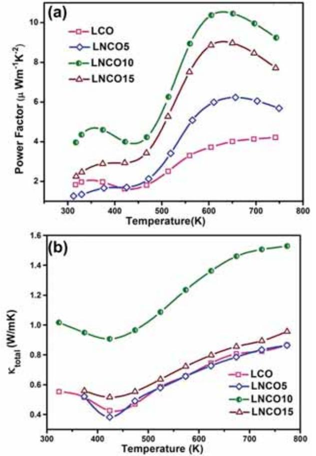
**Figure 10.** (a) Power factor and (b) the total thermal conductivity of LNCO.
