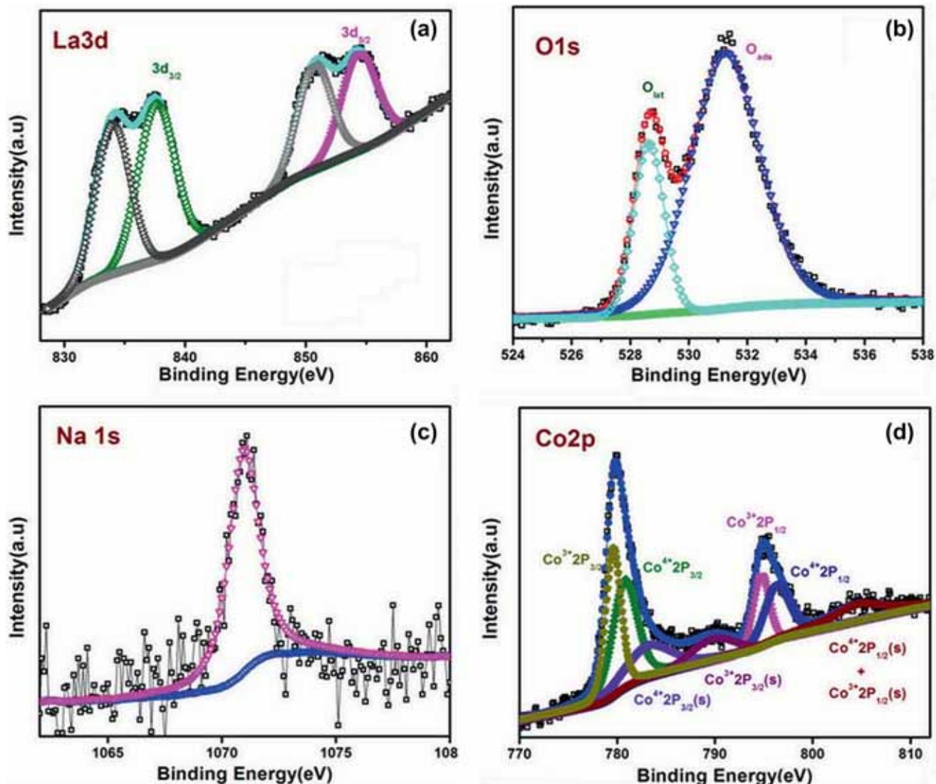
**Figure 8.** XPS spectrum of LNC05 with enlarged region of (a) La3d, (b) O1s, (c) Na1s and (d) Co2p core level spectra of LNC05.
