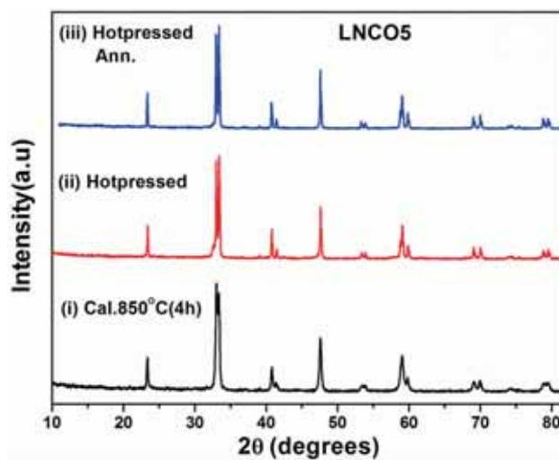
**Figure 4.** Powder XRD patterns of LNCO5 compound (i) calcination powder at  $1123$  K, (ii) powder obtained from the hot pressed pellet and (iii) annealed samples at  $973$  K.
