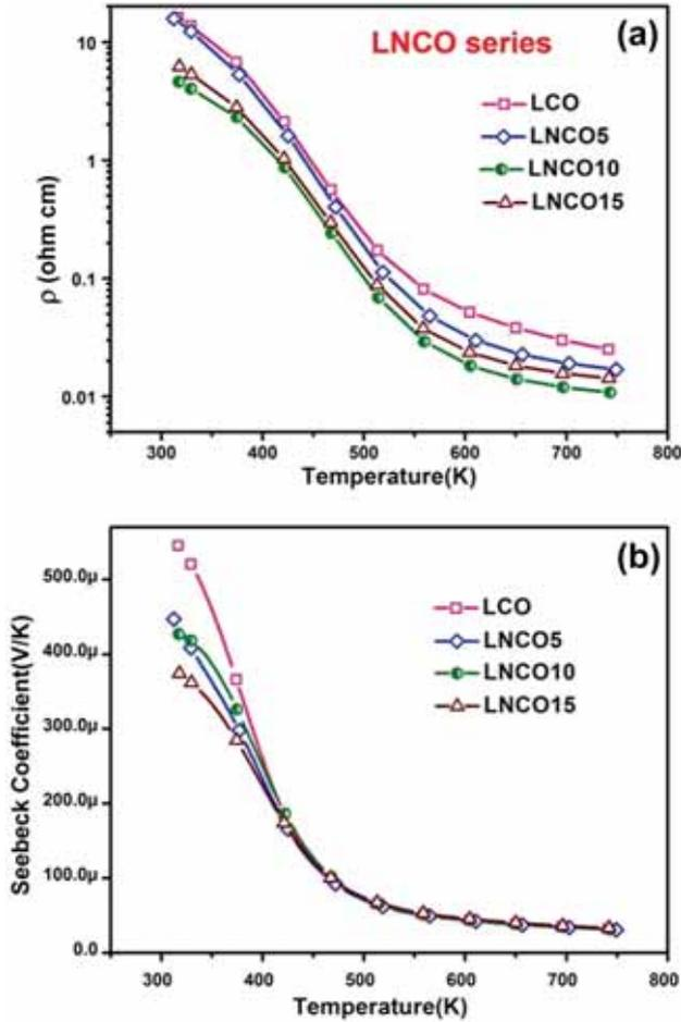
**Figure 9.** Temperature dependent study of (a) plots of electrical resistivity and (b) Seebeck coefficient of  $\text{La}_{1-x}\text{Na}_x\text{CoO}_3$  compositions.
