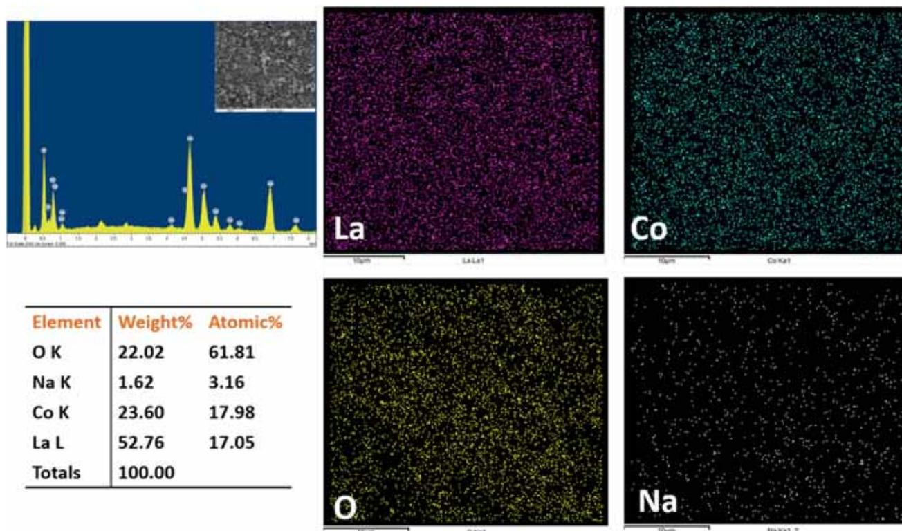
Figure 6. Elemental mapping of LNCO15 compositions.
