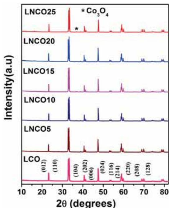
**Figure 1.** Powder XRD patterns of Na-doped  $\text{LaCoO}_3$  compounds.
