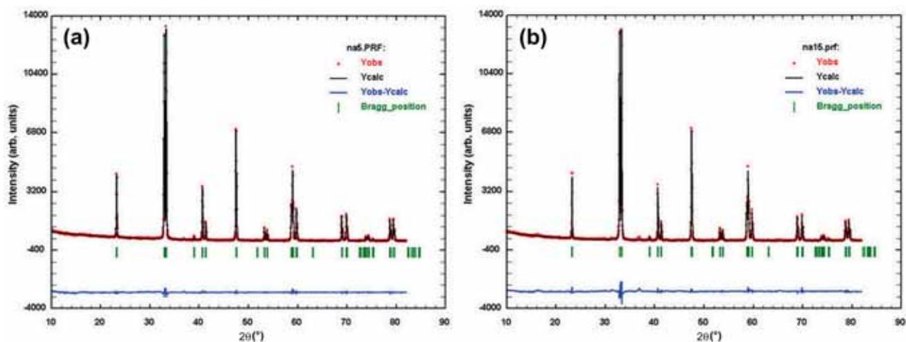
**Figure 2.** Observed, calculated and the different XRD patterns for (a) LNCO5 and (b) LNCO15.
