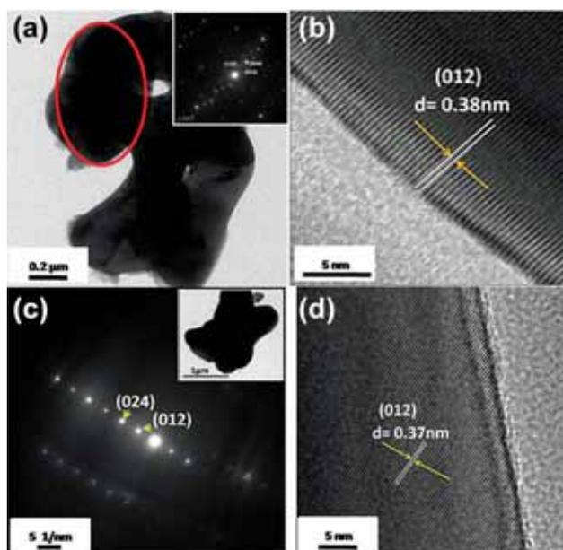
Figure 7. (a) TEM images of LCO, inset shows SAED pattern, (b) HRTEM image of LCO, (c) SAED pattern of LNCO10 and (d) HRTEM image of LNCO10.
