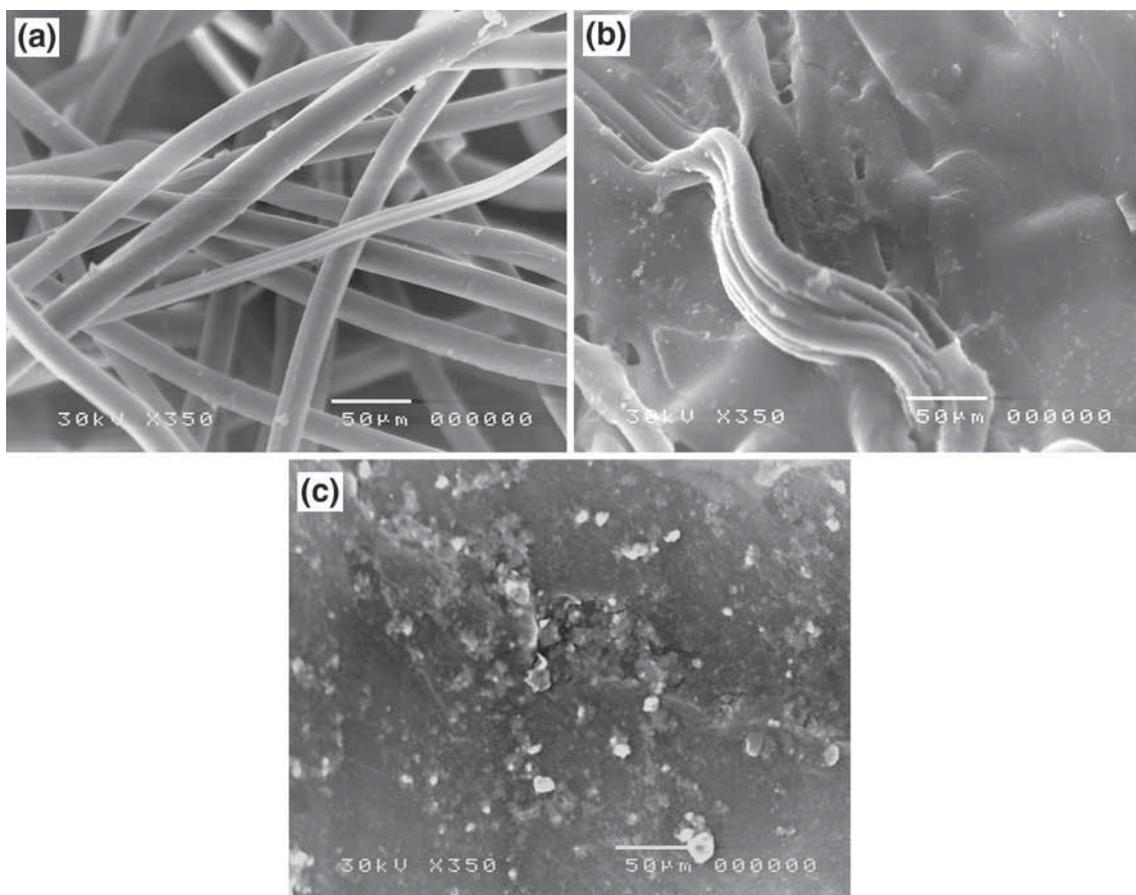
**Figure 4.** SEM images of (a) plain textile, (b) textile-g-(chitosan/HEMA) (50:50) and (c) nano-ZnO/grafted textile at 20 kGy.
