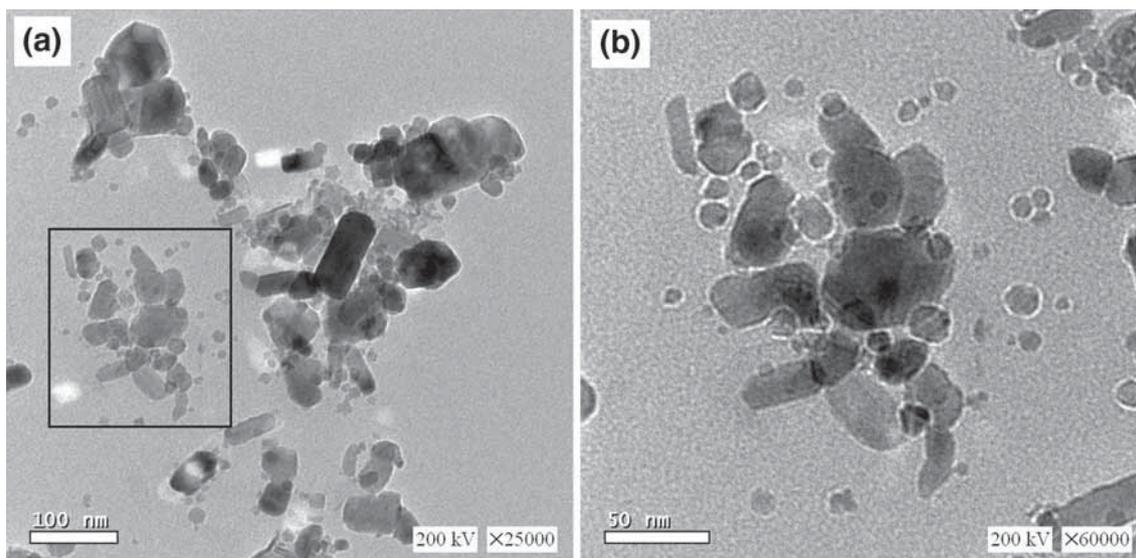
**Figure 7.** Typical TEM micrographs of nano-ZnO/grafted textile with different magnification power: (a) 25,000 and (b) 60,000.
