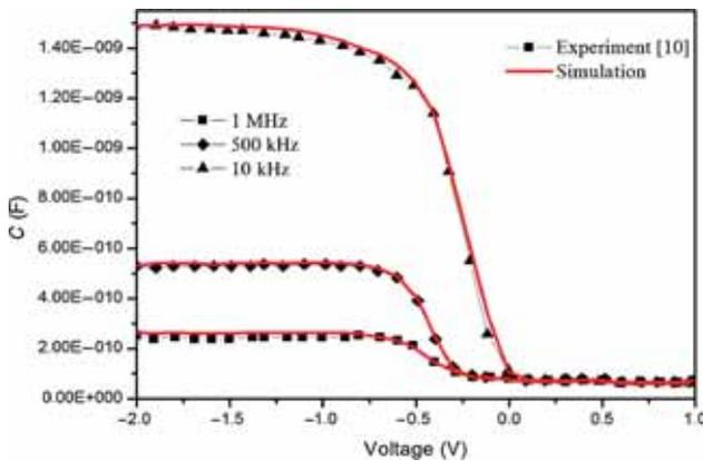
**Figure 1.** Comparison between experimental data [10] (symbol) and simulated (line)  $C-V$  curves for  $\text{Al}/\text{CeO}_2/\text{p-Si}$  MOS capacitor.
