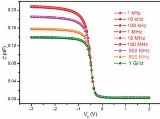
**Figure 4.** The variation of capacitance vs. voltage for different frequencies from 1 kHz to 1 GHz ( $T_{\text{Al}_2\text{O}_3} = 5 \text{ nm}$ ,  $N_A = 1e16 \text{ cm}^{-3}$ ).
