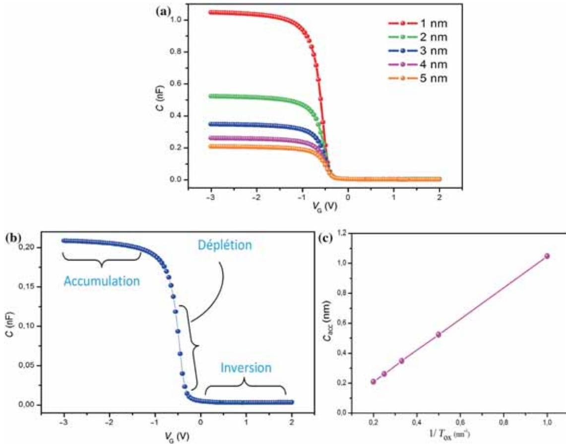
**Figure 2.** (a)  $C$ – $V$  characteristics of the MIS structure for different thicknesses of  $\text{Al}_2\text{O}_3$ . (b) High-frequency  $C$ – $V$  curves for  $T_{\text{ox}} = 5$  nm,  $N_A = 1 \times 10^{16} \text{ cm}^{-3}$  with the different regimes at room temperature. (c) Variation of the accumulation capacitance  $C_{\text{acc}}$  vs. different thicknesses of  $\text{Al}_2\text{O}_3$ .
