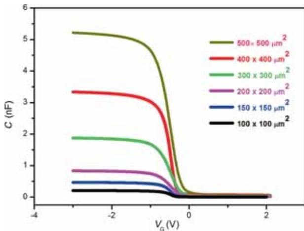
**Figure 3.** Variation of capacitance vs. voltage for different surfaces at a high frequency of 1 kHz and a silicon doping value  $N_A = 1 \times 10^{16} \text{ cm}^{-3}$ .
