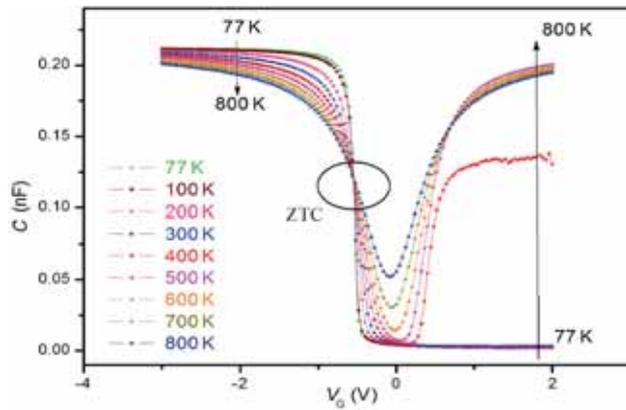
**Figure 5.** High-frequency  $C-V$  curves for  $T_{\text{ox}} = 5 \text{ nm}$  and  $N_A = 1e16 \text{ cm}^{-3}$  with surface area of  $100 \times 100 \mu\text{m}^2$  for a range of temperatures  $T = [77-800] \text{ K}$ .
