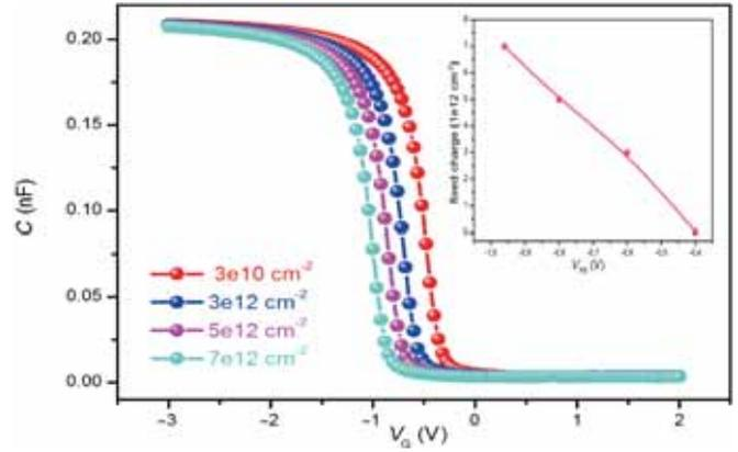
**Figure 6.**  $C-V$  characteristics for different values of fixed charge  $Q_f$  at the interface of  $\text{Al}_2\text{O}_3/\text{p-Si}$ . Inset: Variation of the fixed charge vs. the flat-band voltage  $V_{\text{FB}}$ .
