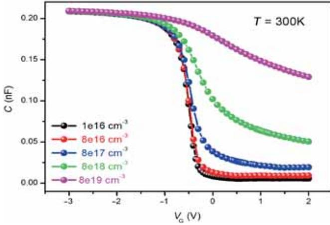
**Figure 7.** Variation of capacity as a function of voltage for different values of the substrate doping.
