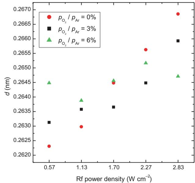
**Figure 4.** Dependence of calculated  $d$ -spacing values for the deposited AZO thin films on rf power density  $P$  for different values of oxygen partial pressure,  $OPP$ .
