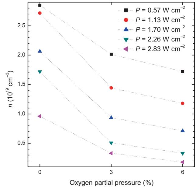
**Figure 10.** Dependence of calculated carrier concentration  $n$  of the studied AZO films prepared at different rf power densities on *OPP*.
