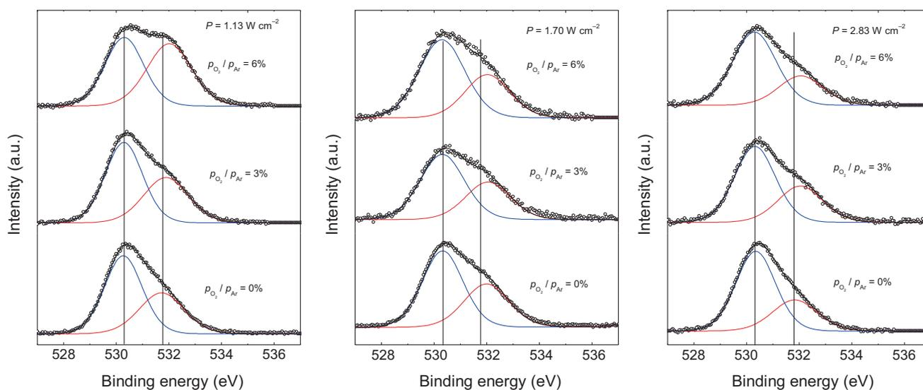
**Figure 5.** The O  $1s$  core peak for different oxygen partial pressure values ( $OPP=0, 3$  and  $6\%$ ) at three different rf power density values ( $P = 1.13, 1.70$  and  $2.83 \text{ W cm}^{-2}$ ). All peaks have been deconvoluted into two components. Two lines are drawn at  $530.3$  and  $531.8 \text{ eV}$  for guidance.
