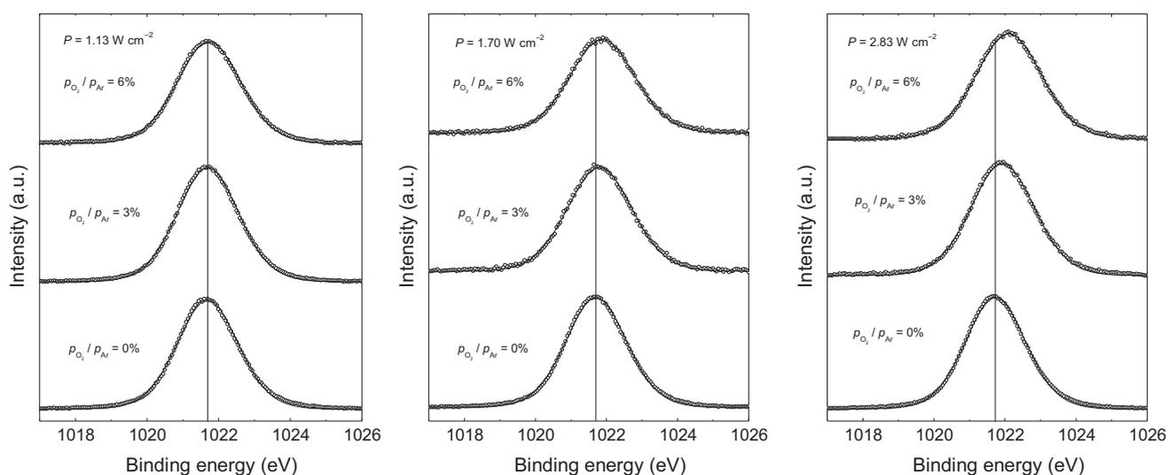
**Figure 6.** The Zn  $2p_{3/2}$  core peak for different oxygen partial pressure values ( $OPP=0, 3$  and  $6\%$ ) at three different rf power density values ( $P = 1.13, 1.70$  and  $2.83 \text{ W cm}^{-2}$ ).
