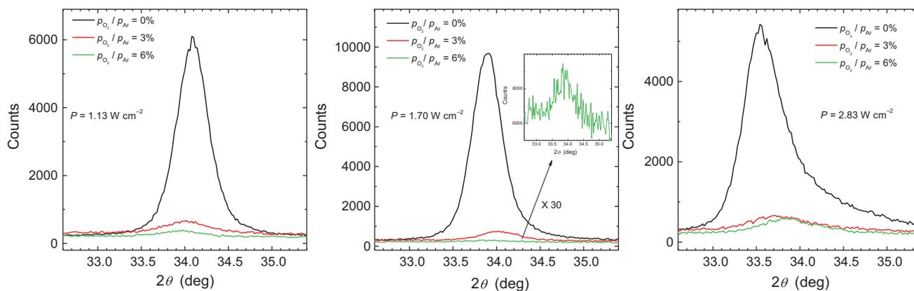
**Figure 2.** X-ray diffraction measurements on AZO thin films grown at different rf power density values  $P$  and different values of oxygen partial pressure,  $OPP$ .
