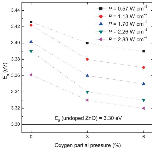
**Figure 9.** Dependence of obtained band gap values for AZO films prepared at different rf power densities on *OPP*.
