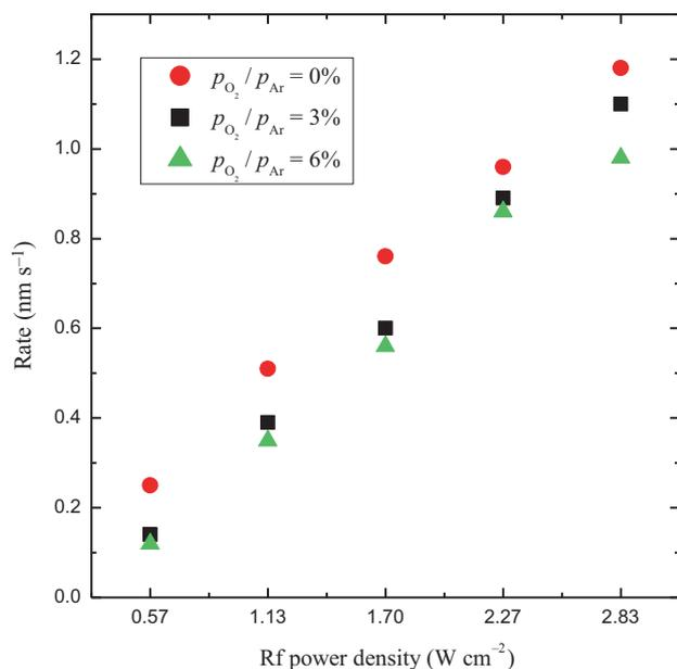
**Figure 1.** Deposition rate as a function of rf power density  $P$  at different values of oxygen partial pressure,  $OPP$ .
