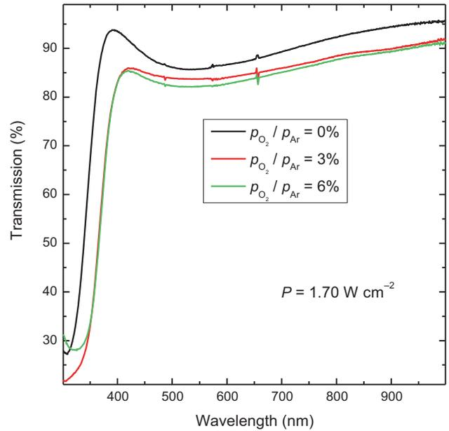
**Figure 8.** Optical transmission spectra of AZO thin films grown at rf power density of  $P = 1.70 \text{ W cm}^{-2}$  with different oxygen partial pressure values,  $OPP$ .
