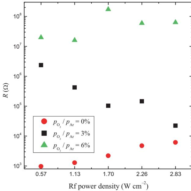
**Figure 7.** Dependence of  $\log R$  on rf power density for AZO thin films prepared at different oxygen partial pressure values,  $OPP$ .
