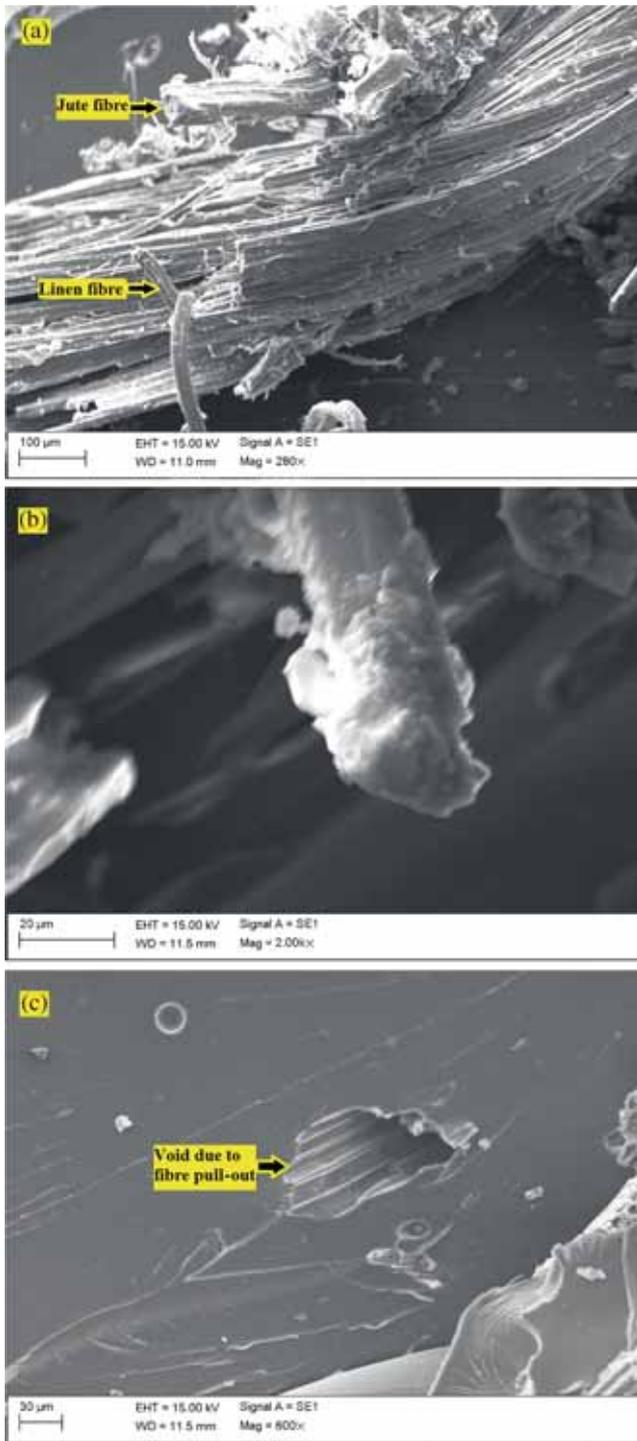
**Figure 8.** SEM micrographs of J2-L3 laminate composite after tensile test: (a) fractured surface, (b) fractured fibre and (c) void due to fibre pull-out.
