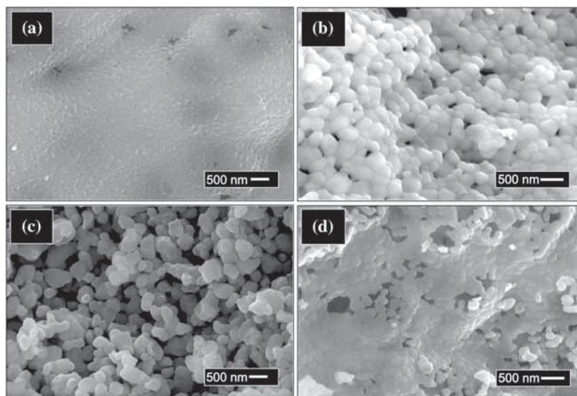
**Figure 3.** SEM micrographs of  $\text{LiNbO}_3$  powders synthesized by combustion reactions (a) R1, (b) R2, (c) R3 and (d) R4.
