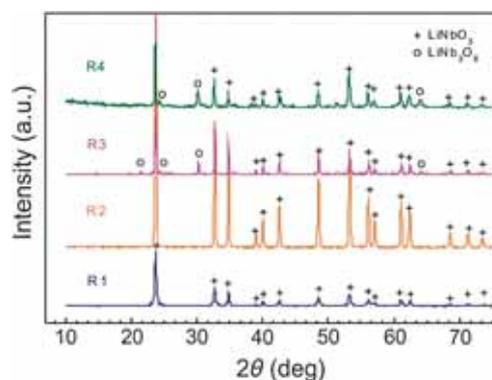
**Figure 2.** XRD patterns of the  $\text{LiNbO}_3$  powders synthesized in the different combustion reactions.
