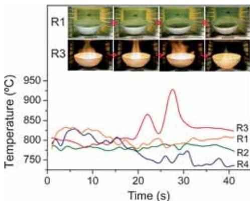
**Figure 1.** Temperature against time during the different stages of the combustion reaction. The insets show a sequence of digital images recorded during the combustion.
