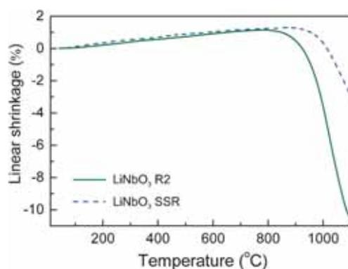
**Figure 6.** Dilatometric curves of the LiNbO<sub>3</sub> green pellets.
