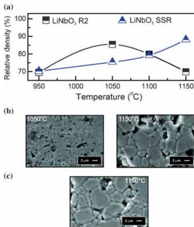
**Figure 7.** (a) Comparative densification curves for powders synthesized by combustion method and solid-state reaction. SEM micrographs are presented for (b) LiNbO<sub>3</sub> R2 at 1050 and 1150°C and (c) LiNbO<sub>3</sub> SSR polycrystalline samples at 1150°C.
