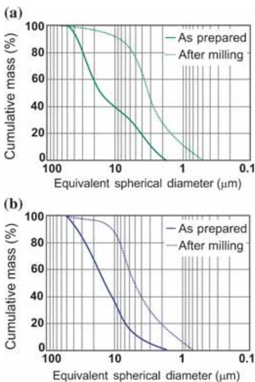
**Figure 5.** Particle size distribution of the powders: (a) LiNbO<sub>3</sub> R2 and (b) LiNbO<sub>3</sub> SSR.
