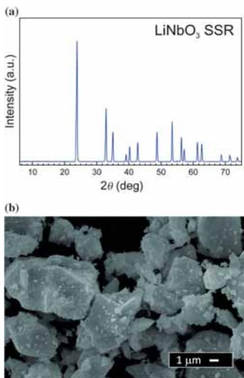
**Figure 4.** (a) XRD pattern of the  $\text{LiNbO}_3$  powder synthesized by solid-state reaction and (b) SEM image of the powder.
