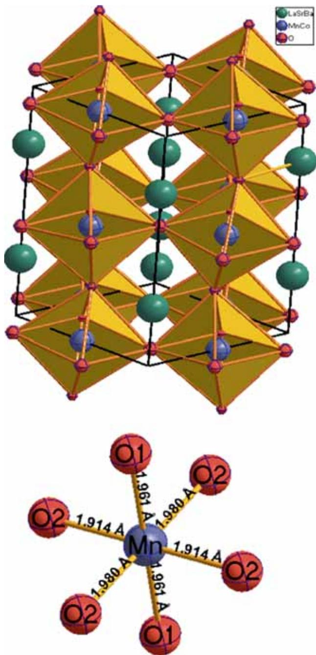
**Figure 2.** View of the orthorhombic (Pnma) crystal structure of  $\text{La}_{0.67}\text{Sr}_{0.22}\text{Ba}_{0.11}\text{MnO}_3$  and the coordination polyhedron of Mn displaying the Mn–O distances.
