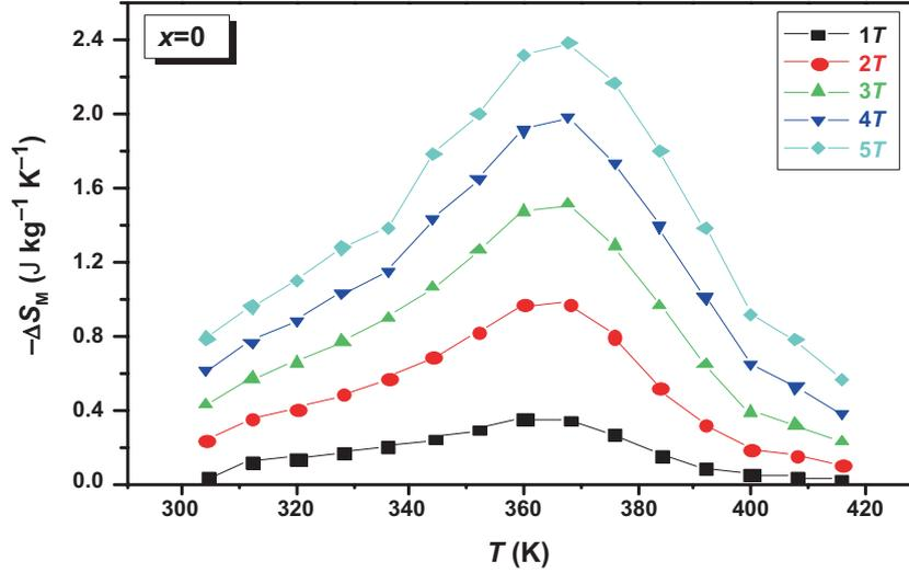
**Figure 6.** Thermal evolution of the entropy under different amplitudes of change in the magnetic field (from bottom to top,  $\Delta H = 1, 2, 3, 4$  and  $5$  T) for the  $\text{La}_{0.67}\text{Sr}_{0.22}\text{Ba}_{0.11}\text{MnO}_3$  sample.
