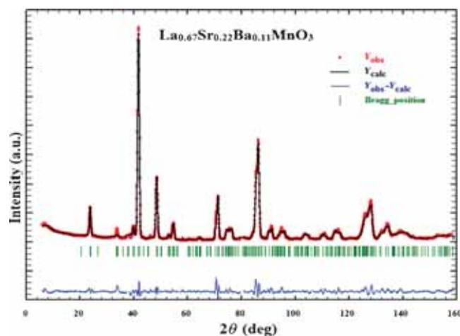
**Figure 1.** Observed (crosses), calculated (full line) and difference (bottom) NPD rietveld profiles for  $\text{La}_{0.67}\text{Sr}_{0.22}\text{Ba}_{0.11}\text{Mn}_{0.9}\text{Co}_{0.1}\text{O}_3$  at 298 K. Vertical lines correspond to the Bragg positions.
