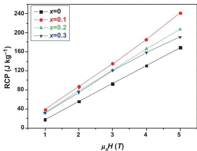
**Figure 7.** Relative cooling power values (RCP) vs. applied magnetic field for La<sub>0.67</sub>Sr<sub>0.22</sub>Ba<sub>0.11</sub>Mn<sub>1-x</sub>Co<sub>x</sub>O<sub>3</sub> (0 ≤ x ≤ 0.3) compounds.
