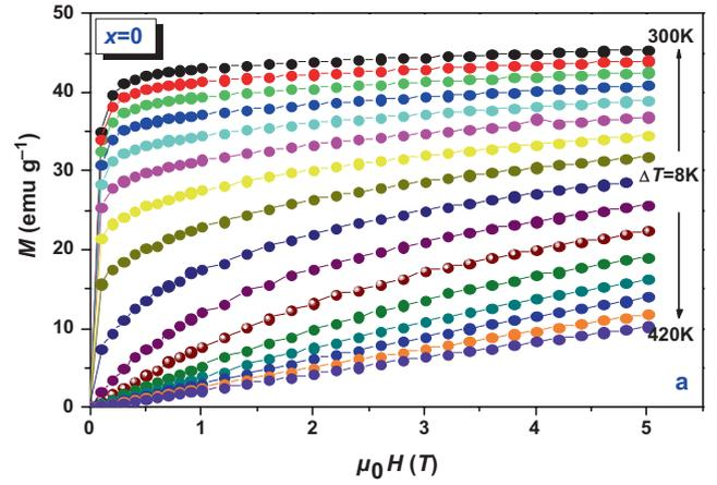
**Figure 5.** Magnetization vs. field isotherms near  $T_C$  for the  $\text{La}_{0.67}\text{Sr}_{0.22}\text{Ba}_{0.11}\text{MnO}_3$  sample.
