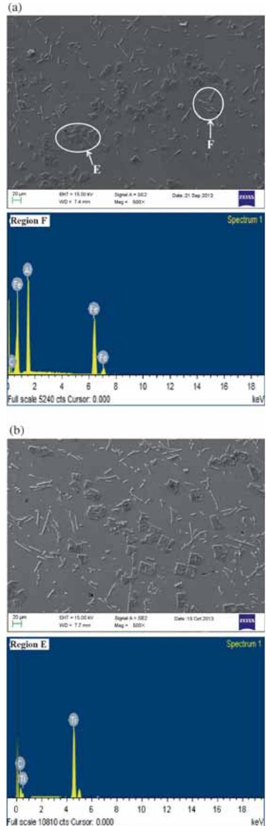
**Figure 3.** SEM micrographs and EDS analysis of carbides of (a) Alloy-3 with cuboid TiC (region E) and elongated  $Fe_3AlC_{0.5}$  carbide particles (region F) and (b) Alloy-4 with similar carbide particles.
