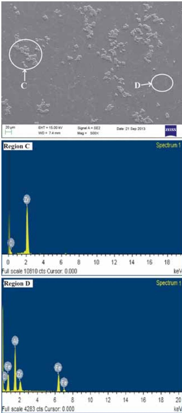
**Figure 2.** SEM micrographs and EDS analysis of carbides of Alloy-2 with cuboid ZrC (region C) and Laves phase  $Zr(FeAl)_2$  (region D).
