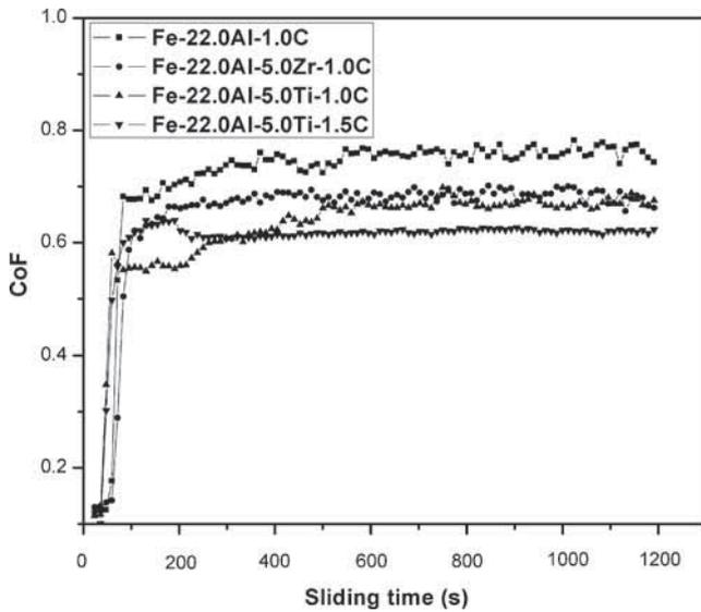
**Figure 6.** The variation of coefficient of friction (CoF) with time for FeAl-based alloys at applied load 10 N with sliding speed  $0.21 \text{ m s}^{-1}$ .
