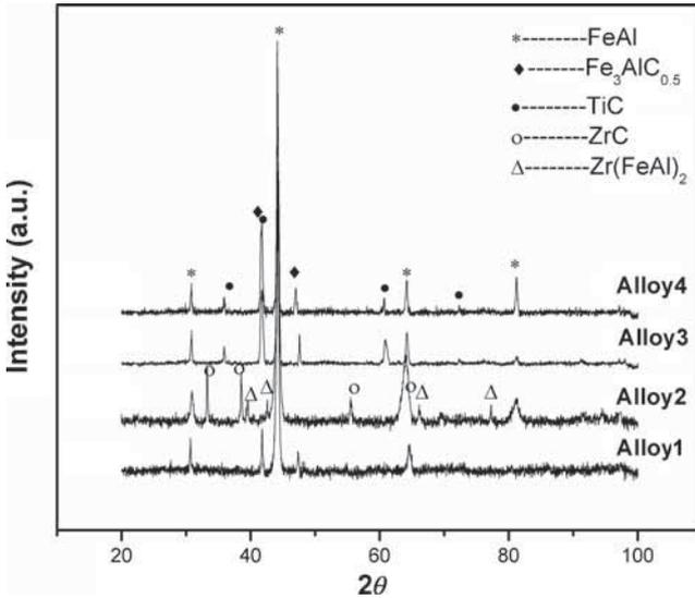
**Figure 4.** XRD patterns obtained from all FeAl-based alloys.
