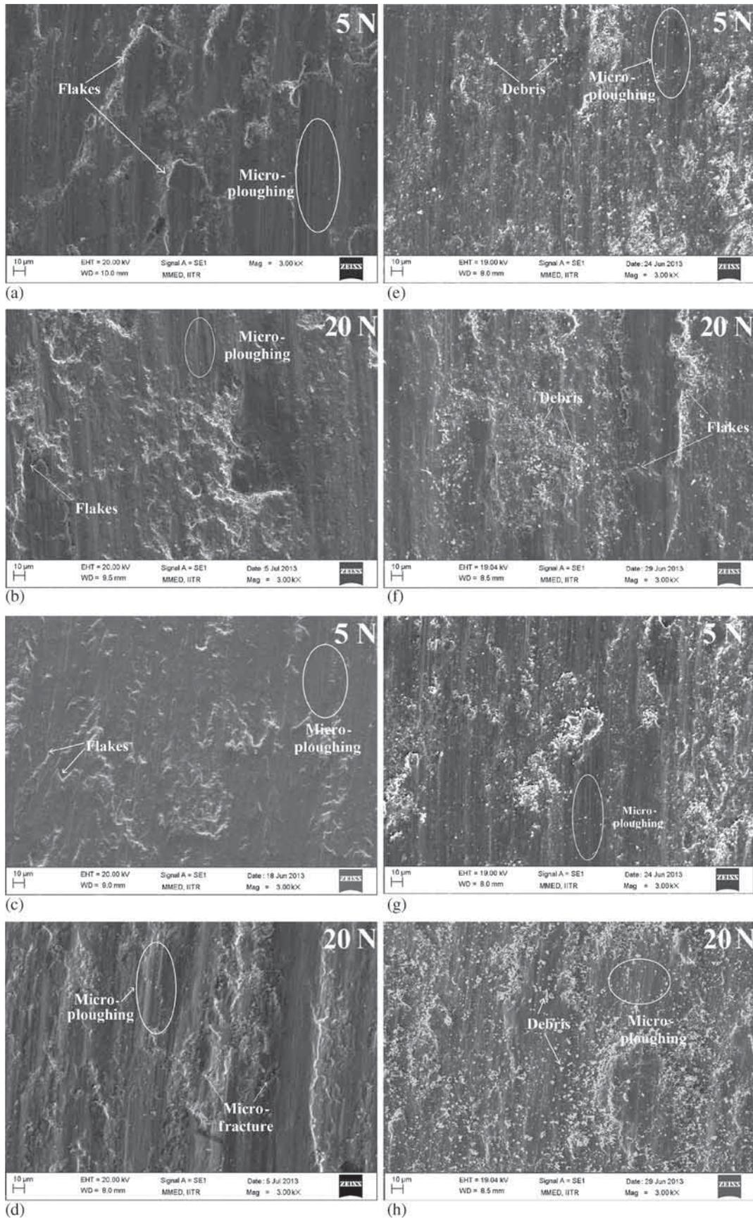
**Figure 8.** SEM micrographs showing morphologies of wear tracks for (a, b) Alloy-1, (c, d) Alloy-2, (e, f) Alloy-3 and (g, h) Alloy-4 at applied load 5 and 20 N with sliding speed  $0.21 \text{ m s}^{-1}$ .
