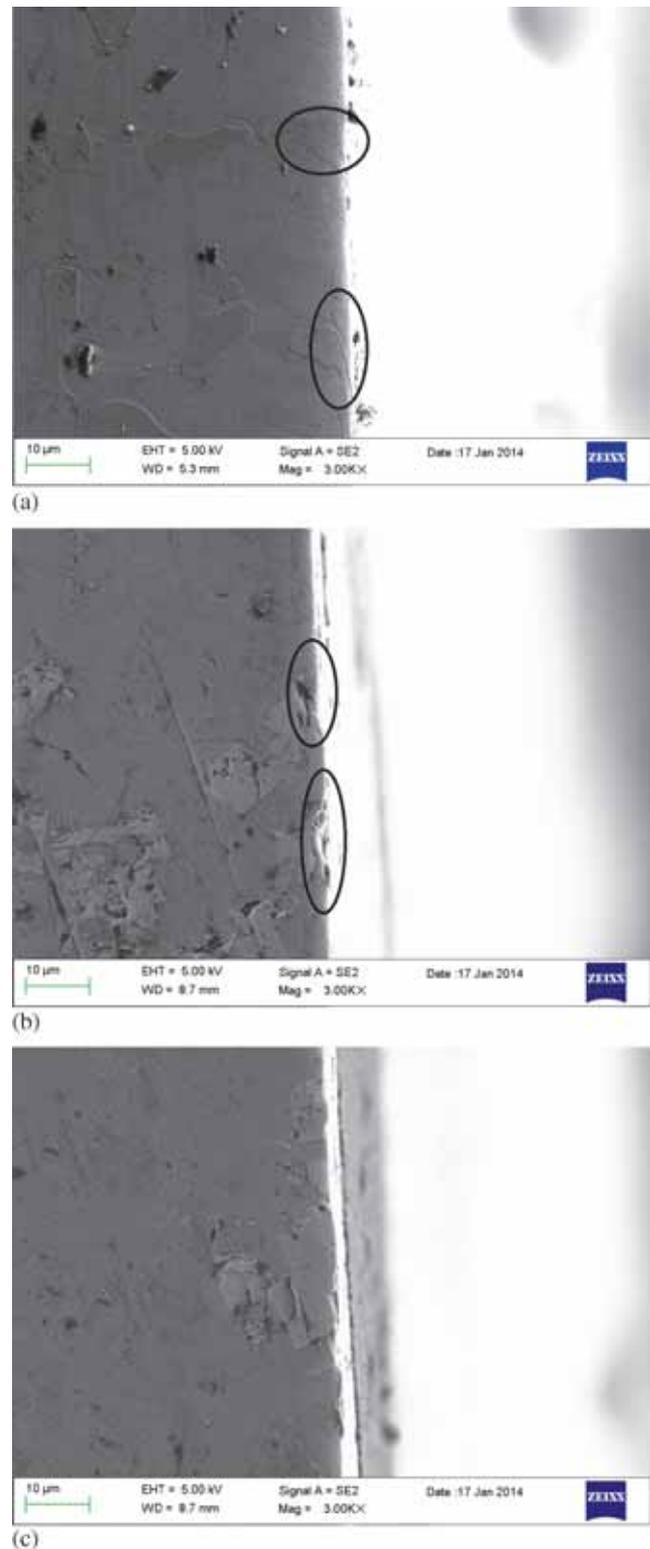
**Figure 7.** Cross-section of wear tracks of (a) Alloy-1, (b) Alloy-2 and (c) Alloy-3 showing different carbides embedded in matrix after sliding wear.
