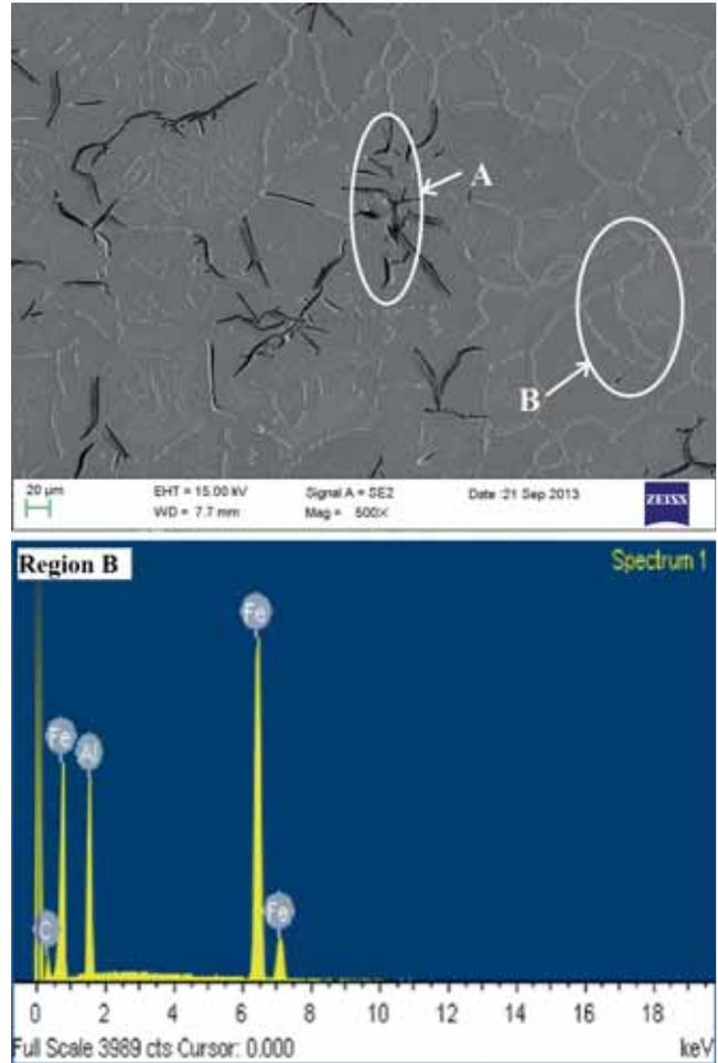
**Figure 1.** SEM micrographs and EDS analysis of carbides of Alloy-1 with network structure of graphite flakes (region A) and Fe<sub>3</sub>AlC<sub>0.5</sub> carbides (region B).
