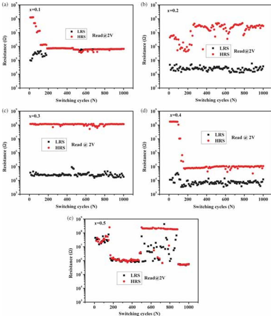
**Figure 5.** The reading endurance and stability of the  $\text{Ag}/\text{La}_{1-x}\text{Zn}_x\text{MnO}_3/\text{p}^+\text{-Si}$  devices.
