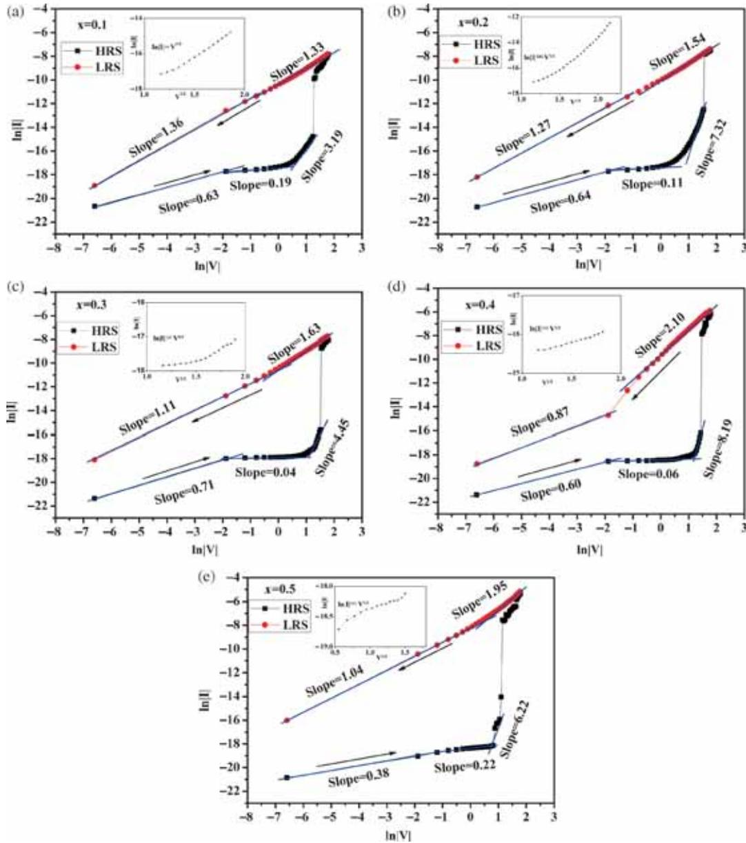
**Figure 4.** Linear fitting for the  $I$ - $V$  curve of the  $\text{Ag}/\text{La}_{1-x}\text{Zn}_x\text{MnO}_3/\text{p}^+\text{-Si}$  in  $\ln$ - $\ln$  scale and corresponding slopes for each portion.
