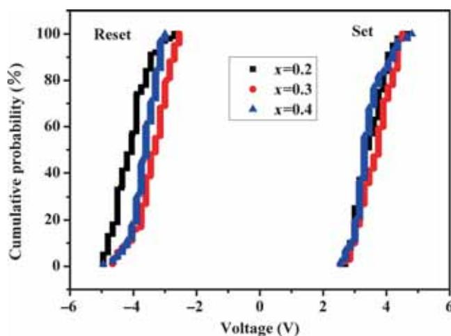
**Figure 6.** The cumulative probabilities of the set and reset voltages of Ag/La<sub>1-x</sub>Zn<sub>x</sub>MnO<sub>3</sub>/p<sup>+</sup>-Si during the 1000 resistive switching cycles.
