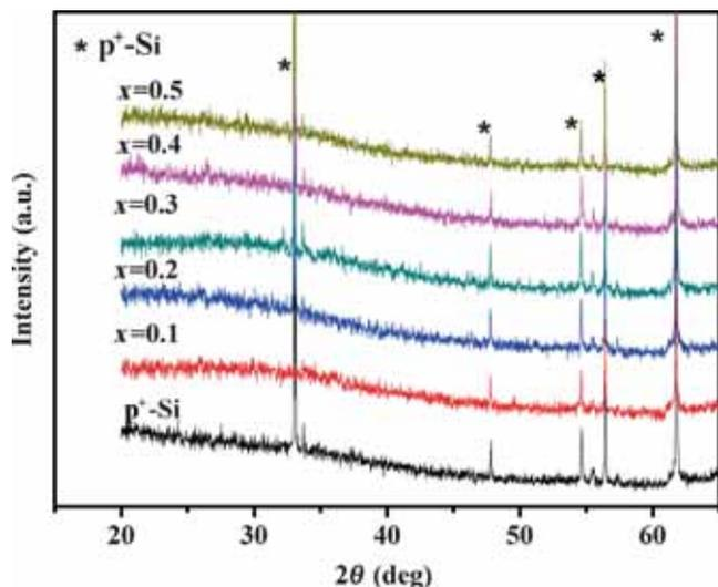
**Figure 1.** XRD patterns of the  $\text{La}_{1-x}\text{Zn}_x\text{MnO}_3/\text{p}^+\text{-Si}$  heterojunction and the  $\text{p}^+\text{-Si}$ .
