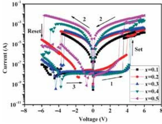
**Figure 3.**  $I$ - $V$  curves of the  $\text{Ag}/\text{La}_{1-x}\text{Zn}_x\text{MnO}_3/\text{p}^+\text{-Si}$  devices in semi-logarithmic scales.
