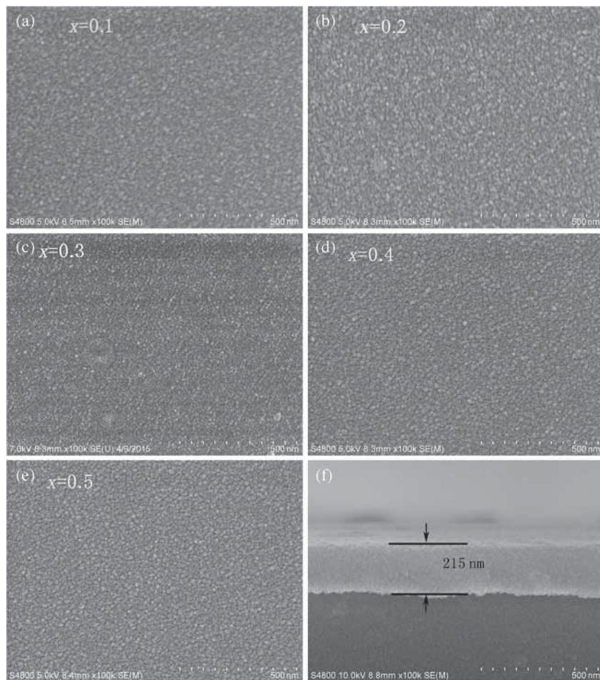
**Figure 2.** SEM images of (a–e) surface and (f) cross-section morphology of the  $\text{La}_{1-x}\text{Zn}_x\text{MnO}_3/\text{p}^+\text{-Si}$ .
