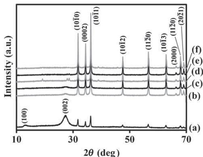
**Figure 1.** XRD patterns of samples at the  $M/Z$  ratios of (a) 50, (b) 10, (c) 5, (d) 2.5, (e) 1.67 and (f) 1, after being calcined at  $540^\circ C$  for 3 h in air. The three and four Miller indices correspond to the  $C_3N_4$  and ZnO phases, respectively.
