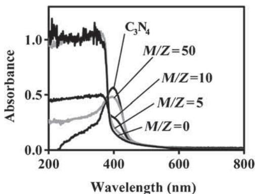
**Figure 8.** Absorption spectra of pure  $C_3N_4$  and the samples at  $M/Z$  ratios of 50, 10, 5 and 0 (pure ZnO) after being calcined at  $540^\circ C$  for 3 h in air.
