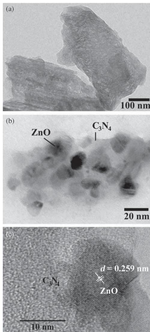
**Figure 6.** TEM images of (a) pure  $\text{C}_3\text{N}_4$  and (b) sample at the  $M/Z$  ratio of 10, and (c) HR-TEM image of sample at the  $M/Z$  ratio of 10.
