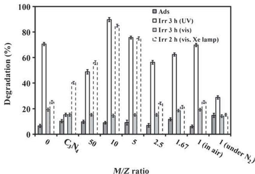
**Figure 9.** Photocatalytic activity of pure  $C_3N_4$  and samples at the  $M/Z$  ratios of 0, 50, 10, 5, 2.5, 1.67 and 1, after being calcined at  $540^\circ\text{C}$  for 3 h in air. The last one is the photocatalytic activity of the sample at the  $M/Z$  ratio of 1 after being calcined at  $540^\circ\text{C}$  for 3 h in  $N_2$ .  $M/Z = 0$  refers to pure ZnO.
