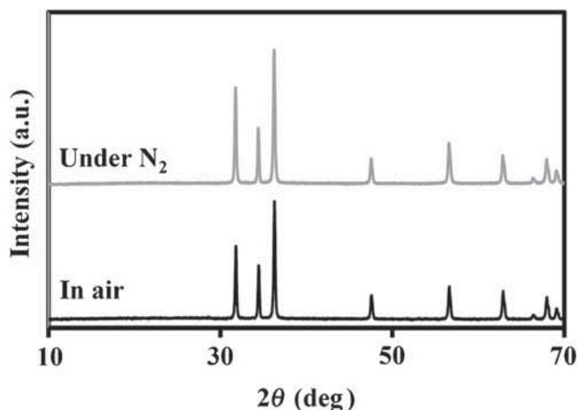
**Figure 2.** XRD patterns of samples at the  $M/Z$  ratio of 1, after being calcined at  $540^\circ\text{C}$  for 3 h in air and in  $N_2$  atmosphere.
