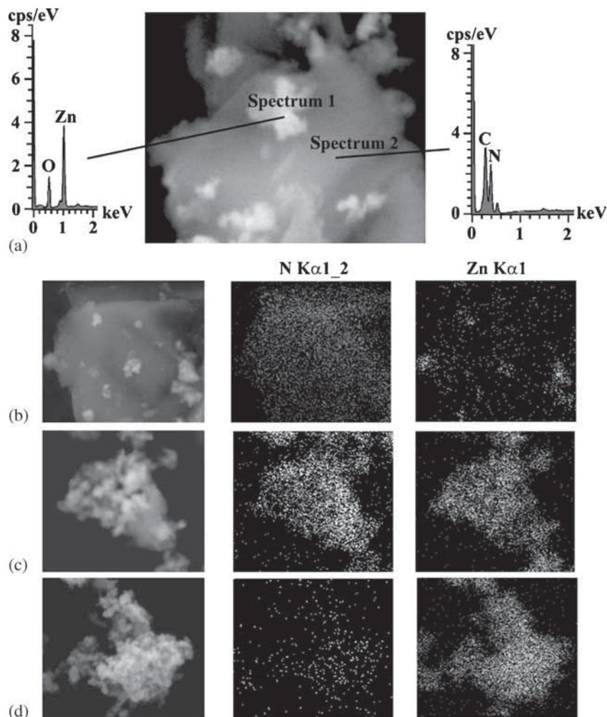
**Figure 7.** The corresponding (a) EDS spectra of  $C_3N_4/ZnO$  and EDS mapping of samples at  $M/Z$  ratios of (b) 50, (c) 5 and (d) 2.5, after being calcined at  $540^\circ C$  for 3 h in air.
