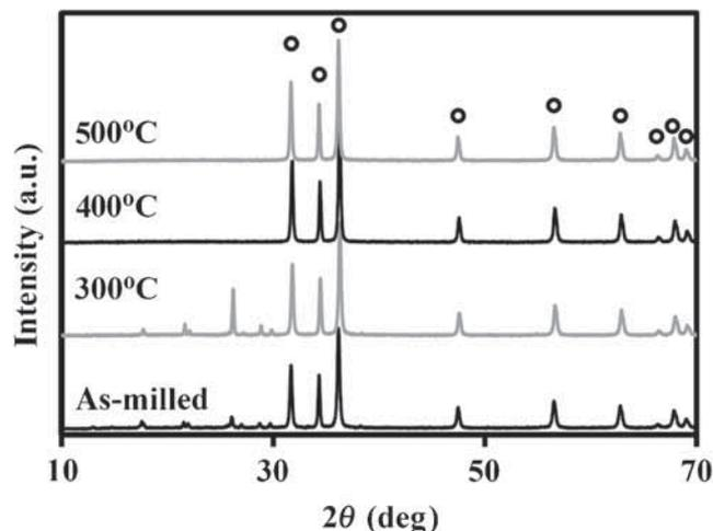
**Figure 3.** XRD patterns of samples at the  $M/Z$  ratio of 1 before and after being calcined at various temperatures for 3 h in air. The circle symbols represent ZnO phase.
