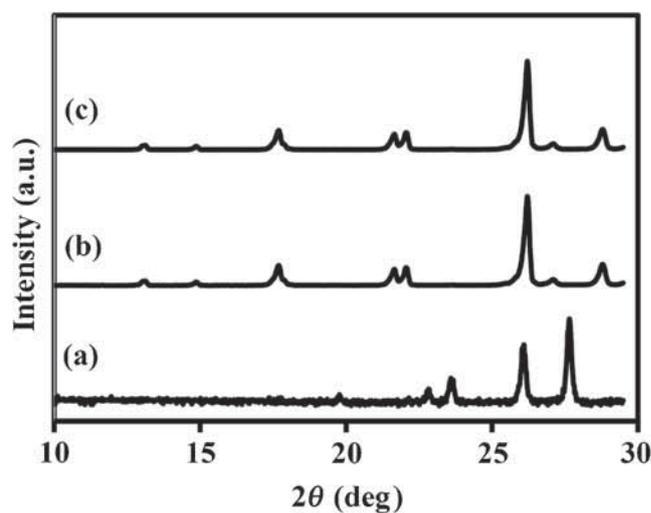
**Figure 4.** XRD patterns of powder at the bottom of the crucible for samples at (a)  $M/Z = 1$  as well as (b) pure melamine and (c) the typical XRD of the powder at the upper inner sidewall of the crucible for samples at  $M/Z = 1$  and pure melamine. The samples were heated at  $350^\circ\text{C}$  for 3 h.
