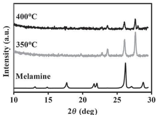
**Figure 5.** XRD patterns of samples containing 0.5 g of melamine and 0.5 g of  $\text{Na}_2\text{CO}_3$  after being calcined at different temperatures for 3 h. For  $350^\circ\text{C}$ , it is an XRD of powder in the bottom of crucible.
