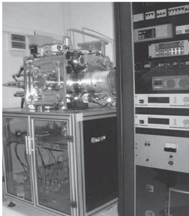
**Figure 2.** Vaksis RF-magnetron sputtering system.
