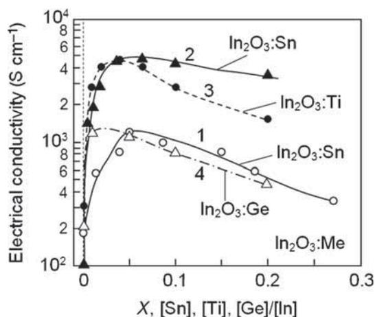
**Figure 2.** 1— $\text{In}_2\text{O}_3:\text{Sn}$  deposited by spray pyrolysis ( $T_{\text{pyr}} = 350^\circ\text{C}$ ); 2, 3— $\text{In}_2\text{O}_3:\text{Sn}$  and  $\text{In}_2\text{O}_3:\text{Ti}$  prepared using solid reaction route and then sintered ( $T_{\text{sint}} = 1400^\circ\text{C}$ ,  $t = 48$  h, air) [10]; 4— $\text{In}_2\text{O}_3:\text{Ge}$  samples were sintered in air at  $T_{\text{sint}} = 1300^\circ\text{C}$  ( $t = 48$  h) [11].
