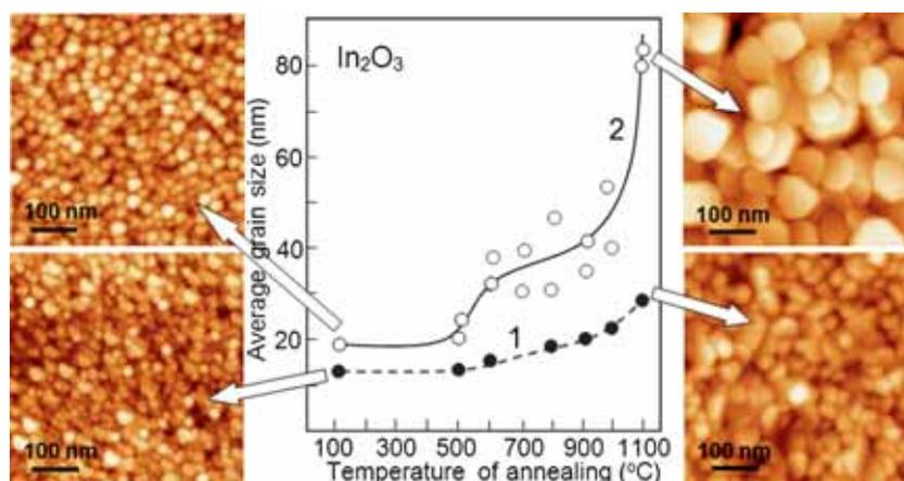
**Figure 5.** Dependences illustrating the influence of annealing on the average crystallite size in the  $\text{In}_2\text{O}_3$  films deposited by spray pyrolysis at  $T = 520^\circ\text{C}$ , and AFM images of these films after deposition and after annealing at  $1100^\circ\text{C}$ : 1— $d \sim 50$  nm, 2— $d \sim 200$  nm.
