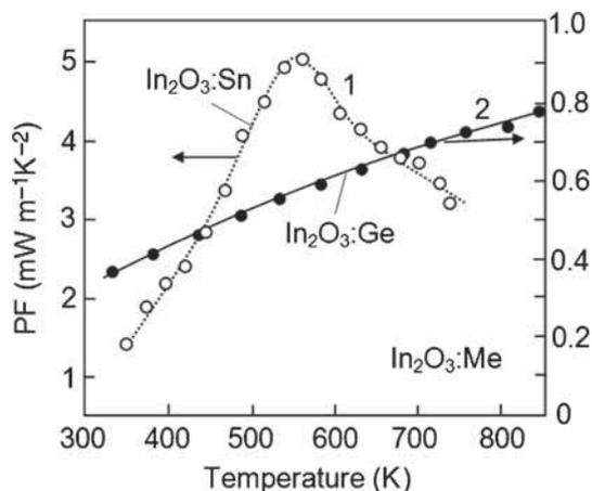
**Figure 6.** Experimental values of power factor as a function of temperature for (1)  $\text{In}_2\text{O}_3:\text{Sn}$  (5%) and (2)  $\text{In}_2\text{O}_3:\text{Ge}$  (5%) films.  $\text{In}_2\text{O}_3:\text{Sn}$  (5%) were deposited at  $T_{\text{pyr}} = 350^\circ\text{C}$ .  $\text{In}_2\text{O}_3:\text{Ge}$  samples were prepared using standard solid reaction route ( $T_{\text{sint}} = 1300^\circ\text{C}$ ,  $t = 48$  h in air) [12].
