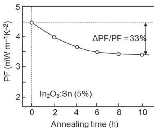
**Figure 4.** Instability of the power factor measured for  $\text{In}_2\text{O}_3:\text{Sn}$  (5% Sn) during thermal treatment in air at  $T_{\text{an}} = 700^\circ\text{C}$ .  $\text{In}_2\text{O}_3:\text{Sn}$  films were deposited at  $T_{\text{pyr}} = 350^\circ\text{C}$ .
