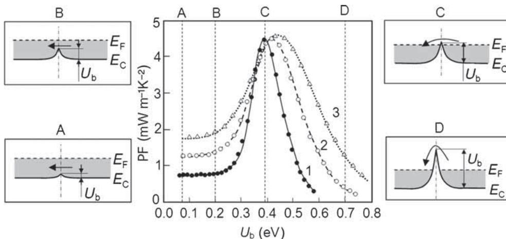
**Figure 3.** Modelled power factor of ITO as function of potential barriers at the intergrain interface at various temperatures (1— $T = 100^\circ\text{C}$ , 2— $300^\circ\text{C}$ , 3— $500^\circ\text{C}$ ). Fermi level position  $E_F = 0.35$  eV.
