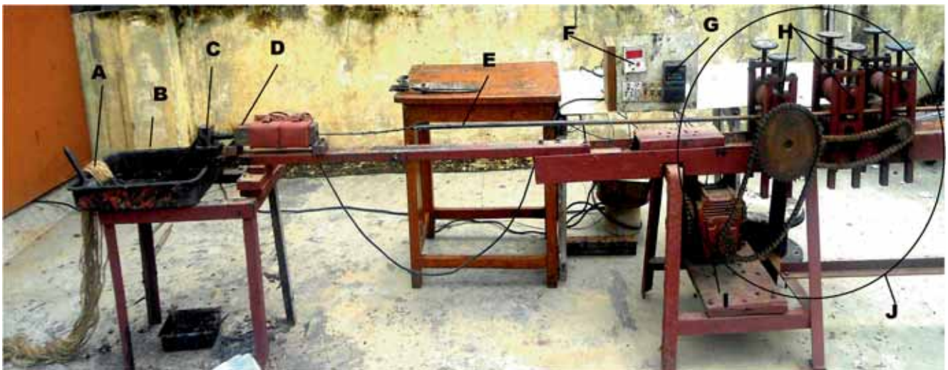
Figure 1. Indigenously developed pultrusion setup. A: jute fibre; B: resin bath; C: pre-former (cold die); D: heating die; E: steel strip for initial pulling; F: temperature controller; G: A.C. frequency drives for speed control; H: pulling roller; I: speed reducer gear box; J: pulling mechanism assembly.
