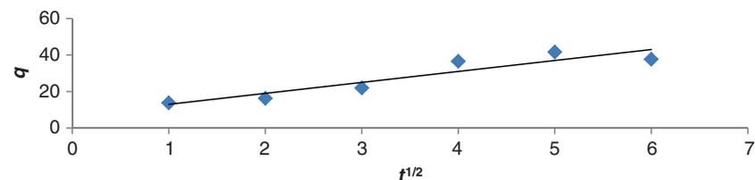
**Figure 9.** Intraparticle diffusion model kinetics for removal of Cr(VI) by composite.
