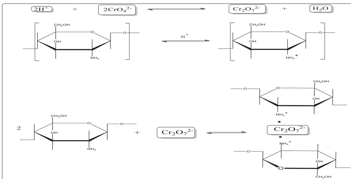
**Figure 16.** Mechanism of Cr(VI) sorption from water on GCB composite.
