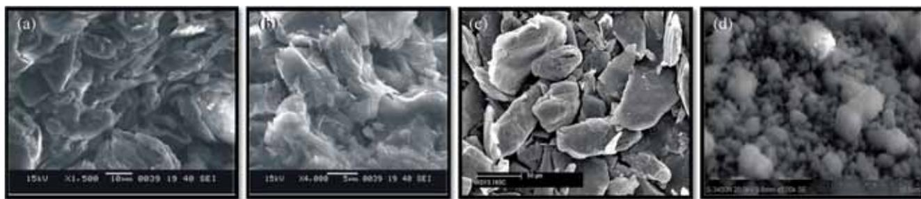
**Figure 3.** SEM images of GCB composite at (a) 1500 $\times$ , (b) 4000 $\times$ , (c) graphite at 250 $\times$  and (d) chitosan skeleton at 5000 $\times$ .
