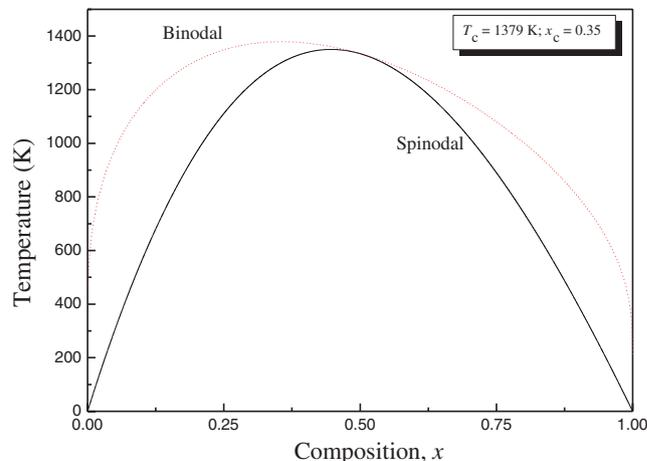
**Figure 7.**  $T$ – $x$  phase diagram of  $\text{SrTe}_{1-x}\text{O}_x$  alloys. Dashed line: binodal curve; solid line: spinodal curve.
