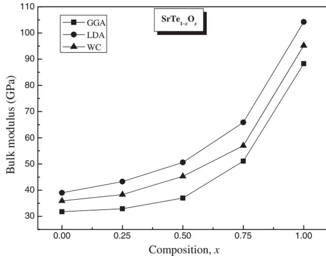
**Figure 2.** Concentration dependence of the bulk modulus calculated by different exchange-correlation energy approximations for SrTe<sub>1-x</sub>O<sub>x</sub> alloy.
