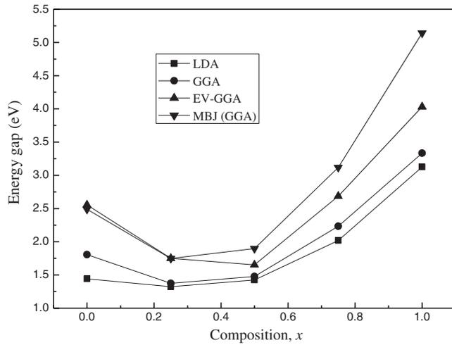
**Figure 3.** Band-gap energies of the SrTe<sub>1-x</sub>O<sub>x</sub> alloys as a function of O concentrations using LDA, GGA, EV-GGA and mBJ.
