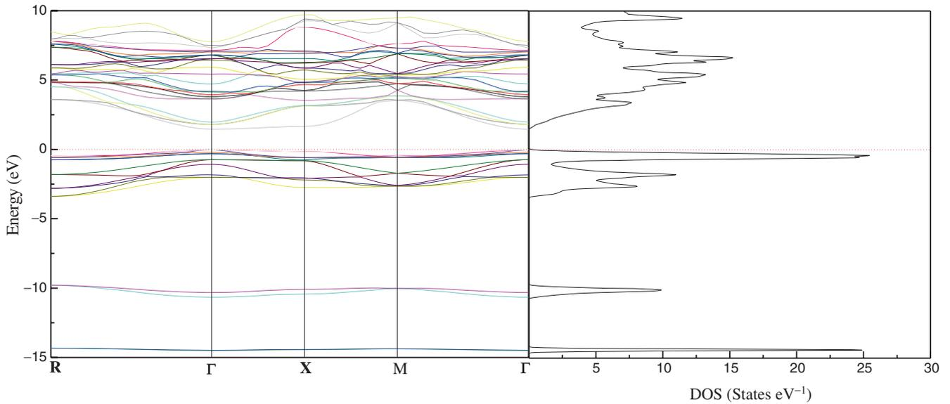
**Figure 5.** Band structure and projected density of states calculated for SrTe<sub>0.5</sub>O<sub>0.5</sub> alloy.
