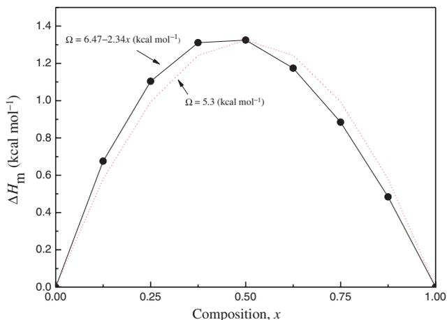
**Figure 6.** Enthalpy of mixing  $\Delta H_m$  as function of concentration for  $\text{SrTe}_{1-x}\text{O}_x$  ternary alloy. Solid curve:  $x$ -dependent interaction parameters  $\Omega$ , dotted curve:  $x$ -independent interaction parameters  $\Omega$ .
