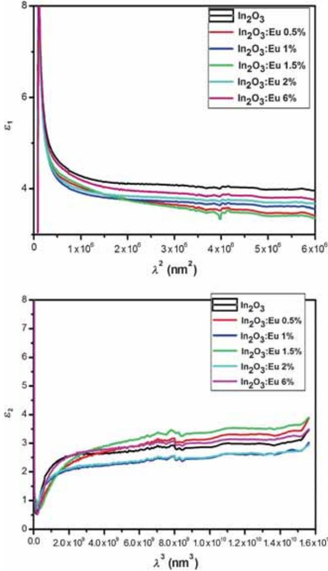
**Figure 8.** Variation of the real part with  $\lambda^2$  and imaginary part with  $\lambda^3$  of complex dielectric constant of Eu-doped In<sub>2</sub>O<sub>3</sub> thin films.
