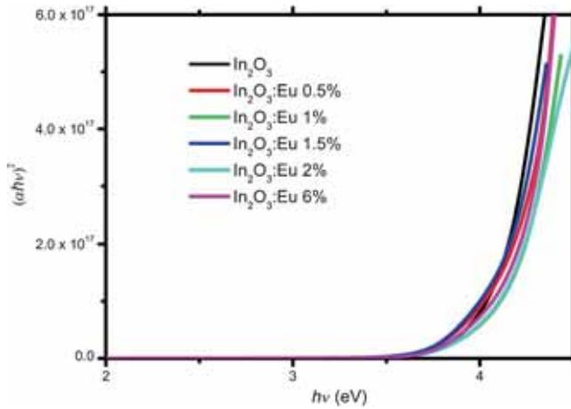
**Figure 5.**  $(\alpha h\nu)^2$  and  $\ln(\alpha)$  vs.  $h\nu$  for Eu-doped  $\text{In}_2\text{O}_3$  thin films.
