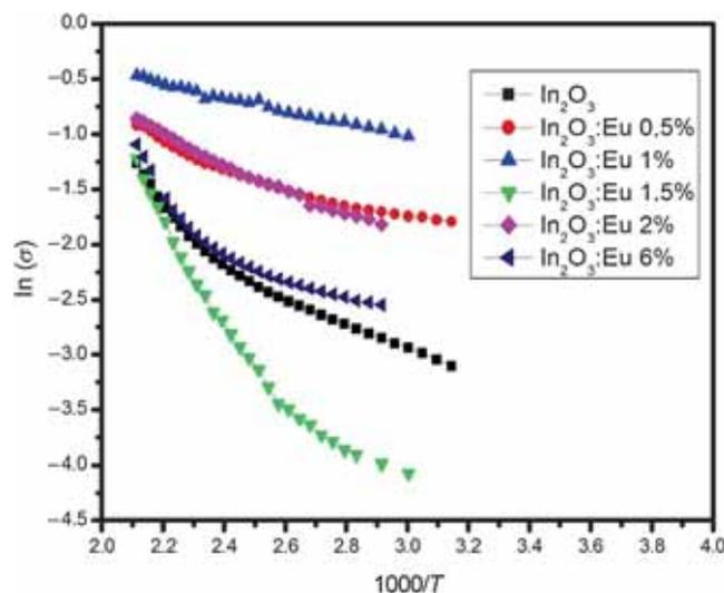
Figure 12. Electrical conductivity as a function of the temperature of Eu-doped  $\text{In}_2\text{O}_3$  thin films.
