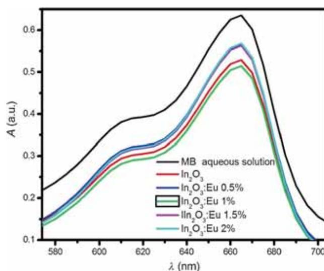
Figure 11. Absorbance spectra of both MB solution and Eu-doped  $\text{In}_2\text{O}_3$  thin films.
