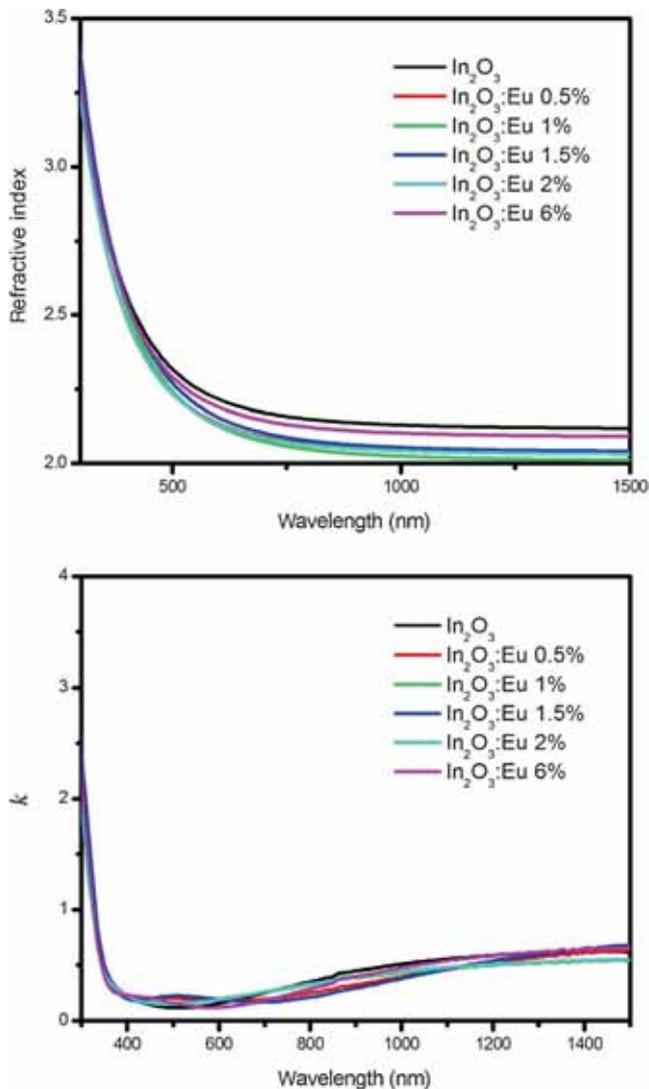
**Figure 7.** Refractive index and extinction coefficient of Eu-doped  $\text{In}_2\text{O}_3$  thin films.
