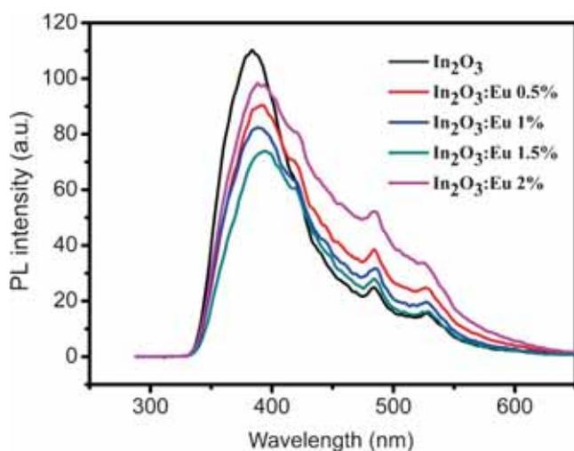
Figure 10. PL spectra of Eu-doped  $\text{In}_2\text{O}_3$  thin films.
