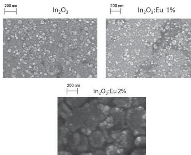
**Figure 3.** SEM observations of Eu-doped  $\text{In}_2\text{O}_3$  thin films.
