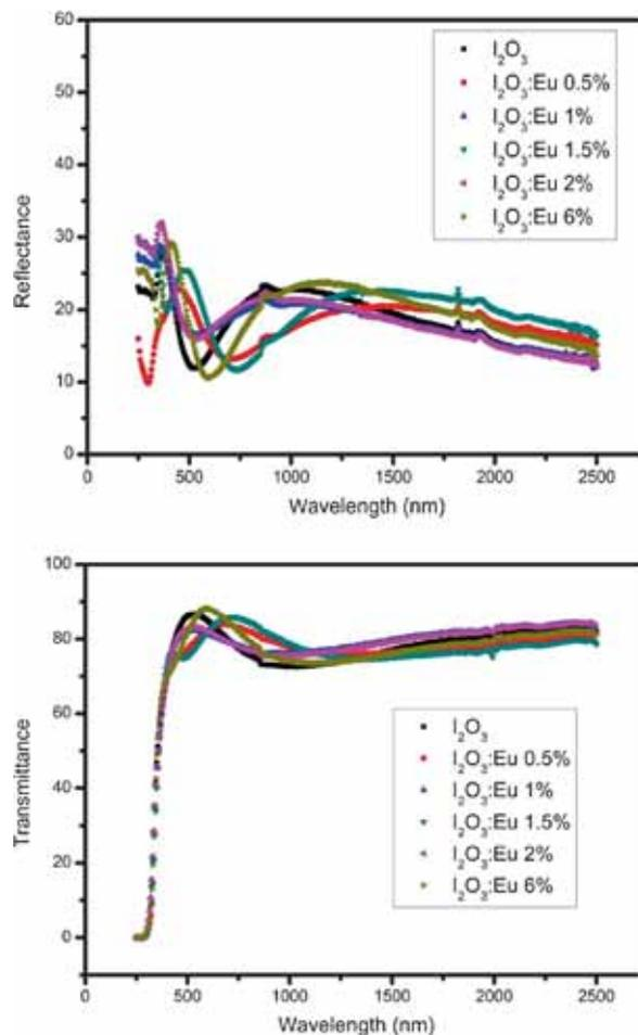
**Figure 4.** Reflection and transmission spectra of Eu-doped  $\text{In}_2\text{O}_3$  thin films.
