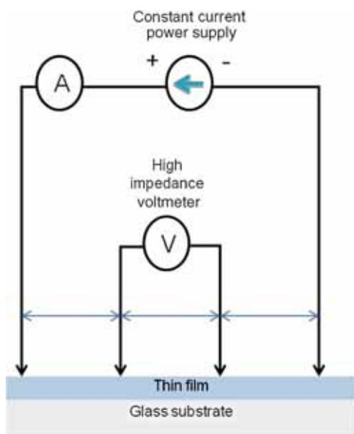
**Figure 1.** Configuration of Four probe method for the electrical measurements.
