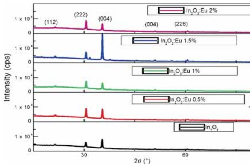
**Figure 2.** X-ray diffraction spectra of Eu-doped  $\text{In}_2\text{O}_3$  thin films for different ratios in the spray solution.
