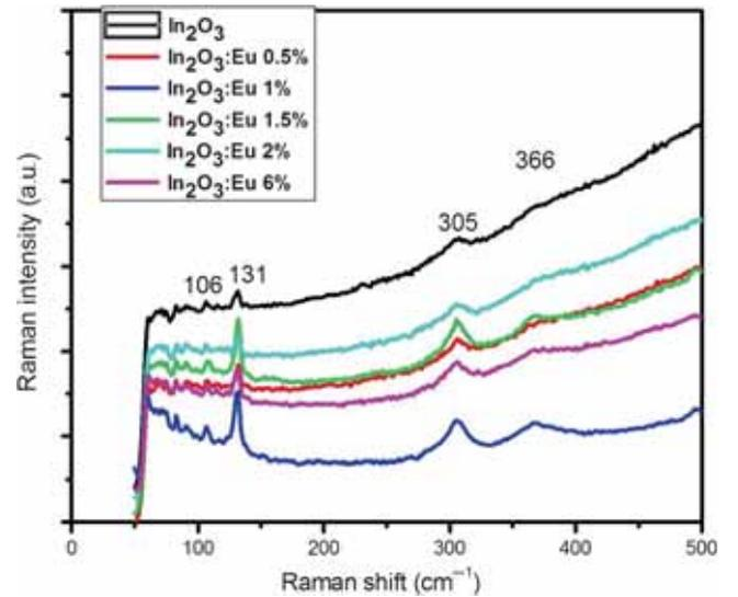
**Figure 9.** Raman spectra of Eu-doped In<sub>2</sub>O<sub>3</sub> thin films.
