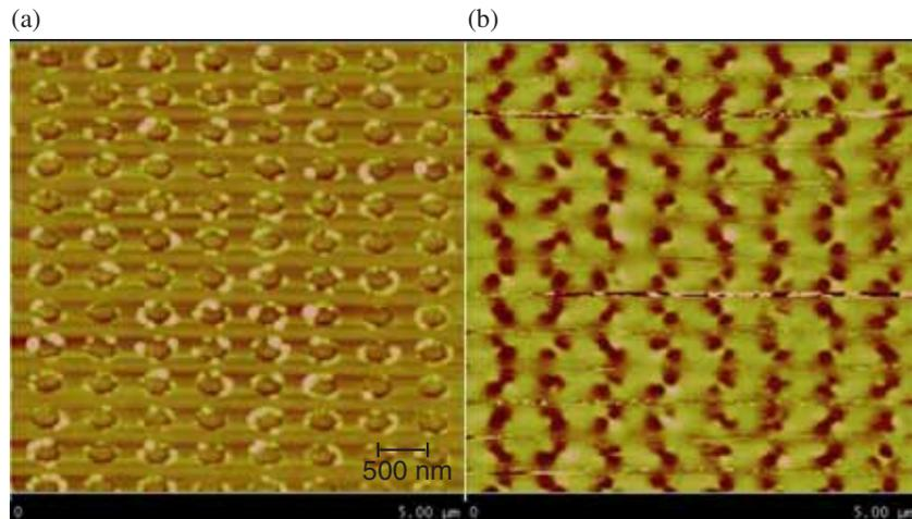
**Figure 4.** (a) AFM and (b) MFM pictures of  $\text{Co}_{50}\text{Fe}_{50}$  nanomagnets of thickness 60 nm.
