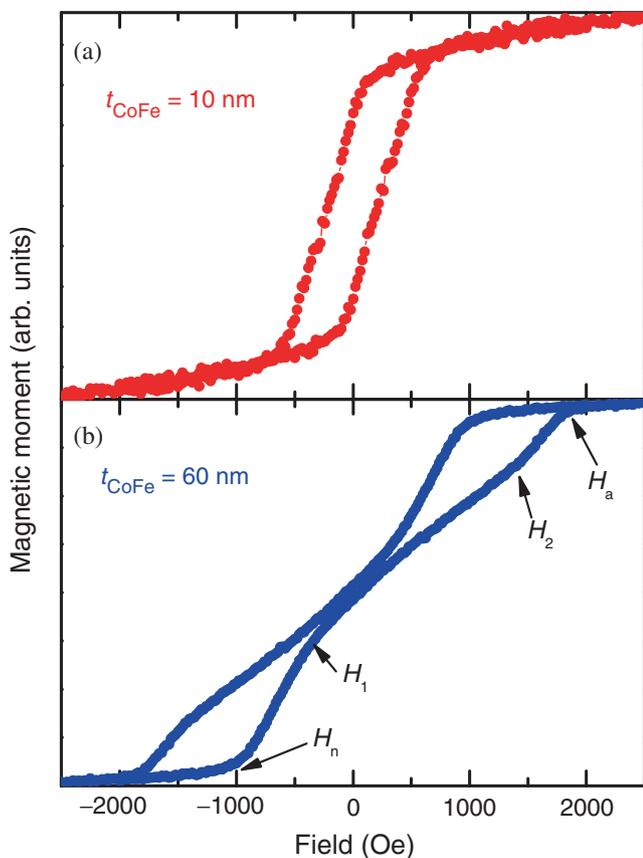
**Figure 1.** Variation of magnetization of  $\text{Co}_{50}\text{Fe}_{50}$  elliptical nanomagnets of thickness (a) 10 and (b) 60 nm.
