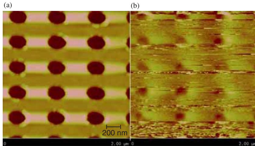
**Figure 3.** (a) AFM and (b) MFM pictures of  $\text{Co}_{50}\text{Fe}_{50}$  nanomagnets of thickness 10 nm.
