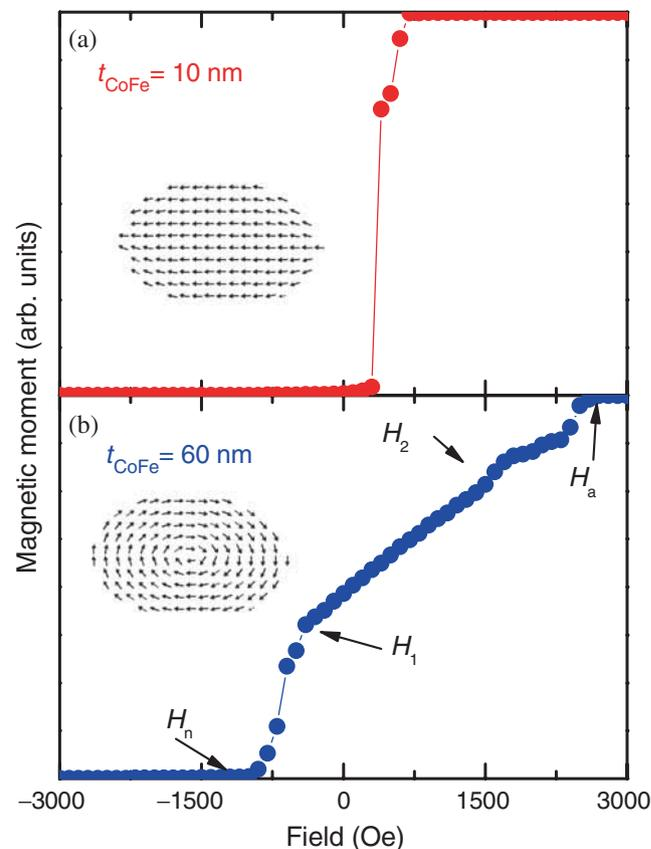
**Figure 2.** Simulation study of  $\text{Co}_{50}\text{Fe}_{50}$  elliptical nanomagnets of thickness (a) 10 and (b) 60 nm.
