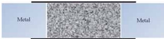
Figure 3. Rod-shaped composites are enclosed between two metal contacts to measure their bulk resistivity. Silver paste is used to make ohmic contacts to the composite.
