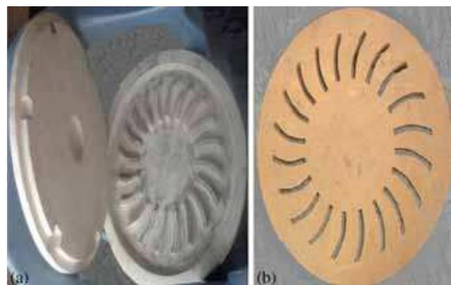
**Figure 1.** Disc brake rotor: (a) pattern and (b) core.
