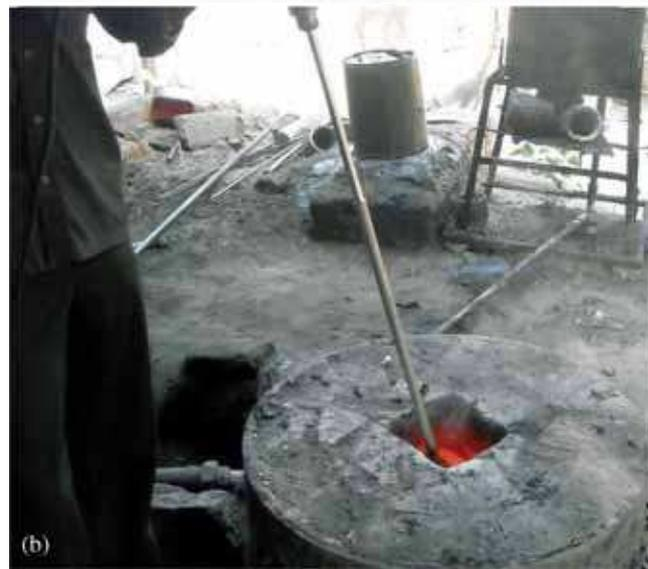
**Figure 3.** Cenosphere to the molten metal: (a) addition and (b) stirring by hand stirrer.
