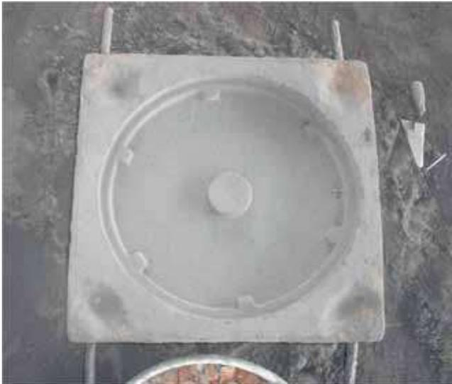
**Figure 2.** Preparation of sand mould for disc brake rotor.
