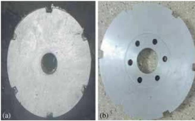
Figure 4. Casted disc brake rotor: (a) before machining and (b) after machining.
