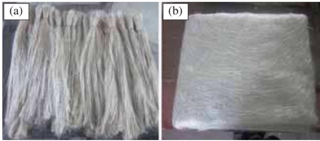
**Figure 2.** Fibres used for composite fabrication: (a) kenaf fibres and (b) glass fibre.
