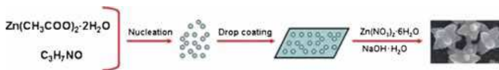
Figure 1. Schematic process for fabricating ZnO nanoflowers.
