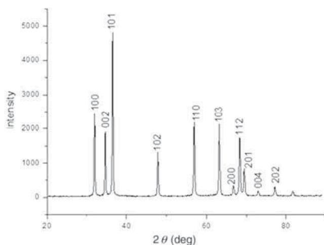
**Figure 3.** XRD spectrum of *L. aculeata*-mediated ZnO nanoparticles.
