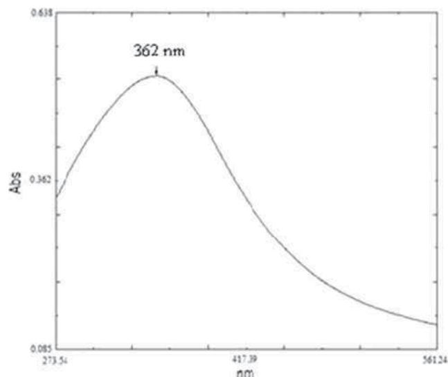
**Figure 1.** UV spectrum of *L. aculeata*-mediated ZnO nanoparticles.
