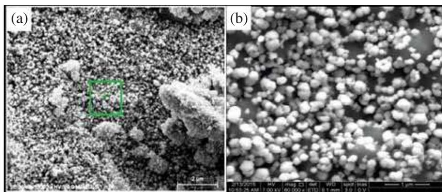
Figure 5. (a and b) FESEM images of *L. aculeata*-mediated ZnO nanoparticles.
