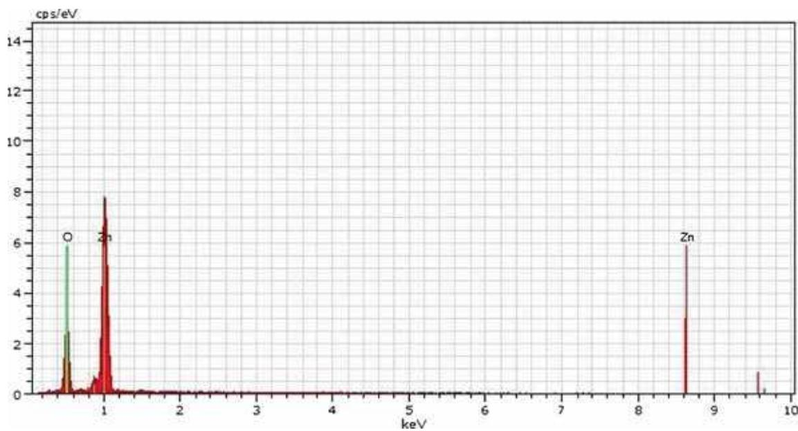
Figure 4. EDX spectrum of *L. aculeata*-mediated ZnO nanoparticles.
