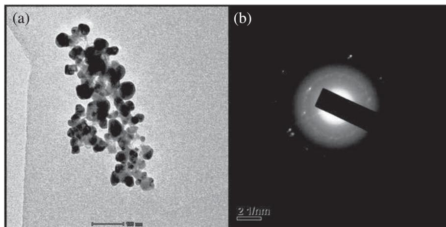
Figure 6. (a) HRTEM images of *L. aculeata*-mediated ZnO nanoparticles and (b) SAED pattern analysis of ZnO nanoparticles.
