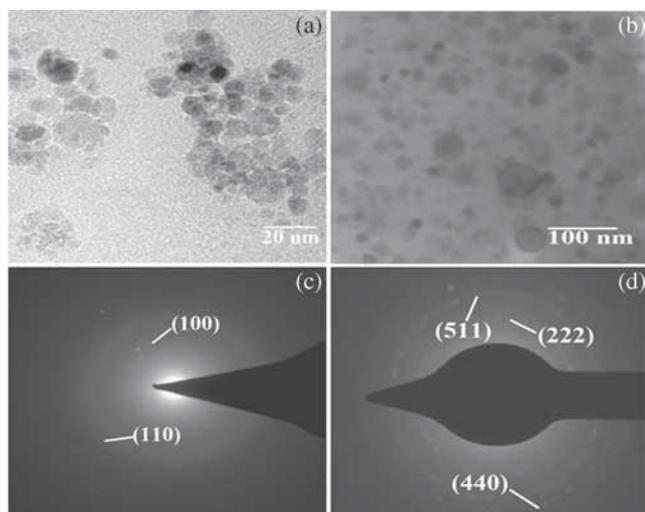
**Figure 5.** TEM images and SAED patterns of (a, c) CoS and (b, d) Co<sub>9</sub>S<sub>8</sub> nanocrystallites obtained from pyrolysis of Co(furtscz)<sub>2</sub> and CoCl<sub>2</sub>(furtsczH)<sub>2</sub> in furnace at 450 and 475°C, respectively.
