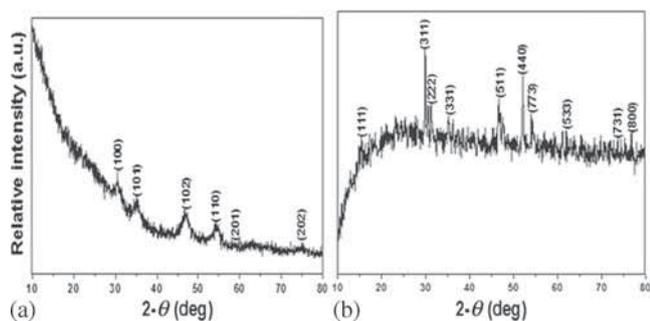
**Figure 1.** XRD patterns of (a) CoS and (b) Co<sub>9</sub>S<sub>8</sub> nanocrystallites obtained from pyrolysis of Co(furtscz)<sub>2</sub> and CoCl<sub>2</sub>(furtschH)<sub>2</sub> in furnace at 450 and 475°C, respectively.
