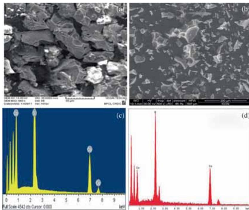
**Figure 3.** SEM images and EDAX spectra of (a, c)  $\text{CoS}$  and (b, d)  $\text{Co}_9\text{S}_8$  nanocrystallites obtained from pyrolysis of  $\text{Co}(\text{furtscz})_2$  and  $\text{CoCl}_2(\text{furtsczH})_2$  in furnace at 450 and 475°C, respectively.
