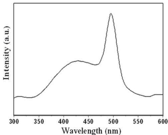
**Figure 8.** PL spectrum of CoS nanocrystallites obtained from solvothermal decomposition of Co(cinnamtsz)<sub>2</sub> in ethylene glycol.
