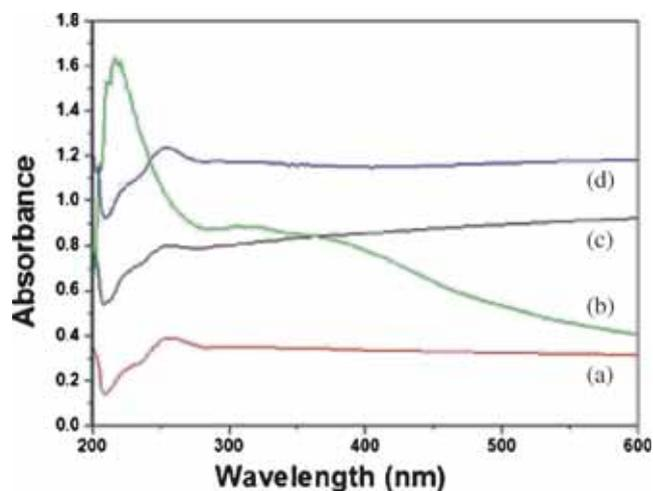
**Figure 7.** Absorption spectra of (a) Co<sub>9</sub>S<sub>8</sub> nanocrystallites obtained from pyrolysis of CoCl<sub>2</sub>(furtsczH)<sub>2</sub>, (b) CoS nanocrystallites obtained from pyrolysis of Co(cinnamtsz)<sub>2</sub>, (c) CoS nanocrystallites obtained from solvothermal decomposition of CoCl<sub>2</sub>(furtsczH)<sub>2</sub> and (d) CoS nanocrystallites obtained from solvothermal decomposition of CoCl<sub>2</sub>(4-facphtszH)<sub>2</sub>.
