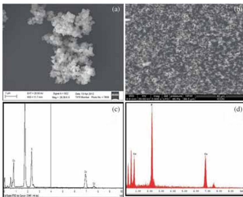
**Figure 4.** SEM images and EDAX spectra of (a, c)  $\text{Co}_9\text{S}_8$  and (b, d)  $\text{CoS}$  nanocrystallites obtained from solvothermal decomposition of  $\text{Co}(\text{furtscz})_2$  and  $\text{CoCl}_2(\text{furtsczH})_2$  in ethylene glycol, respectively.
