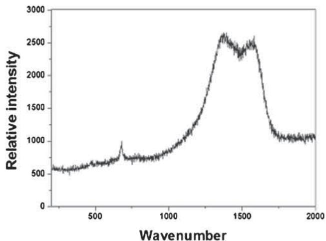
**Figure 10.** Raman spectrum of  $\text{CoS}$  nanocrystallites obtained from solvothermal decomposition of  $\text{CoCl}_2(\text{furtsczH})_2$  in ethylene glycol.
