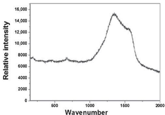
**Figure 9.** Raman spectrum of  $\text{CoS}$  nanocrystallites obtained from pyrolysis of  $\text{Co}(\text{furtscz})_2$  at  $450^\circ\text{C}$ .
