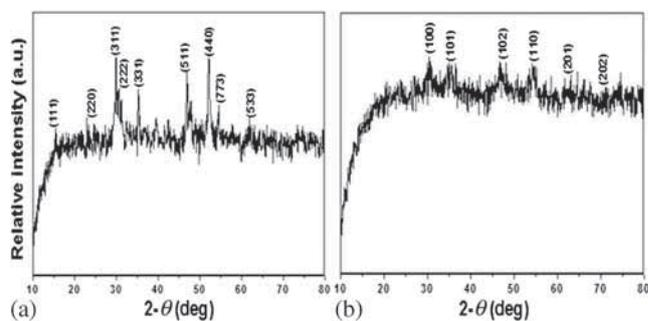
**Figure 2.** XRD patterns of (a) Co<sub>9</sub>S<sub>8</sub> and (b) CoS nanocrystallites obtained from solvothermal decomposition of Co(furtscz)<sub>2</sub> and CoCl<sub>2</sub>(furtschH)<sub>2</sub> in ethylene glycol, respectively.
