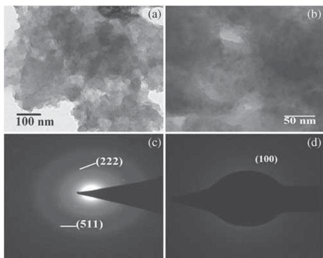
**Figure 6.** TEM images and SAED patterns of (a, c) CoS and (b, d) Co<sub>9</sub>S<sub>8</sub> nanocrystallites obtained from solvothermal decomposition of Co(furtscz)<sub>2</sub> and CoCl<sub>2</sub>(furtsczH)<sub>2</sub> in ethylene glycol, respectively.
