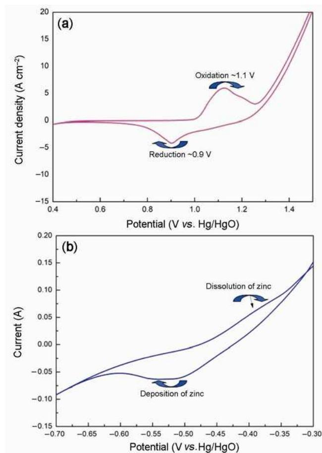
**Figure 2.** Typical CVs of the (a) zinc metal and (b) NiCo $_2$ O $_4$  at a scan rate of  $2 \text{ mV s}^{-1}$ .
