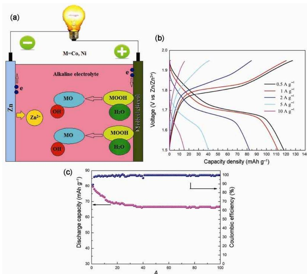
**Figure 3.** (a) Schematic representation of the electrochemical reaction process of the Zn–NiCo<sub>2</sub>O<sub>4</sub> prototype cell; (b) charge and discharge curves of the NiCo<sub>2</sub>O<sub>4</sub> at different rates using Zn metal as the counter electrode and (c) cycling performance of the Zn//NiCo<sub>2</sub>O<sub>4</sub> prototype cell at 2 A g<sup>-1</sup>.
