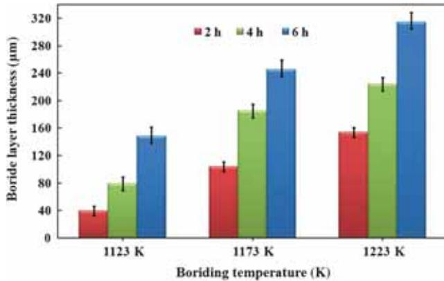
**Figure 2.** Thickness values of boride layers as a function of boriding parameters (time and temperature).
