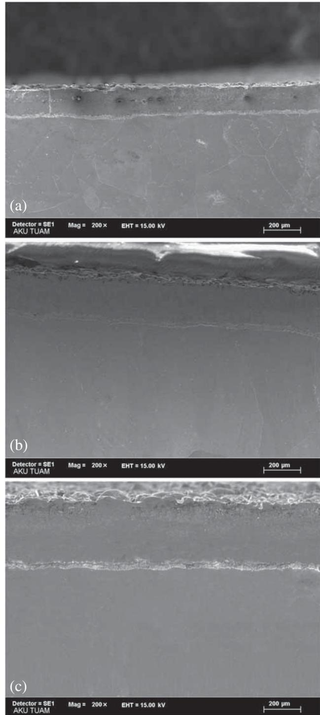
**Figure 1.** Cross-sections of the borided Nickel 201 alloy (a) 1123 K–6 h, (b) 1173 K–6 h and (c) 1223 K–6 h.
