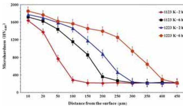
**Figure 4.** Microhardness profiles obtained at the surface of borided Nickel 201 alloy.
