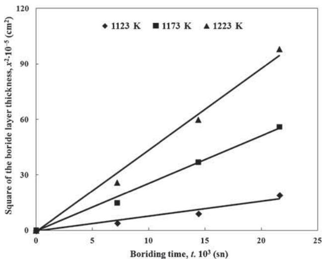
**Figure 5.** Time dependence of the square of boride layer thickness at increasing temperatures.
