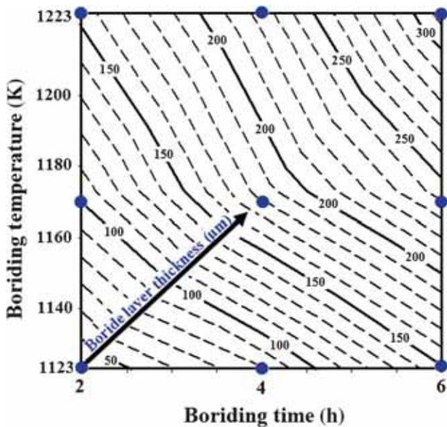
**Figure 7.** Contour diagram describing the evolution of boride layer thickness as a function of boriding parameters (time and temperature).
