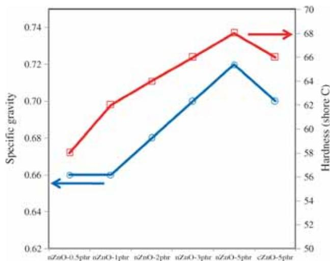
**Figure 6.** Specific gravity and hardness of the CR foam with various synthesized ZnO nanoparticles' content compared with conventional ZnO.
