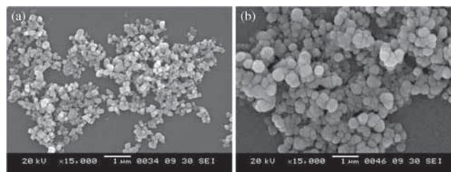
**Figure 3.** SEM images of ZnO particles (a) the synthesized ZnO nanoparticles and (b) the conventional ZnO.
