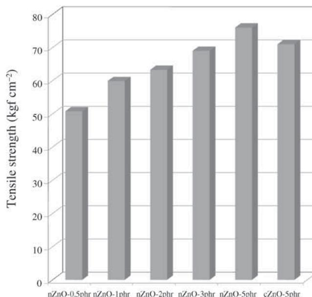
**Figure 7.** Tensile strength of the CR foam with various synthesized ZnO nanoparticles' content compared with conventional ZnO.
