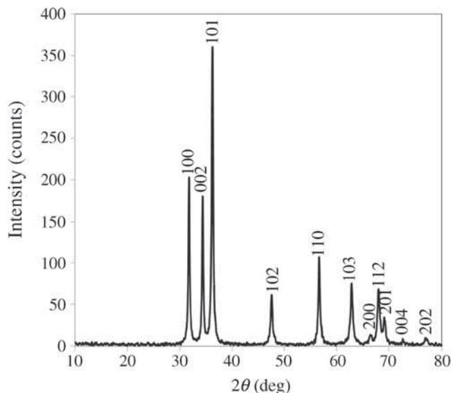
**Figure 1.** XRD pattern of the synthesized ZnO nanoparticles.
