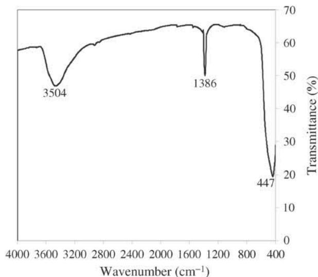
**Figure 2.** FTIR spectra of the synthesized ZnO nanoparticles.
