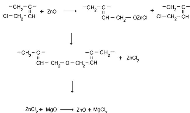
**Figure 5.** Mechanism of crosslinking by metal oxide.
