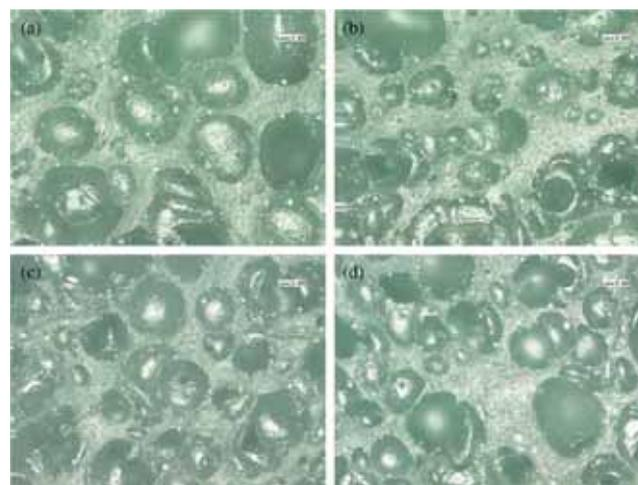
**Figure 8.** Morphology of the CR foam using (a) the synthesized ZnO nanoparticles at 1 phr, (b) the synthesized ZnO nanoparticles at 3 phr, (c) the synthesized ZnO nanoparticles at 5 phr and (d) the conventional ZnO at 5 phr.
