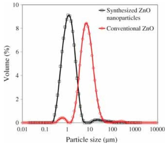
**Figure 4.** Particle size distribution of the synthesized ZnO nanoparticles and the conventional ZnO.
