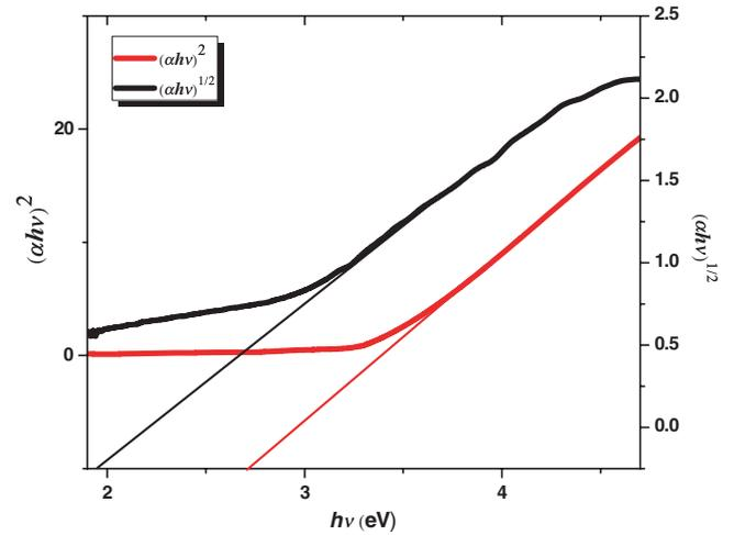
**Figure 5.** Direct and indirect band gap of sample GG7.
