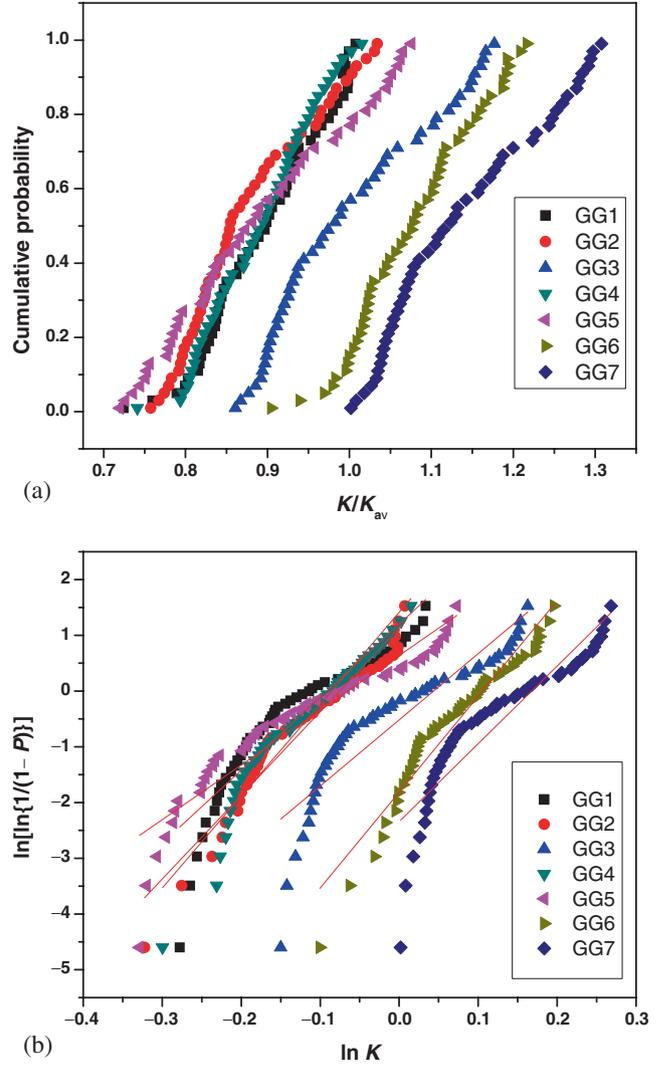
**Figure 6.** (a) Cumulative probability of failure for all the samples and (b) Weibull plots for fracture toughness of all the samples.
