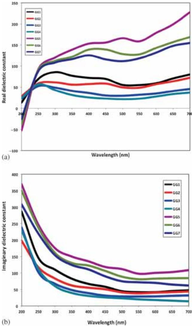
**Figure 4.** (a) Real dielectric constant of all the glass composites and (b) imaginary dielectric constant of all the glass composites.
