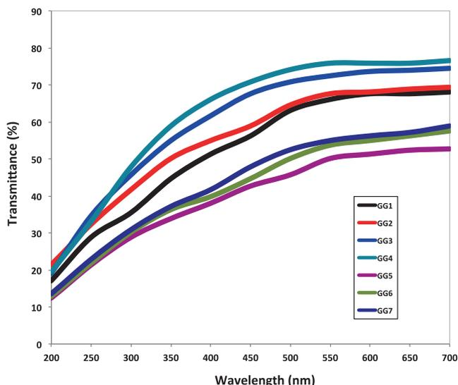
**Figure 2.** Transmission spectra of all the glass composites.
