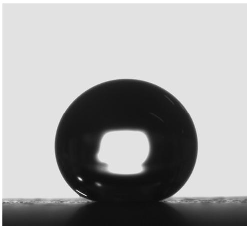
**Figure 3.** Measured CA of 160° on superhydrophobic sample.
