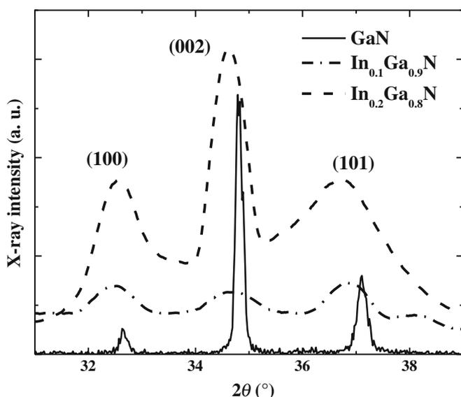
**Figure 2.** X-ray diffractogram patterns of  $\text{In}_x\text{Ga}_{1-x}\text{N}$  samples: (A) GaN, (B)  $\text{In}_{0.1}\text{Ga}_{0.9}\text{N}$  and (C)  $\text{In}_{0.2}\text{Ga}_{0.8}\text{N}$ .
