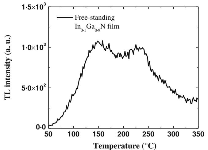
**Figure 5.** TL signal of free-standing  $\text{In}_{0.1}\text{Ga}_{0.9}\text{N}$  layer exposed to 360 Gy of beta radiation.
