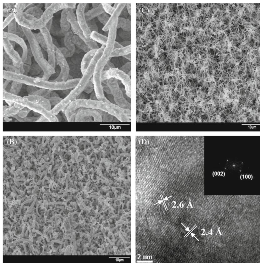
**Figure 3.** SEM and TEM images of the  $\text{In}_x\text{Ga}_{1-x}\text{N}$  samples grown by chemical vapour deposition: (A) GaN, (B)  $\text{In}_{0.1}\text{Ga}_{0.9}\text{N}$ , (C)  $\text{In}_{0.2}\text{Ga}_{0.8}\text{N}$  and (D) high resolution TEM image of the  $\text{In}_{0.1}\text{Ga}_{0.9}\text{N}$ .
