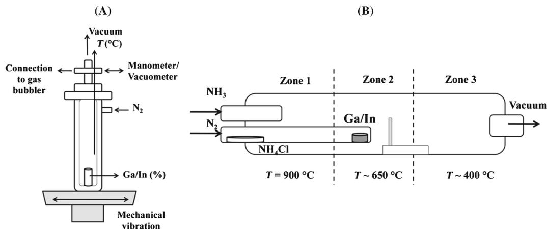
**Figure 1.** Schematic diagrams of the two stages of indium–gallium nitride growth. (A) Small reactor used for In–Ga alloy formation and (B) horizontal CVD reactor used for the  $\text{In}_x\text{Ga}_{1-x}\text{N}$  growth.
