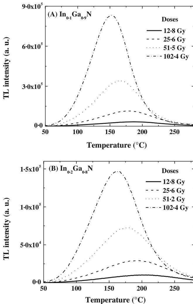
**Figure 4.** Thermoluminescence glow curve of (A)  $\text{In}_{0.1}\text{Ga}_{0.9}\text{N}$  and (B)  $\text{In}_{0.2}\text{Ga}_{0.8}\text{N}$  samples exposed to beta radiation at different doses.
