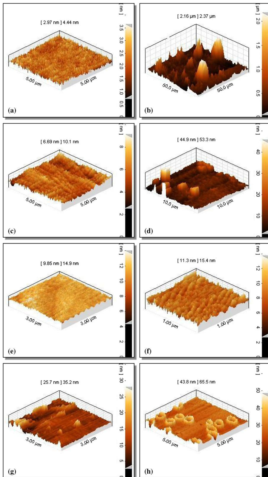
**Figure 6.** AFM images of B1 (200 °C), B2 (300 °C), B3 (350 °C) and B4 (400 °C) samples before and after spray-water test: (a) B1 before test, (b) B1 after test (c) B2 before test, (d) B2 after test, (e) B3 before test, (f) B3 after test, (g) B4 before test and (h) B4 after test.
