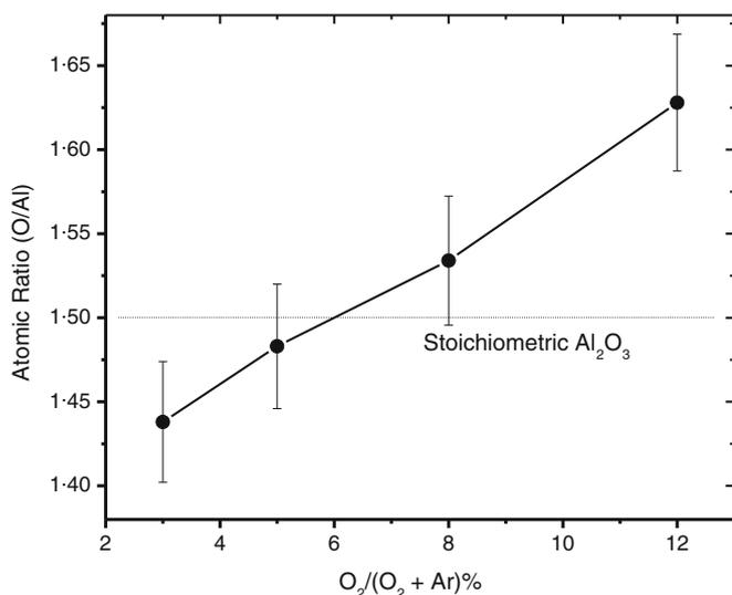
**Figure 3.** Compositional change of alumina thin films as a function of oxygen flow ratio.
