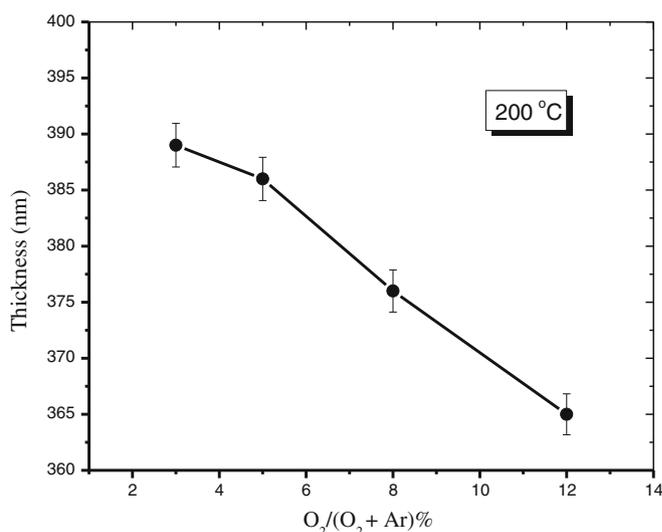
**Figure 1.** Variation of films thickness as a function of oxygen volume percentage at 200 °C.
