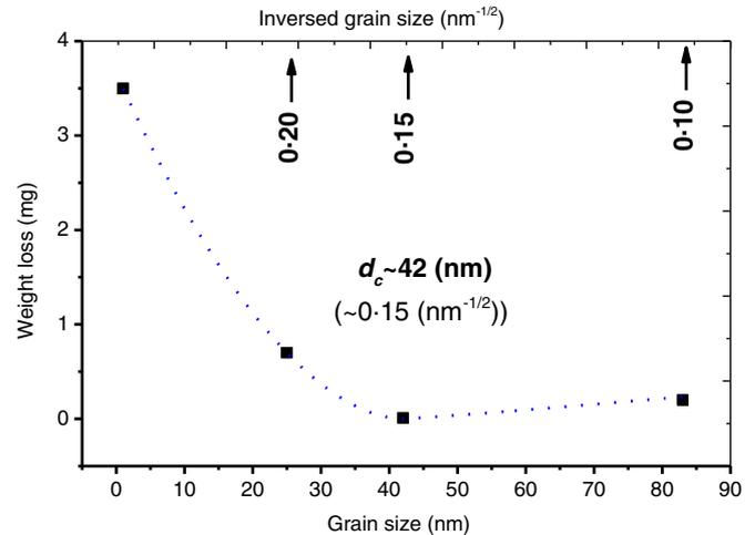
**Figure 8.** Weight loss of  $\text{Al}_2\text{O}_3$  coatings as a function of average grain size.
