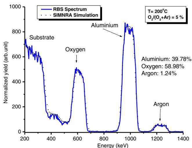
**Figure 2.** Typical RBS spectrum with corresponding SIMNRA simulated curve.
