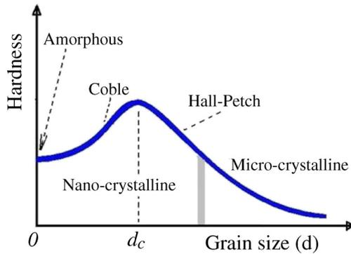
**Figure 7.** Schematic illustration of hardness vs average grain size.
