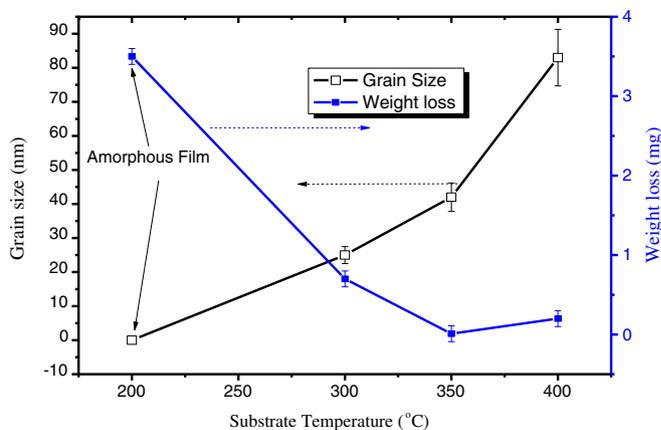
**Figure 5.** Grain size and weight loss of the films as a function of substrate temperature.
