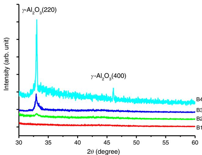
**Figure 4.** X-ray diffraction patterns of alumina films deposited at different substrate temperatures.
