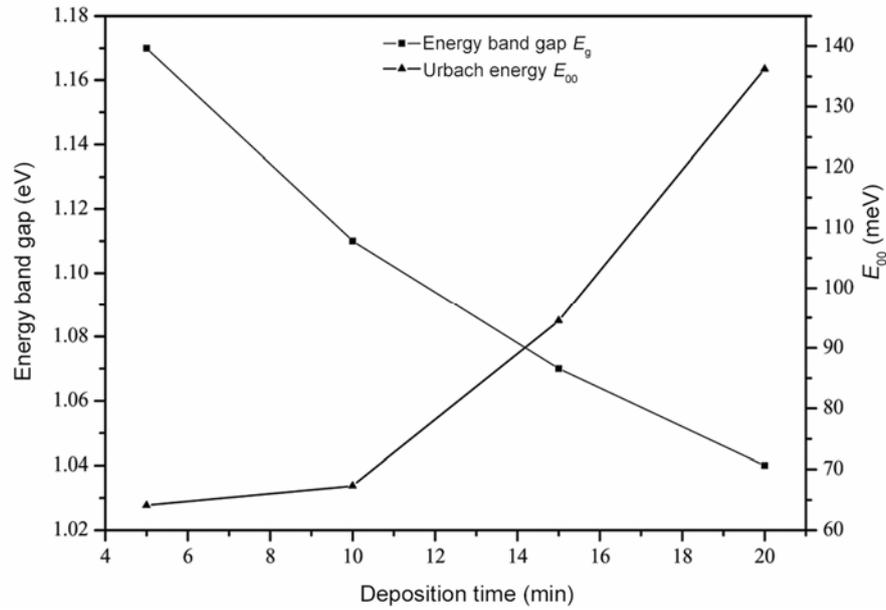
**Figure 8.** Variation of energy band gap,  $E_g$ , and Urbach energy,  $E_{00}$ , vs deposition time.
