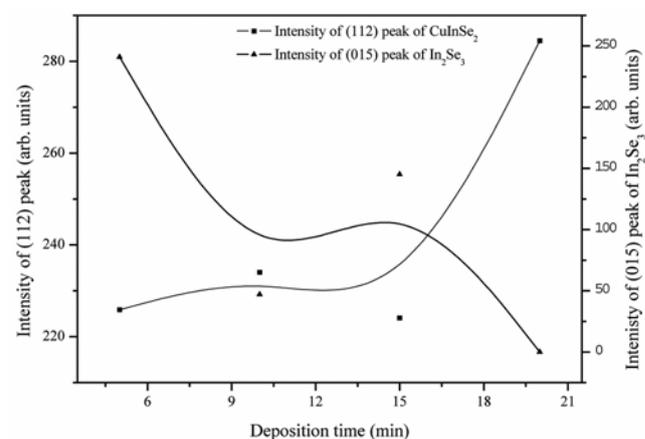
**Figure 4.** Representation of the intensity of the main CuInSe<sub>2</sub> and In<sub>2</sub>Se<sub>3</sub> diffraction peak as a function of the deposition time.
