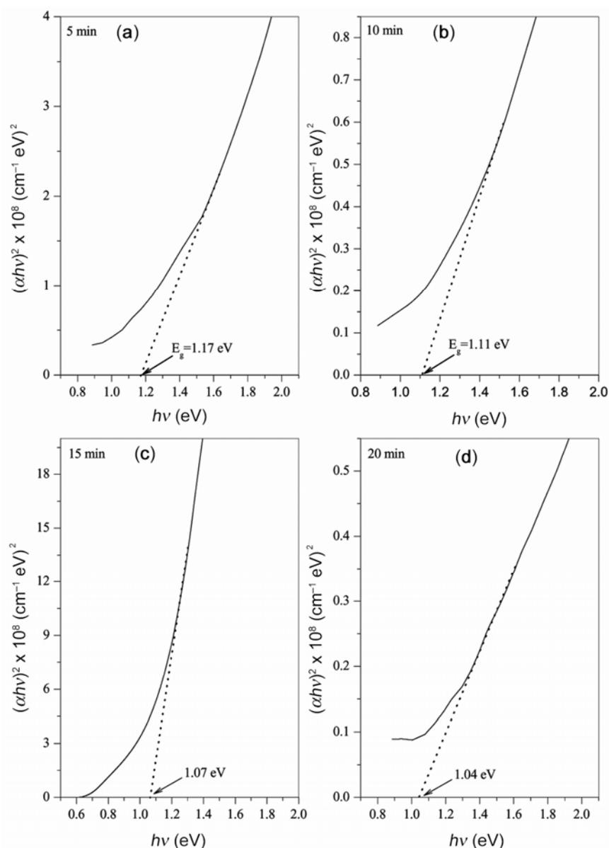
**Figure 7.** The square of the measured absorption coefficient  $(\alpha h\nu)^2$  vs the incident photon energy ( $h\nu$ ) for  $\text{CuInSe}_2$  film deposited at different times: (a) 5, (b) 10, (c) 15 and (d) 20 min.
