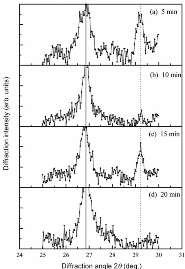
**Figure 3.** XRD scans reflecting only a section of the scan 25–30° for the films related to different deposition times.
