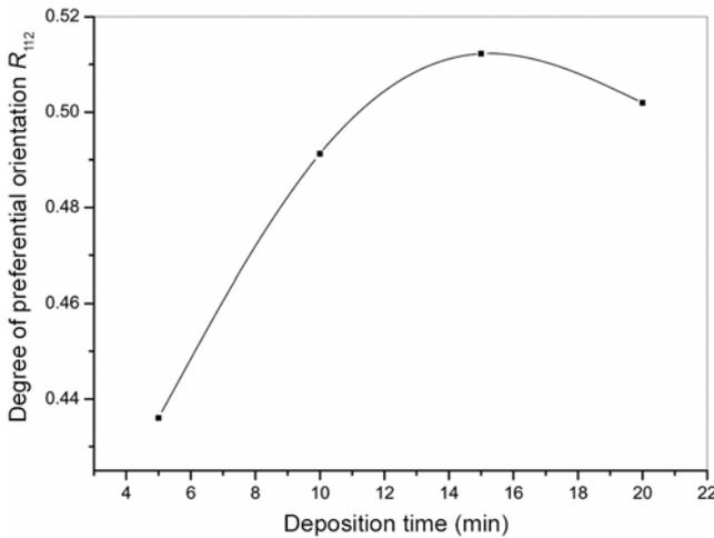
**Figure 5.** The variations of  $R_{(112)}$  of elaborated thin films as a function of deposition time.
