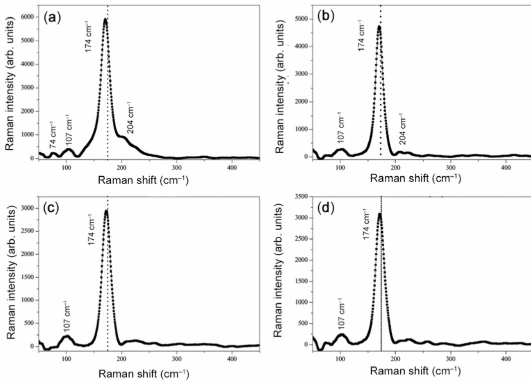
**Figure 9.** Raman spectra of CuInSe<sub>2</sub> thin films deposited at different times: (a) 5, (b) 10, (c) 15 and (d) 20 min.
