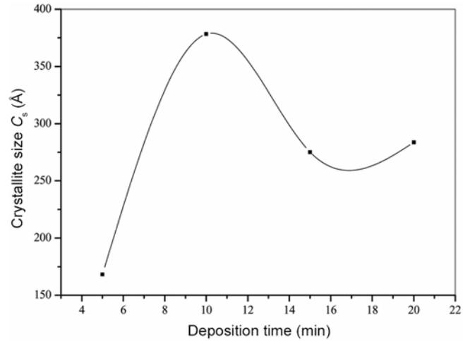
**Figure 6.** Variation of crystallite size with deposition time.
