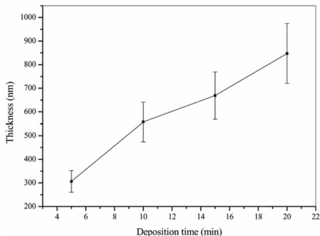
Figure 1. Variation of film thickness vs deposition time.
