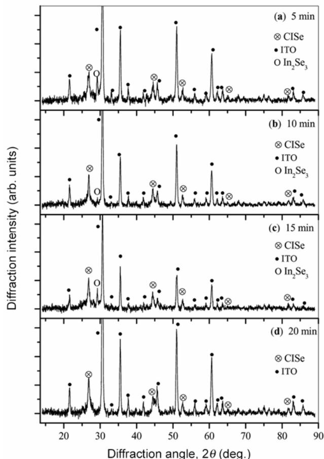
Figure 2. XRD patterns of CuInSe<sub>2</sub> deposited on ITO-coated glass substrate after annealing under vacuum at 300 °C during 30 min related to different deposition times: (a) 5, (b) 10, (c) 15 and (d) 20 min. The diffraction peaks identified from the CuInSe<sub>2</sub>, ITO and In<sub>2</sub>Se<sub>3</sub> are, respectively, marked by ⊕, • and ○.
