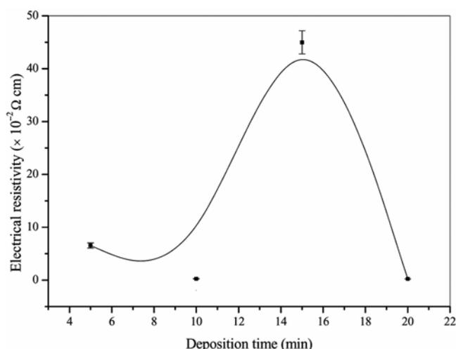
**Figure 10.** Variation of the room temperature electrical resistivity vs deposition time.
