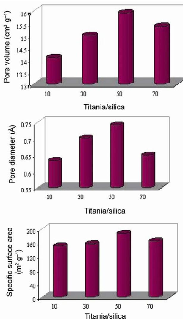
**Figure 2.** N<sub>2</sub> adsorption-desorption measurements of samples at different weight ratios of titania to silica.
