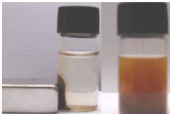
**Figure 8.** Recovery of catalyst (left) from medium (right) by a magnet.
