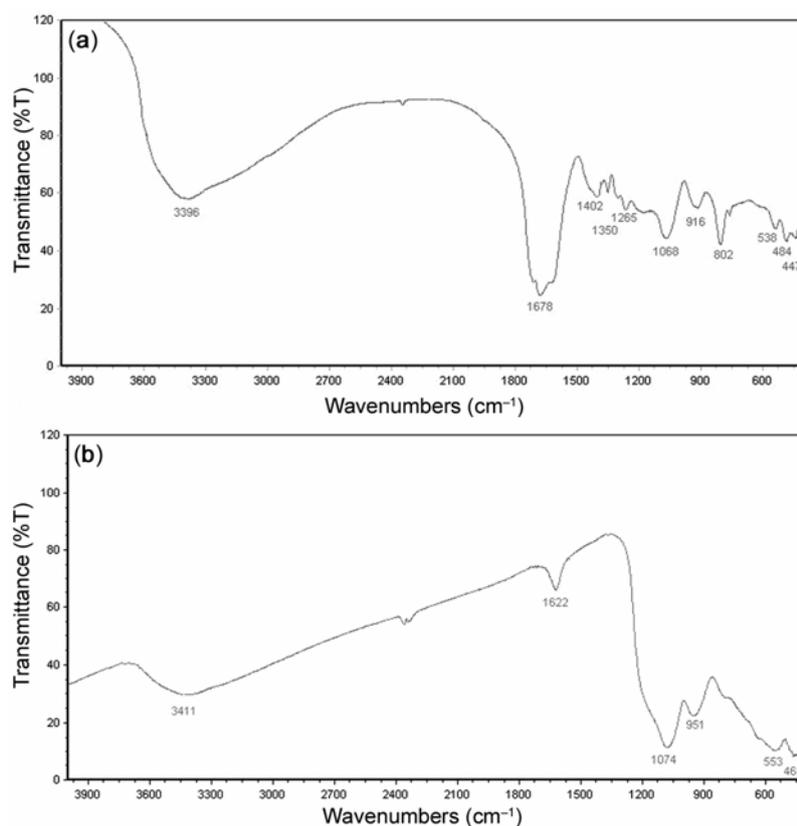
**Figure 7.** FT-IR spectra of the Fe-V/TiO<sub>2</sub>-SiO<sub>2</sub> promoted with zinc: (a) precursor and (b) calcined sample.
