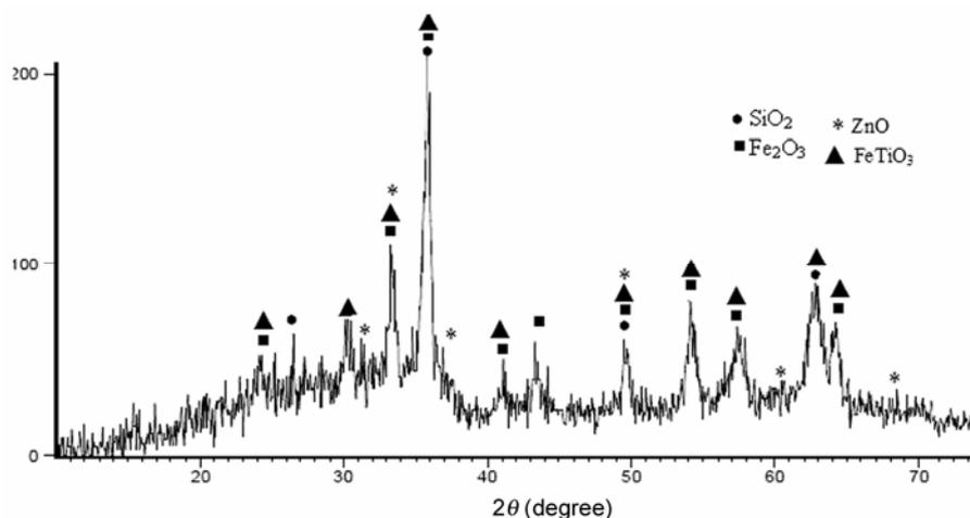
**Figure 5.** XRD pattern of Fe–V/TiO<sub>2</sub>–SiO<sub>2</sub> sample modified by zinc.
