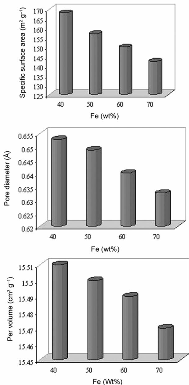
**Figure 3.** Specific surface area, pore diameter and pore volume of samples at different weight ratios of Fe.
