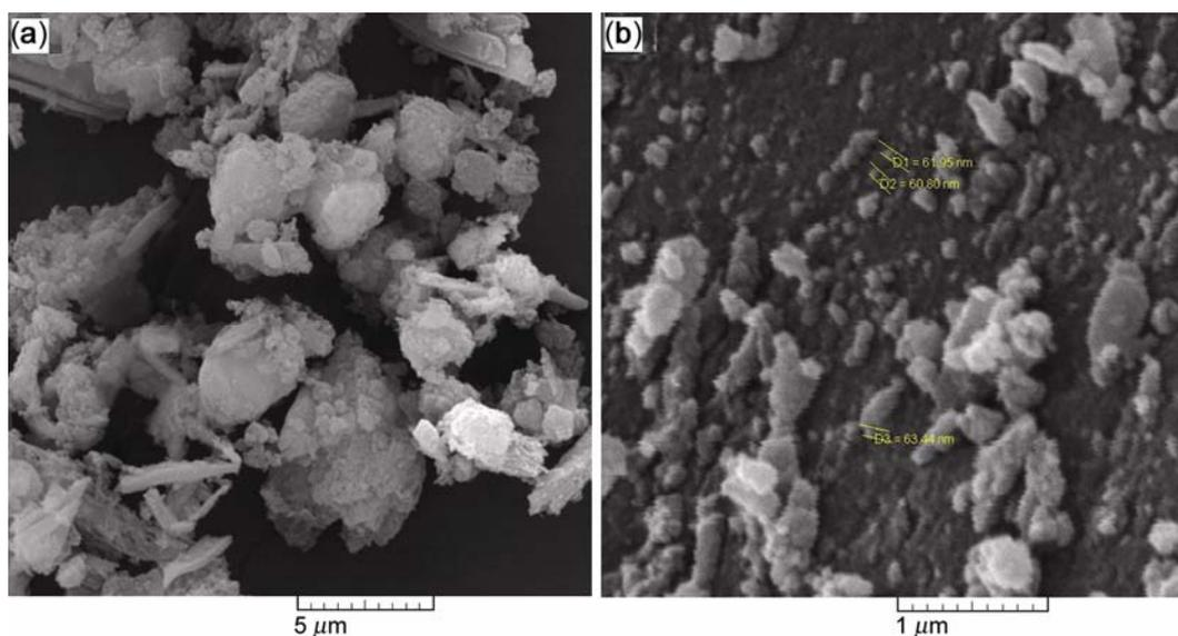
**Figure 6.** SEM images of Fe-V/TiO<sub>2</sub>-SiO<sub>2</sub> sample modified by Zn: (a) precursor and (b) calcined sample.
