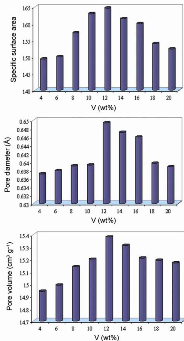
**Figure 4.** Specific surface area, pore diameter and pore volume of samples at different weight ratios of vanadium.
