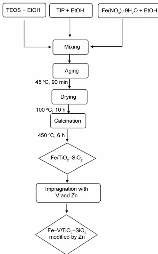
**Figure 1.** Diagram of the chemical processes for the preparation of Fe-V/TiO<sub>2</sub>-SiO<sub>2</sub> samples promoted with zinc.
