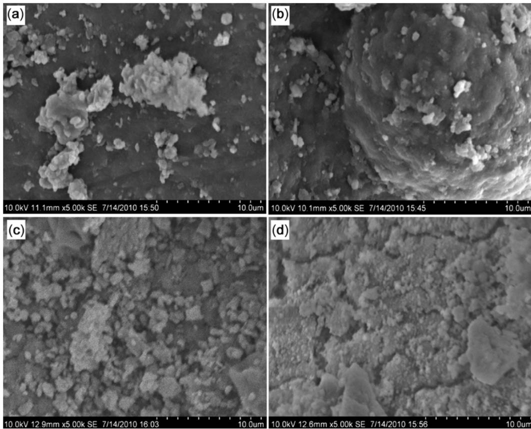
**Figure 4.** SEM micrograph (magnification 500 $\times$ ) of (a) BC, (b) BCTA, (c) BC after treatment in SBF for 21 days and (d) BCTA after treatment in SBF for 21 days.
