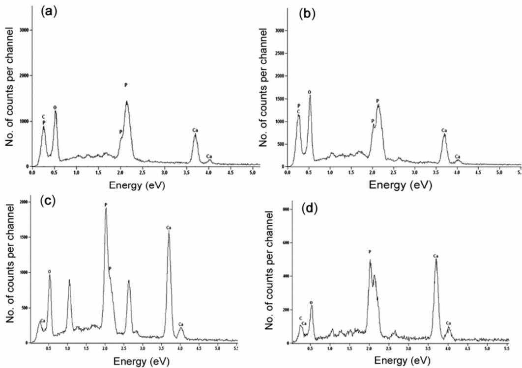
**Figure 5.** EDX data of (a) BC, (b) BCTA, (c) BC after treatment in SBF for 21 days and (d) BCTA after treatment in SBF for 21 days.
