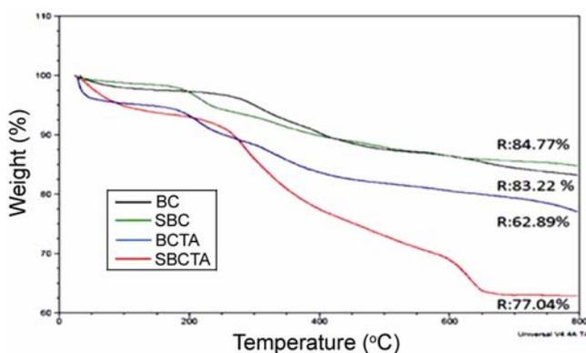
**Figure 3.** Thermogravimetric analysis of BC, BCTA, SBC and SBCTA.
