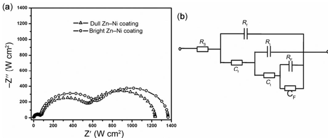
**Figure 10.** Nyquist plots of (a) dull and bright ZnNi alloy deposits at  $4 \text{ A dm}^{-2}$  obtained in absence and presence of EV at  $4 \text{ A dm}^{-2}$  and (b) its equivalent electrical circuit.
