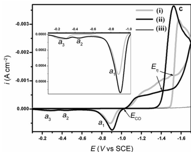
**Figure 2.** Cyclic voltammograms obtained from bath 0.34 M  $\text{ZnSO}_4 \cdot 7\text{H}_2\text{O}$ , 0.076 M  $\text{NiSO}_4 \cdot 7\text{H}_2\text{O}$ , 0.065 M  $\text{H}_3\text{BO}_3$  and 2 M  $\text{Na}_2\text{SO}_4$  in (i) absence and (ii) presence of 1.5 mM EV and (iii) in supporting electrolyte 2 M  $\text{Na}_2\text{SO}_4$ , 0.065 M  $\text{H}_3\text{BO}_3$  and 1.5 mM EV.
