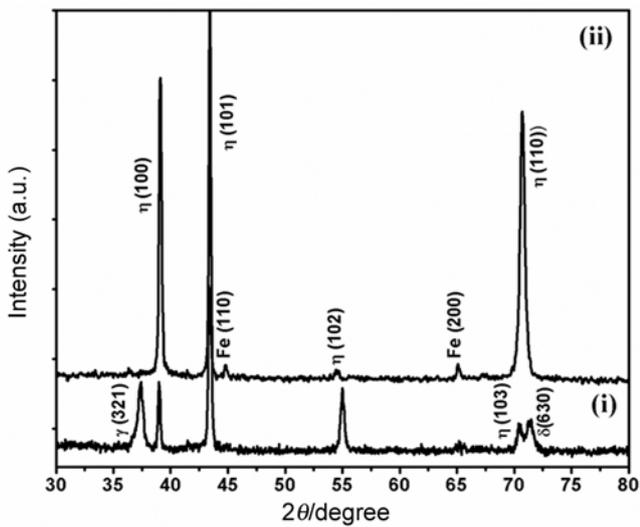
**Figure 5.** X-ray diffraction patterns of (i) dull and (ii) bright ZnNi electrodeposit obtained in absence and presence of EV at  $4 \text{ A dm}^{-2}$ .
