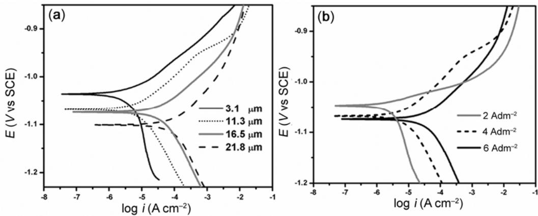
**Figure 9.** The potentiodynamic polarization curves for bright ZnNi coating obtained in presence of EV at different (a) thicknesses and (b) current densities.
