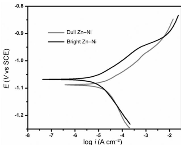
**Figure 8.** Potentiodynamic polarization curves for dull and bright ZnNi deposit obtained in absence and presence of EV at 4 A dm<sup>-2</sup>.
