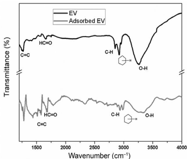
**Figure 3.** FT-IR spectra of EV powder sample and adsorbed EV on steel.
