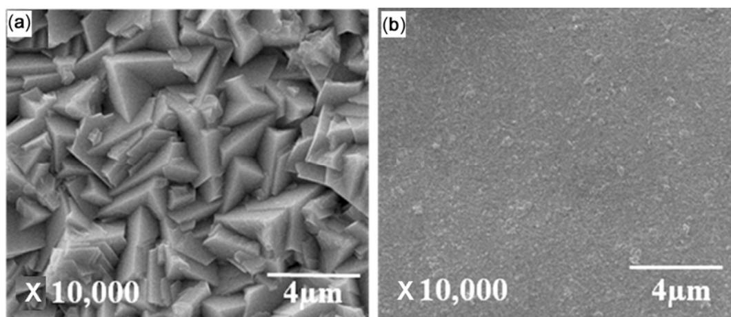
**Figure 4.** SEM images of (a) dull and (b) bright ZnNi electrodeposit obtained in absence and presence of EV at  $4 \text{ A dm}^{-2}$ .
