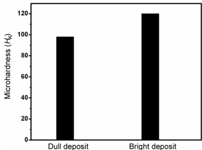
**Figure 7.** Microhardness of dull and bright ZnNi deposit obtained in absence and presence of EV at  $4 \text{ A dm}^{-2}$ .
