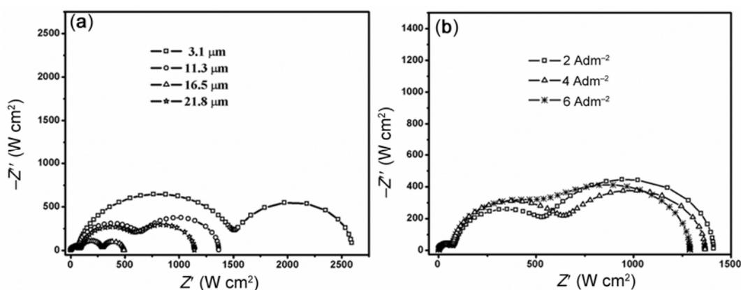
**Figure 11.** Nyquist plots of bright ZnNi alloy coating obtained in presence of EV at different (a) thicknesses and (b) current densities.
