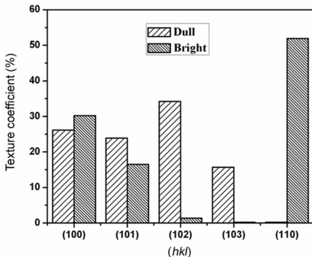
**Figure 6.** Percent  $T_c$  values as a function of crystallographic plane for dull and bright ZnNi deposit obtained in absence and presence of EV at  $4 \text{ A dm}^{-2}$ .
