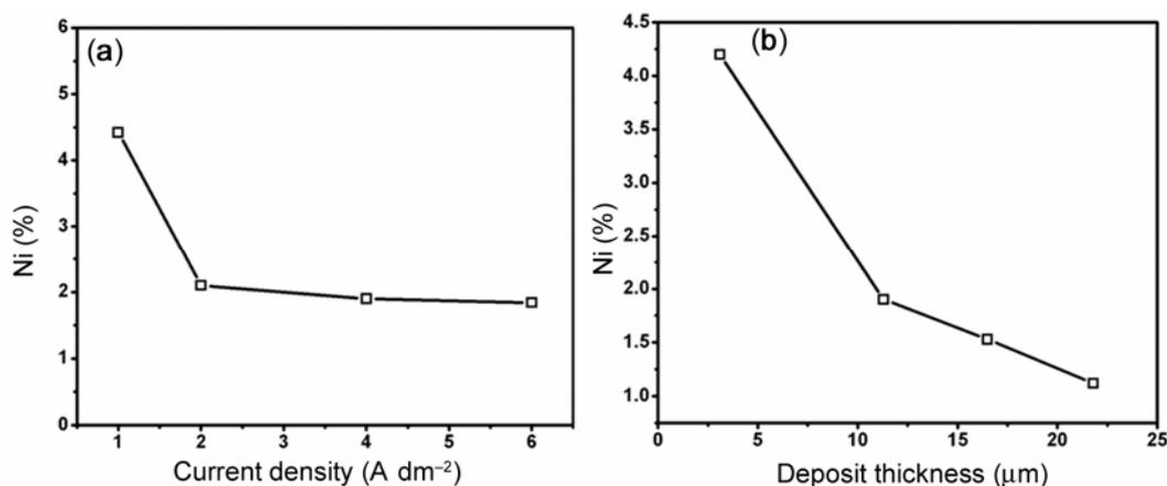
**Figure 1.** Effect of (a) current density and (b) thickness of coating on the composition of ZnNi deposit obtained from optimized bath.
