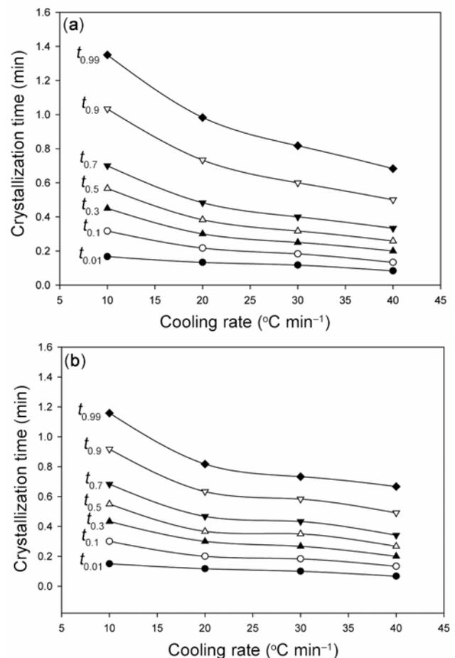
**Figure 4.** Crystallization time at various relative crystallinity values as a function of cooling rate for (a) pure PE and (b) PECN15.
