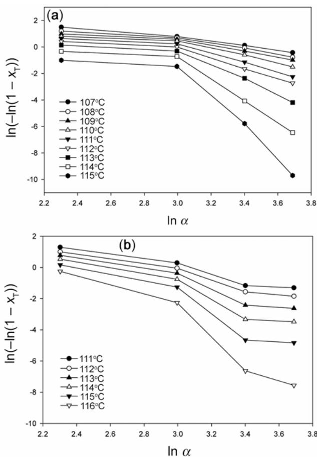
Figure 7. Ozawa plots of (a) pure PE and (b) PECN15 during non-isothermal crystallization.
