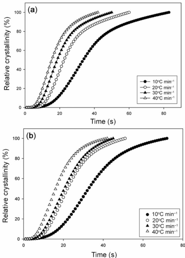
**Figure 3.** Relative crystallinity as a function of time for non-isothermal crystallization of (a) pure PE and (b) PECN15 at different cooling rates.
