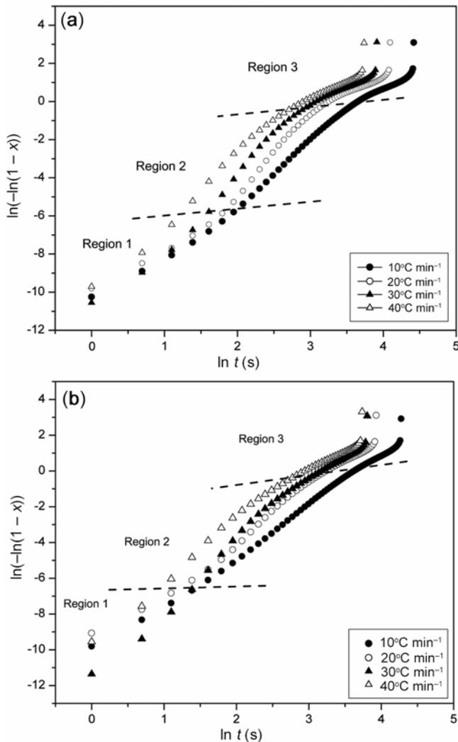
**Figure 6.** Avrami plots of (a) pure PE and (b) PECN15 at different cooling rates.
