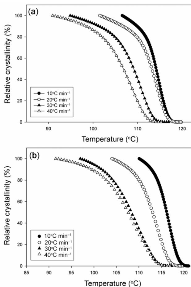
**Figure 2.** Relative crystallinity as a function of temperature for non-isothermal crystallization of (a) pure PE and (b) PECN15 at different cooling rates.
