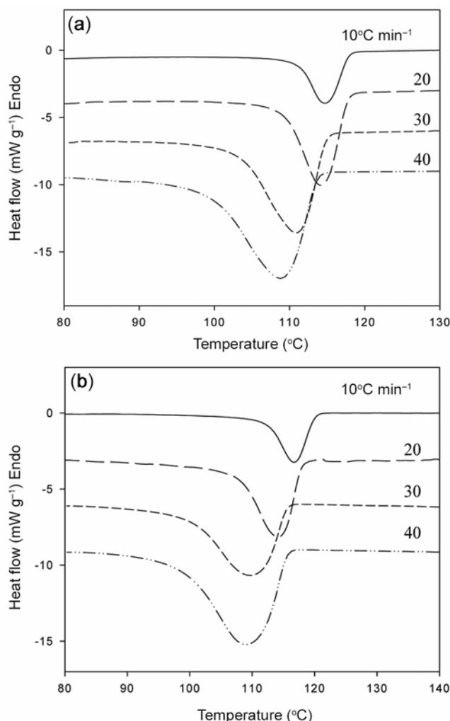
**Figure 1.** Non-isothermal crystallization curves for (a) pure PE and (b) PECN15 at different cooling rates.
