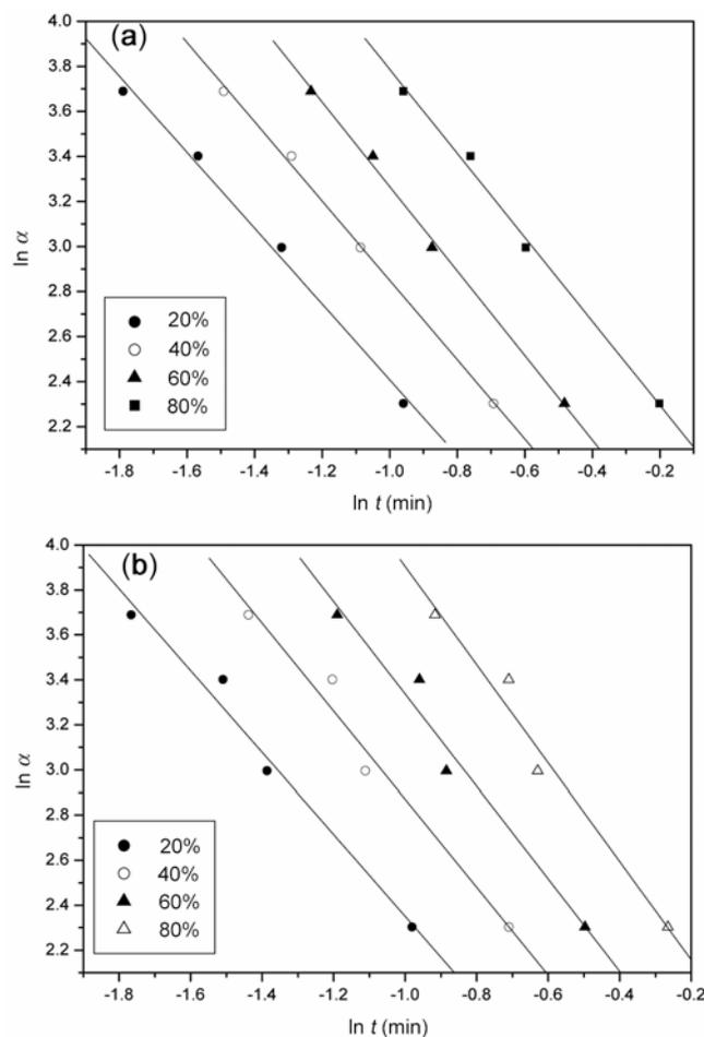
Figure 8. Plot of  $\ln \alpha$  as a function of  $\ln t$  for (a) pure PE and (b) PECN15 at different relative degree of crystallinity.
