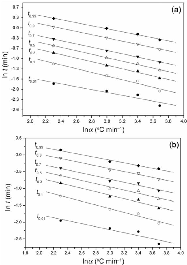
**Figure 5.** Crystallization time at various relative crystallinity values as a function of cooling rate for (a) pure PE and (b) PECN15.
