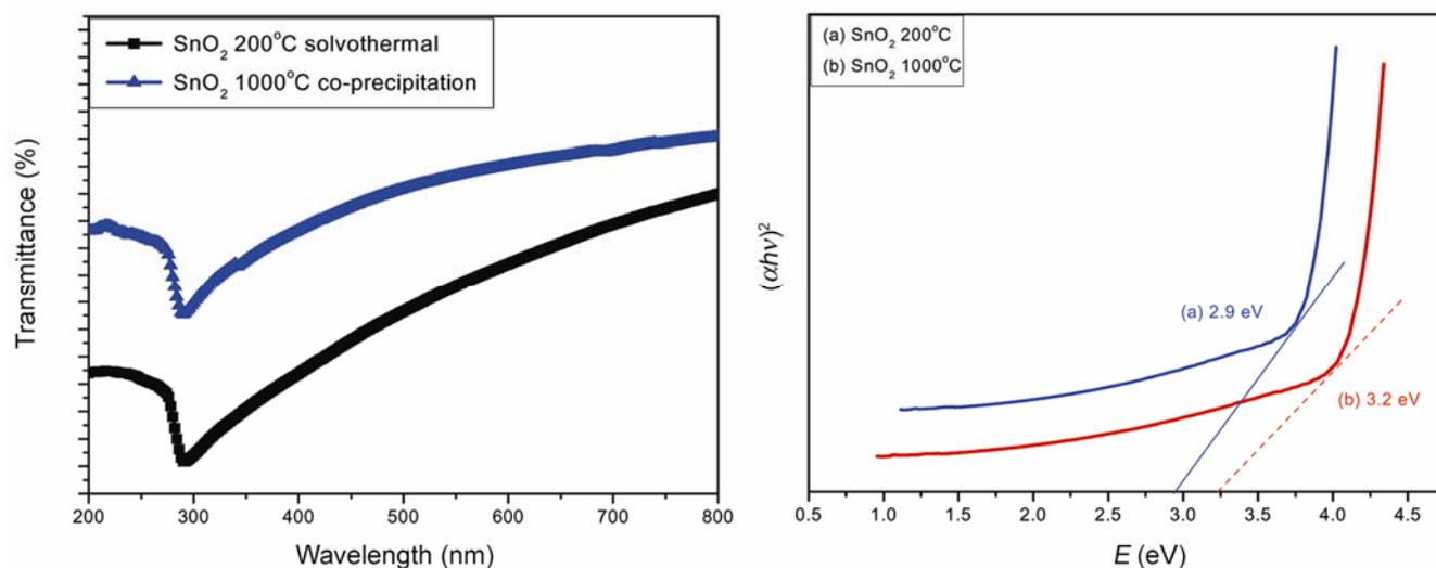
**Figure 3.** UV-Vis  $T\%$  and band gap of the as-prepared samples using two methods (a) co-precipitation method and (b) solvothermal method, respectively.
