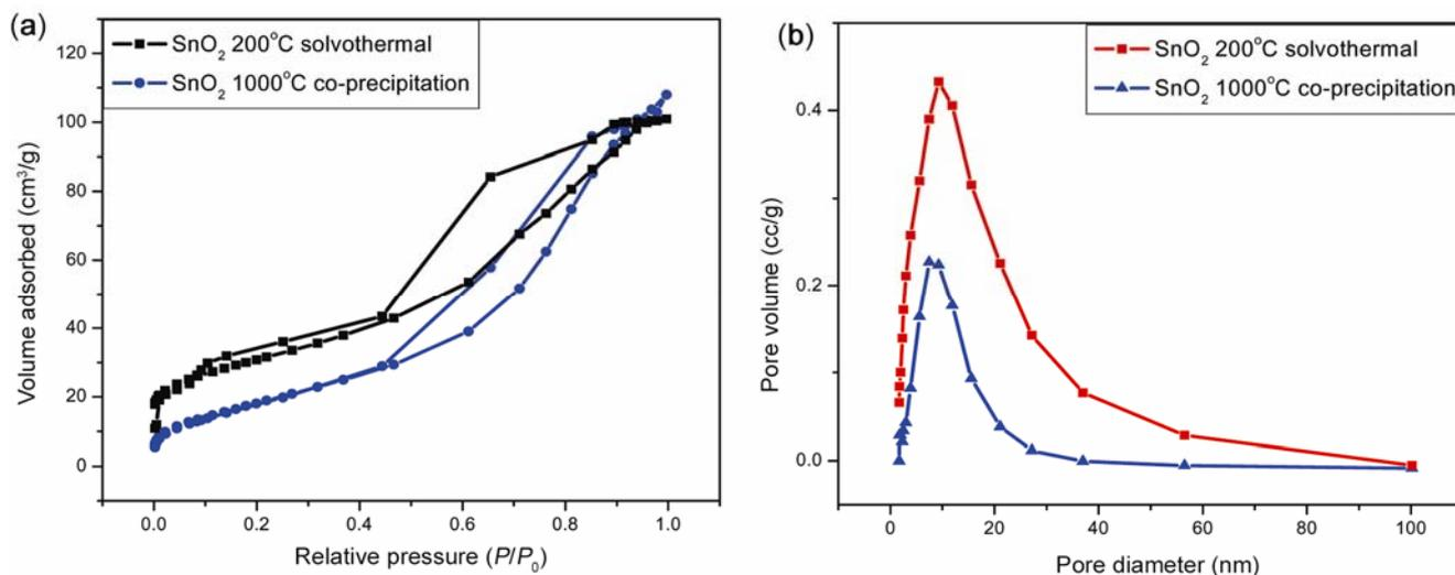
**Figure 2.** (a)  $N_2$  adsorption–desorption isotherms surface area and (b) corresponding pore size distribution of the as-prepared samples using two methods: co-precipitation and solvothermal methods.
