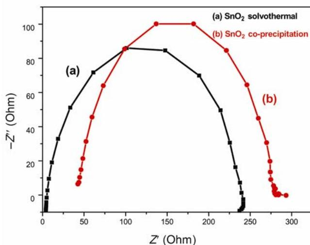
**Figure 5.** Nyquist diagrams of the impedance spectra of (a) DSSCs based on  $\text{SnO}_2$  nanopowders solvothermal method compared to (b) DSSCs based on  $\text{SnO}_2$  nanopowders co-precipitation method.
