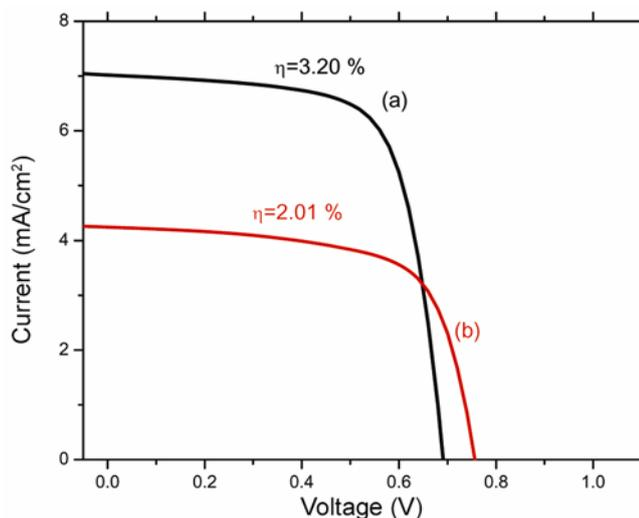
**Figure 4.** Comparison of the  $I$ - $V$  characteristics of DSSCs made from (a)  $\text{SnO}_2$  nanopowders solvothermal method and (b)  $\text{SnO}_2$  nanopowders co-precipitation method.
