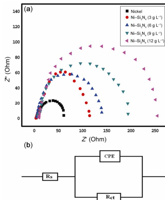
**Figure 7.** (a) Nyquist diagrams of impedance spectrum of electrodeposited nickel and Ni-Si<sub>3</sub>N<sub>4</sub> nanocomposite coatings. (■) Electrodeposited nickel, (●) Ni-Si<sub>3</sub>N<sub>4</sub> (3 g L<sup>-1</sup>), (▲) Ni-Si<sub>3</sub>N<sub>4</sub> (6 g L<sup>-1</sup>), (▼) Ni-Si<sub>3</sub>N<sub>4</sub> (9 g L<sup>-1</sup>) and (◄) Ni-Si<sub>3</sub>N<sub>4</sub> (12 g L<sup>-1</sup>) and (b) equivalent electrical circuit.
