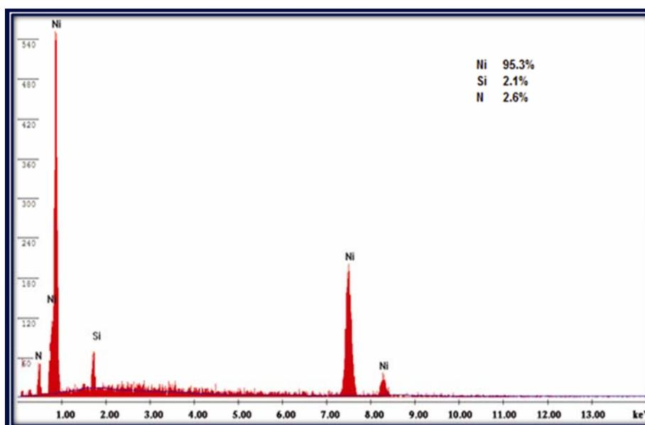
**Figure 4.** EDAX analysis spectrum of electrodeposited Ni-Si<sub>3</sub>N<sub>4</sub> (12 g L<sup>-1</sup>) nanocomposite coatings.
