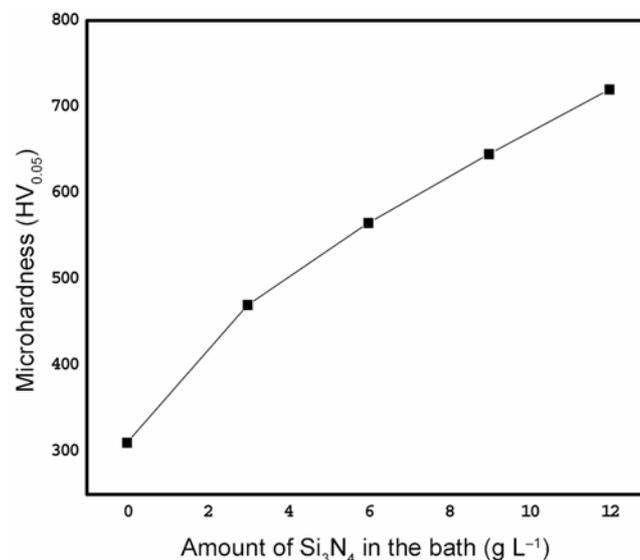
**Figure 6.** Effect of Si<sub>3</sub>N<sub>4</sub> content on hardness of coatings.
