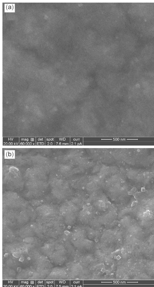
**Figure 5.** SEM photographs of (a) electrodeposited nickel and (b) Ni-Si<sub>3</sub>N<sub>4</sub> (12 g L<sup>-1</sup>) nanocomposite coatings.
