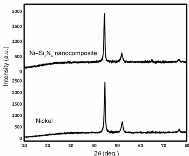
**Figure 3.** XRD patterns of (a) electrodeposited nickel and (b) Ni-Si<sub>3</sub>N<sub>4</sub> nanocomposite coating.
