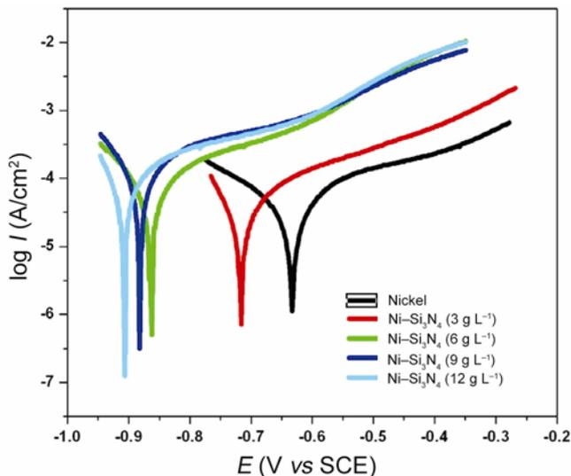
**Figure 8.** Potentiodynamic polarization curves of electrodeposited nickel and Ni-SiO<sub>2</sub> nanocomposite coatings. (a) Electrodeposited nickel, (b) Ni-Si<sub>3</sub>N<sub>4</sub> (3 g L<sup>-1</sup>), (c) Ni-Si<sub>3</sub>N<sub>4</sub> (6 g L<sup>-1</sup>), (d) Ni-Si<sub>3</sub>N<sub>4</sub> (9 g L<sup>-1</sup>) and (e) Ni-Si<sub>3</sub>N<sub>4</sub> (12 g L<sup>-1</sup>).
