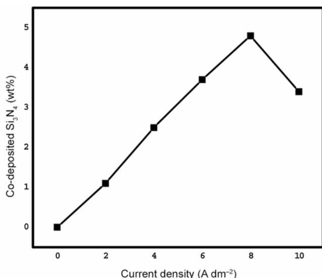
**Figure 2.** Effect of current density on weight percentage of Si<sub>3</sub>N<sub>4</sub> in nanocomposite coatings containing Si<sub>3</sub>N<sub>4</sub> (12 g L<sup>-1</sup>).
