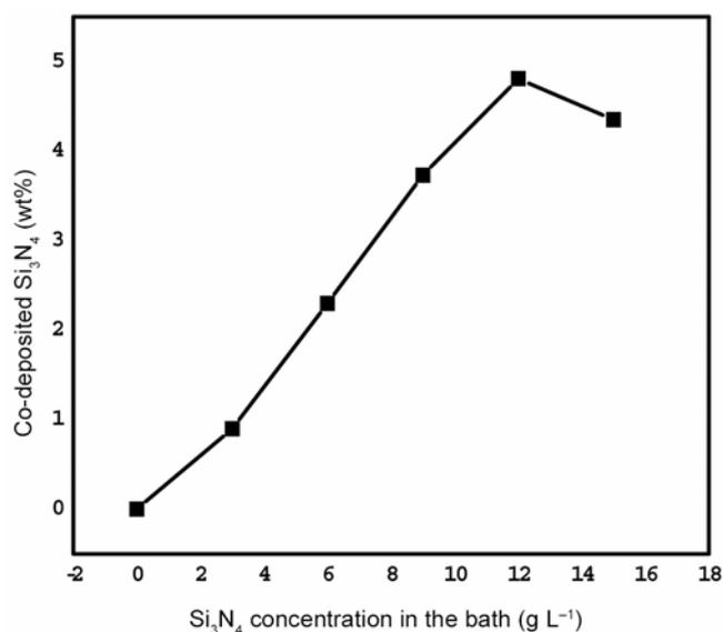
**Figure 1.** Effect of amount of Si<sub>3</sub>N<sub>4</sub> in bath (in grams per litre) on weight percentage of Si<sub>3</sub>N<sub>4</sub> in nanocomposite coatings.
