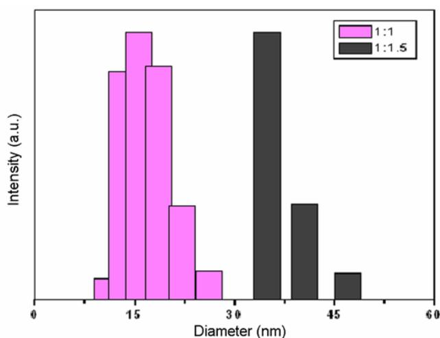
**Figure 3.** Particle size distribution of 1:1 and 1:1.5 ZnO nanocolloids.
