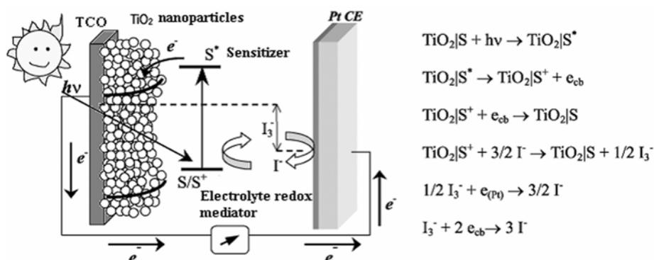
**Figure 10.** Schematic diagram showing working of DSSC and role of dye.
