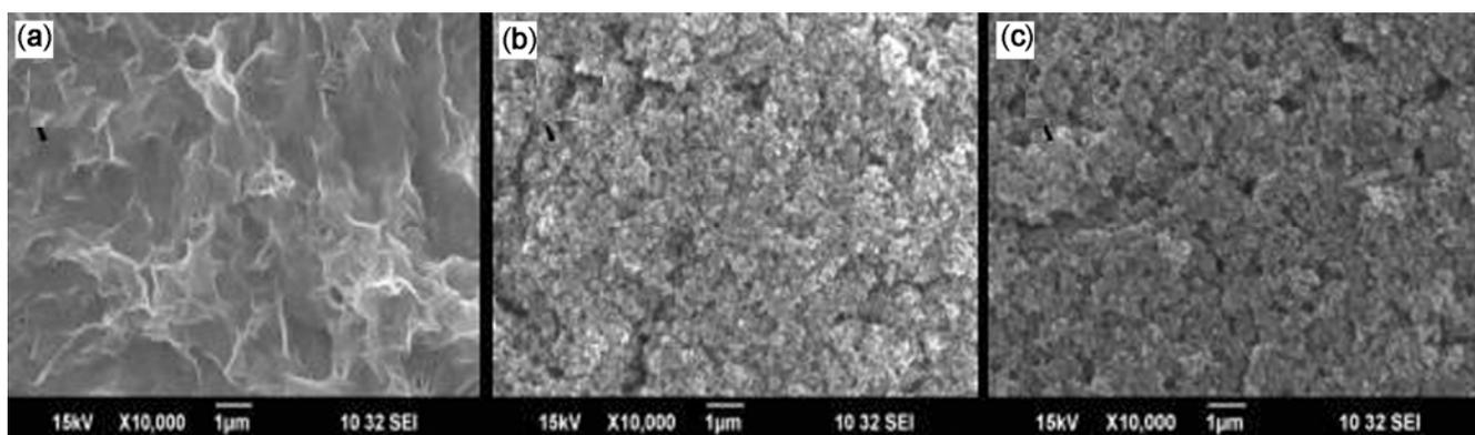
**Figure 2.** SEM images of (a) ZnO thin film, (b) mesoporous TiO<sub>2</sub> thin film and (c) ZnO coated TiO<sub>2</sub> thin film.
