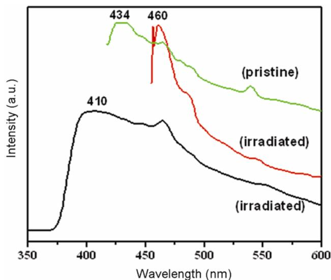
**Figure 8.** PL spectra of Al<sub>2</sub>O<sub>3</sub>:C (a) pristine sample and (b), (c) irradiated samples.
