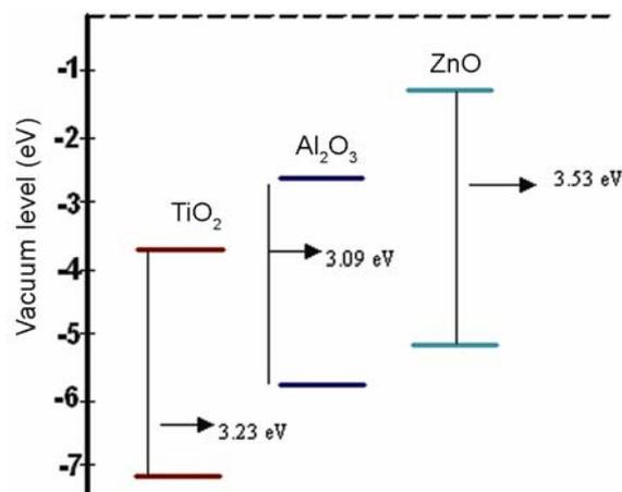
**Figure 9.** Schematic diagram of the electrochemically determined HOMO and LUMO of TiO<sub>2</sub>, ZnO and Al<sub>2</sub>O<sub>3</sub>.
