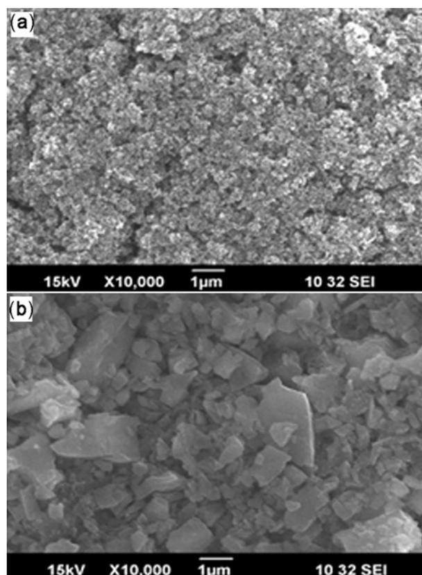
**Figure 7.** SEM images of (a) mesoporous TiO<sub>2</sub> thin film and (b) Al<sub>2</sub>O<sub>3</sub> : C-coated TiO<sub>2</sub> film.
