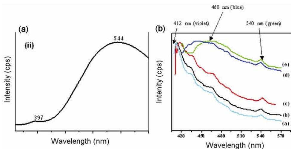
**Figure 4.** Photoluminescence spectra of (a) ZnO suspension and (b) ZnO thin film.
