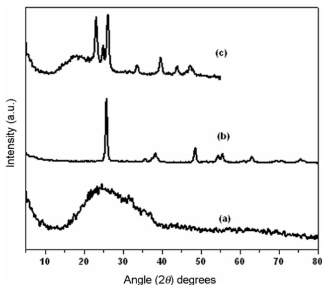
**Figure 1.** X-ray diffractograms of (a) amorphous ZnO, (b) crystalline ZnO and (c) ZnO coated over  $\text{TiO}_2$ .
