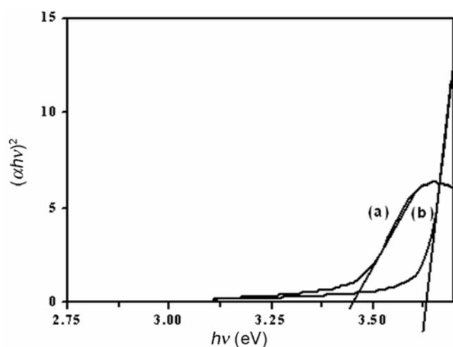
**Figure 5.** Bandgap determination of ZnO of colloidal suspension: (a) 1 : 1.5 and (b) 1 : 1.
