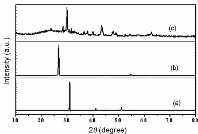
**Figure 6.** X-ray diffractograms of (a) Al<sub>2</sub>O<sub>3</sub>, (b) graphite and (c) Al<sub>2</sub>O<sub>3</sub> : C.
