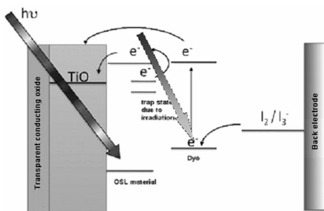
**Figure 11.** Schematic diagram showing combined action of solid-state absorber and dye in DSSC.
