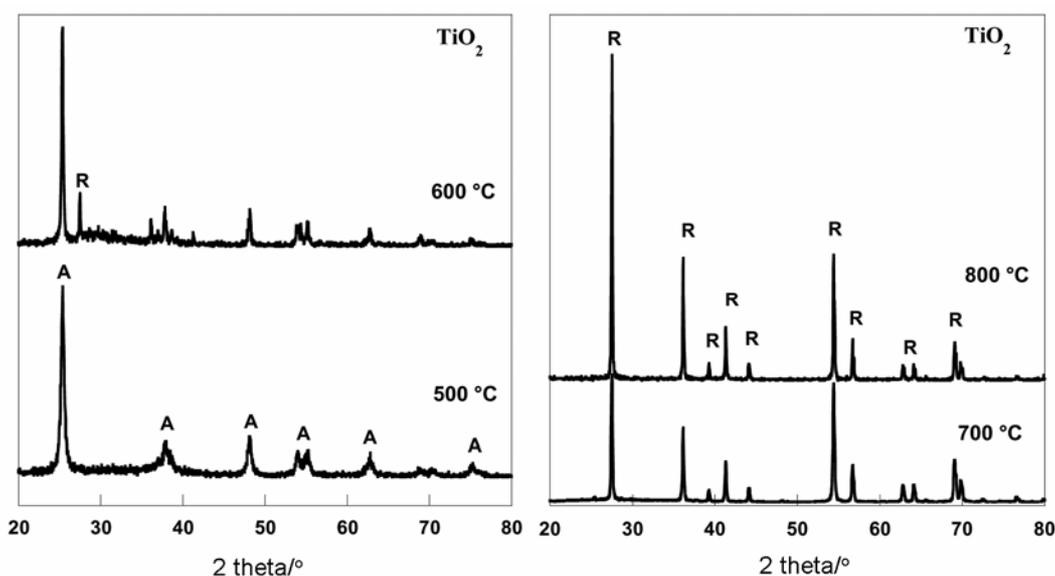
**Figure 3.** *In situ* XRD diffractograms of TiO<sub>2</sub> and A: anatase and R: rutile.
