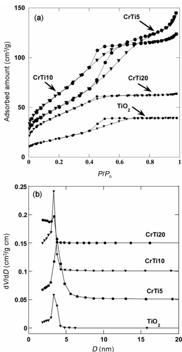
**Figure 1.** (a) Isotherms for adsorption of nitrogen on CrTiX samples and (b) pore size distributions measured in samples.
