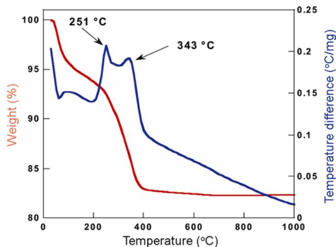
**Figure 2.** TGA-DTA curves of TiO<sub>2</sub> before calcination.
