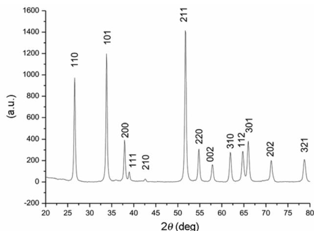
**Figure 1.** X-ray diffraction pattern for Sn<sub>0.95</sub>Co<sub>0.05</sub>O<sub>2</sub> nanocrystalline.
