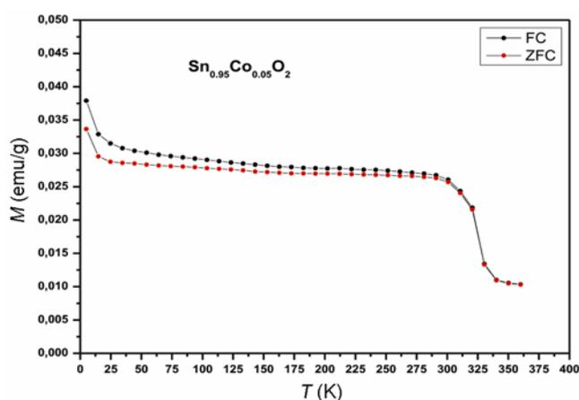
**Figure 2.** Magnetization vs temperature measured on a  $\text{Sn}_{0.95}\text{Co}_{0.05}\text{O}_2$  nanocrystalline at external magnetic field of 500 Oe.
