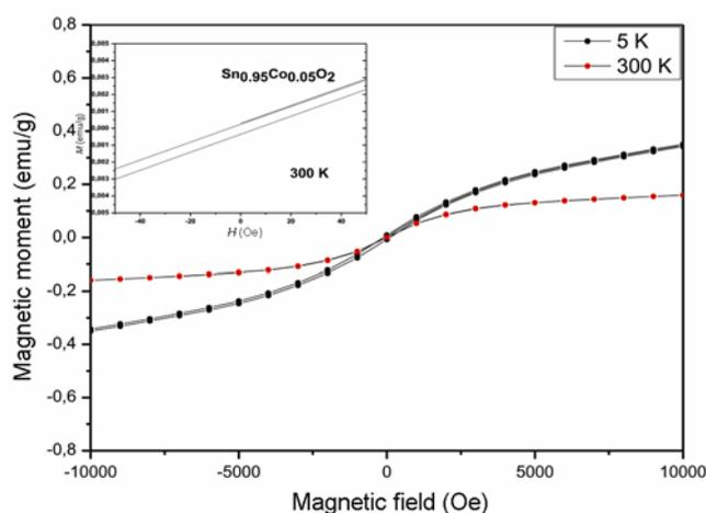
**Figure 3.** Magnetic hysteresis loops of  $\text{Sn}_{0.95}\text{Co}_{0.05}\text{O}_2$  nanocrystalline at temperatures 5 and 300 K.
