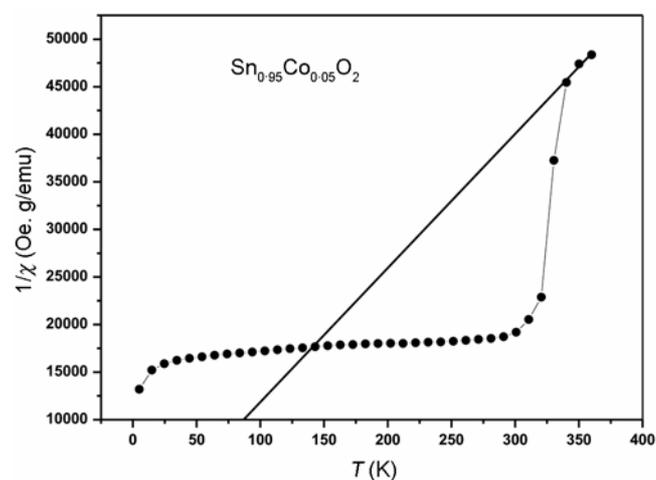
**Figure 4.** Inverse magnetic susceptibility vs temperature for  $\text{Sn}_{0.95}\text{Co}_{0.05}\text{O}_2$  nanocrystalline.
