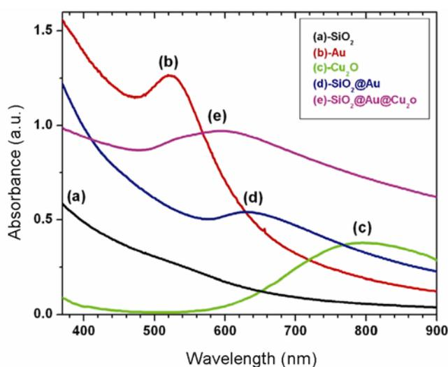
**Figure 7.** Optical absorption (UV-Vis) of silica, Au,  $\text{Cu}_2\text{O}$ ,  $\text{SiO}_2\text{-Au}$  core/shell nanoparticles and  $\text{SiO}_2\text{-Au-Cu}_2\text{O}$  core/shell/shell nanoparticles.
