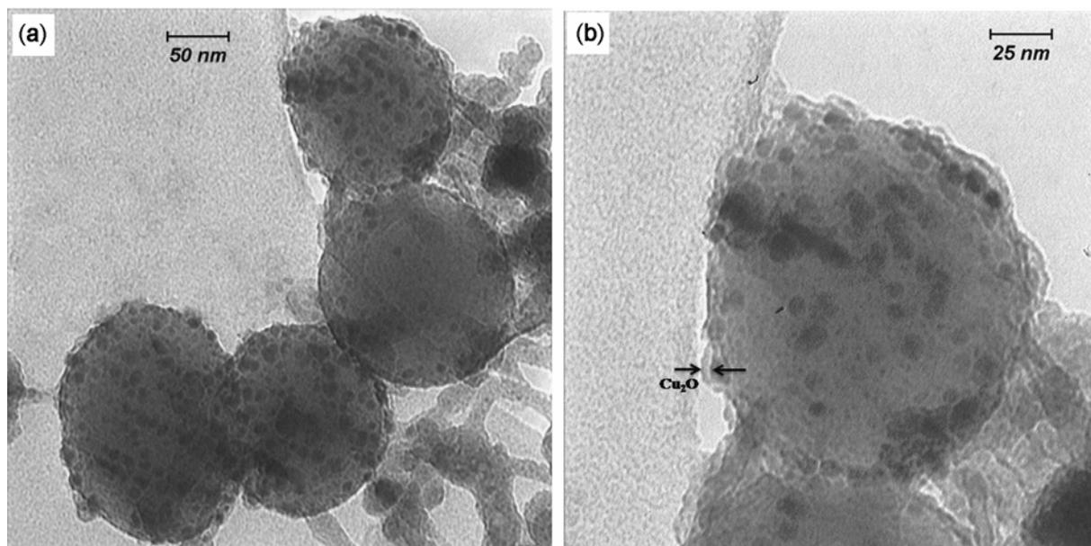
**Figure 4.** TEM images of SiO<sub>2</sub>-Au-Cu<sub>2</sub>O core/shell/shell nanoparticles.
