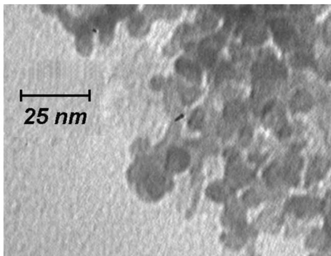
**Figure 5.** TEM image of colloidal gold nanoparticles.
