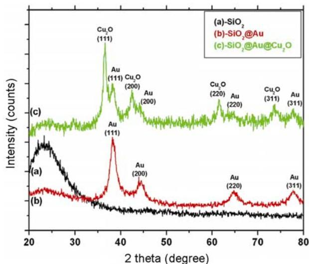
**Figure 1.** XRD patterns of (a) pure silica nanoparticles, (b)  $\text{SiO}_2\text{-Au}$  core/shell nanoparticles and (c)  $\text{SiO}_2\text{-Au-Cu}_2\text{O}$  core/shell/shell nanoparticles.
