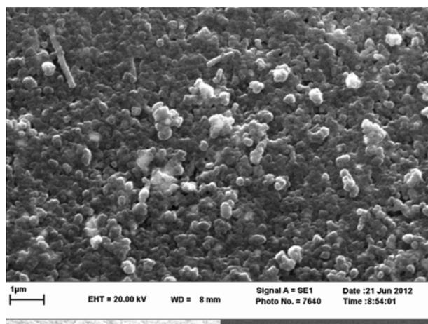
**Figure 2.** SEM images of  $\text{SiO}_2\text{-Au-Cu}_2\text{O}$  core/shell/shell nanoparticles.
