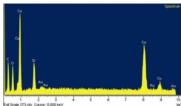
**Figure 3.** EDX spectra of  $\text{SiO}_2\text{-Au-Cu}_2\text{O}$  core/shell/shell nanoparticles.
