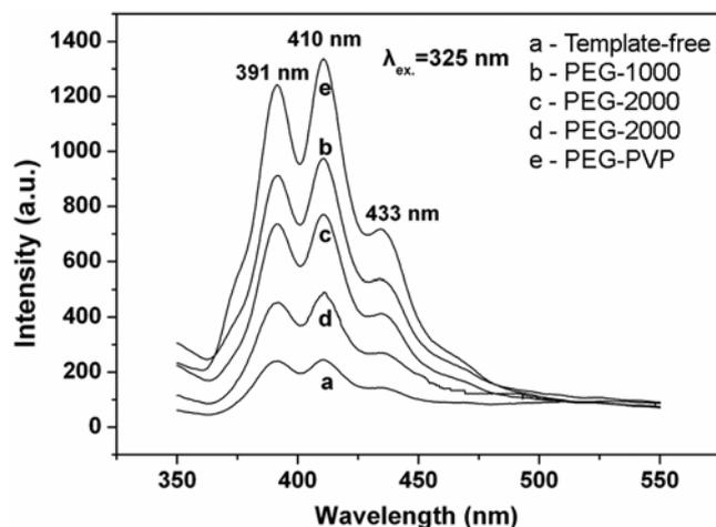
**Figure 7.** Emission spectra of ZnO:Al:Mo films deposited with and without template.
