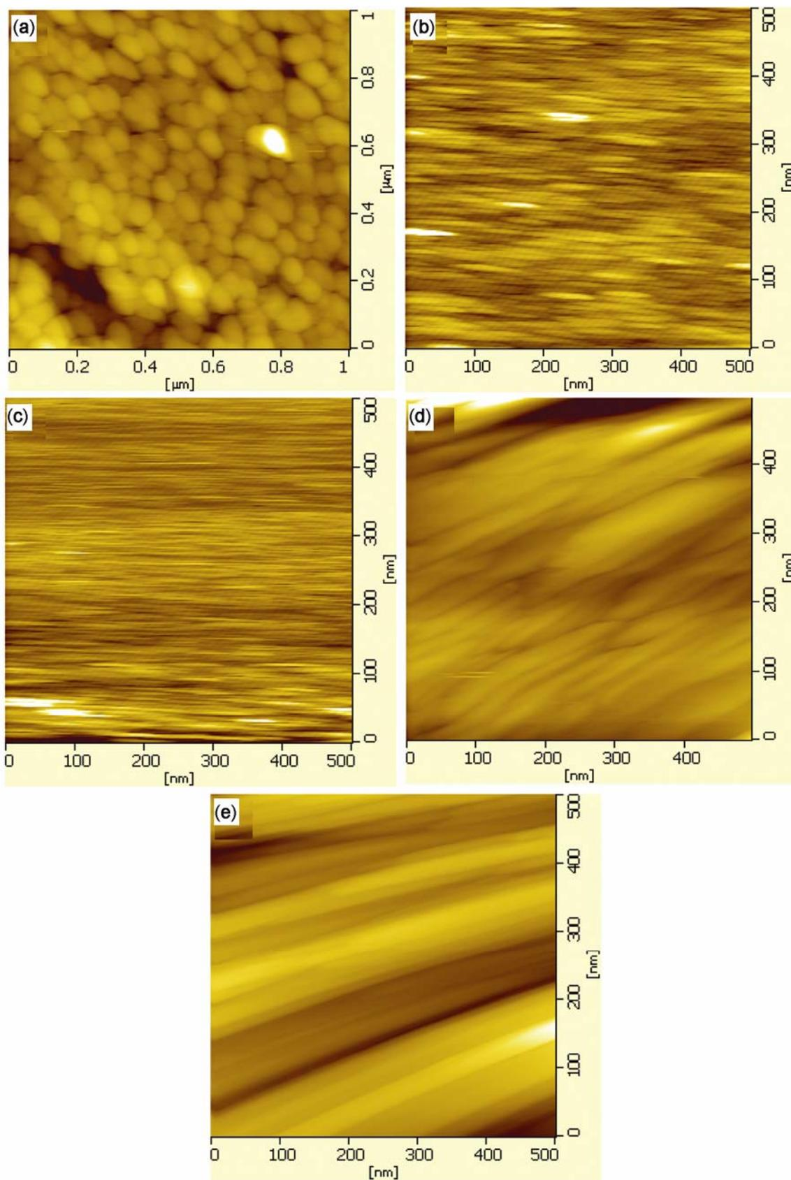
**Figure 2.** AFM micrographs of ZnO : Al : Mo films deposited (a) without and with template, (b) PEG-1000, (c) PEG-2000, (d) PEG-4000 and (e) PVP.
