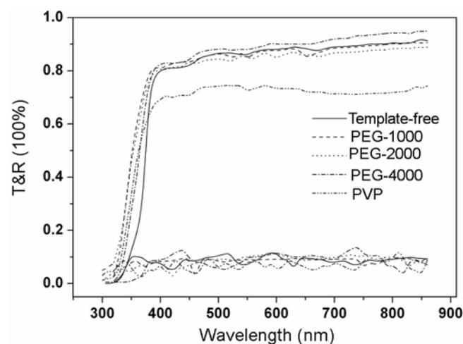
**Figure 4.** Transmittance and reflectance spectra of ZnO:Al:Mo films deposited with and without template.
