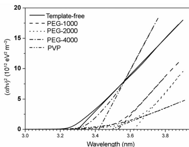
**Figure 5.** Plots of  $(\alpha h\nu)^2$  vs  $h\nu$  for ZnO:Al:Mo films deposited with and without template.
