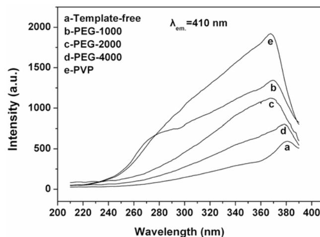
**Figure 6.** Excitation spectra of ZnO:Al:Mo films deposited with and without template.
