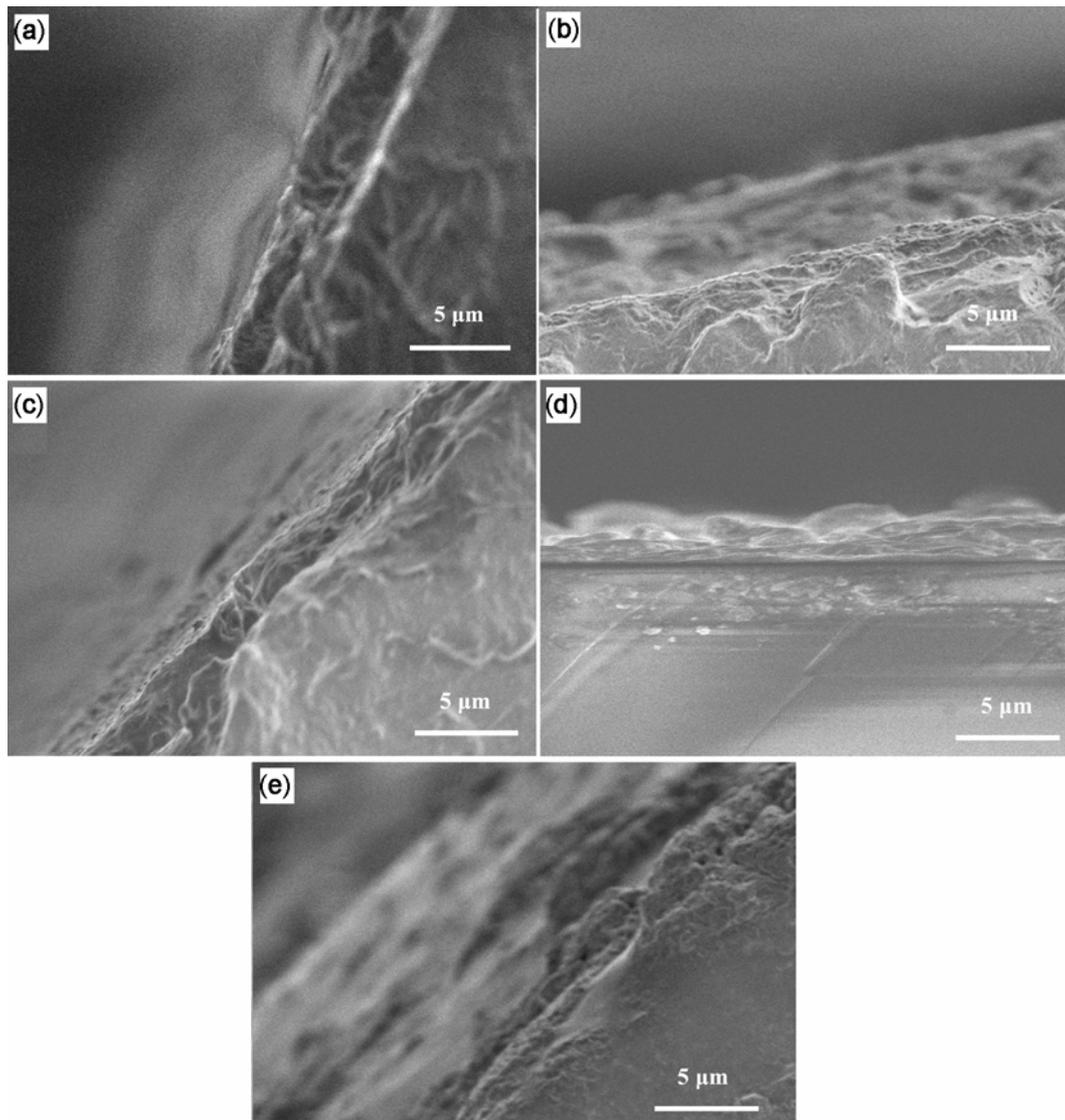
**Figure 3.** Cross-section SEM micrographs of ZnO:Al:Mo films deposited (a) without and with template, (b) PEG-1000, (c) PEG-2000, (d) PEG-4000 and (e) PVP.
