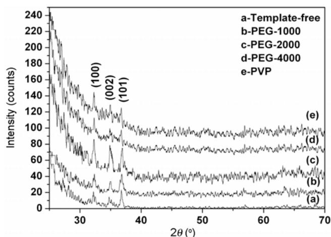
**Figure 1.** XRD patterns of ZnO:Al:Mo films deposited with and without template.
