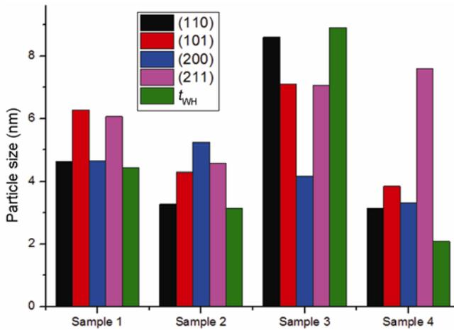
**Figure 3.** Comparison of particle size calculated by DS formula along each plane (110), (101), (200) and (211) and WH plot of all samples.
