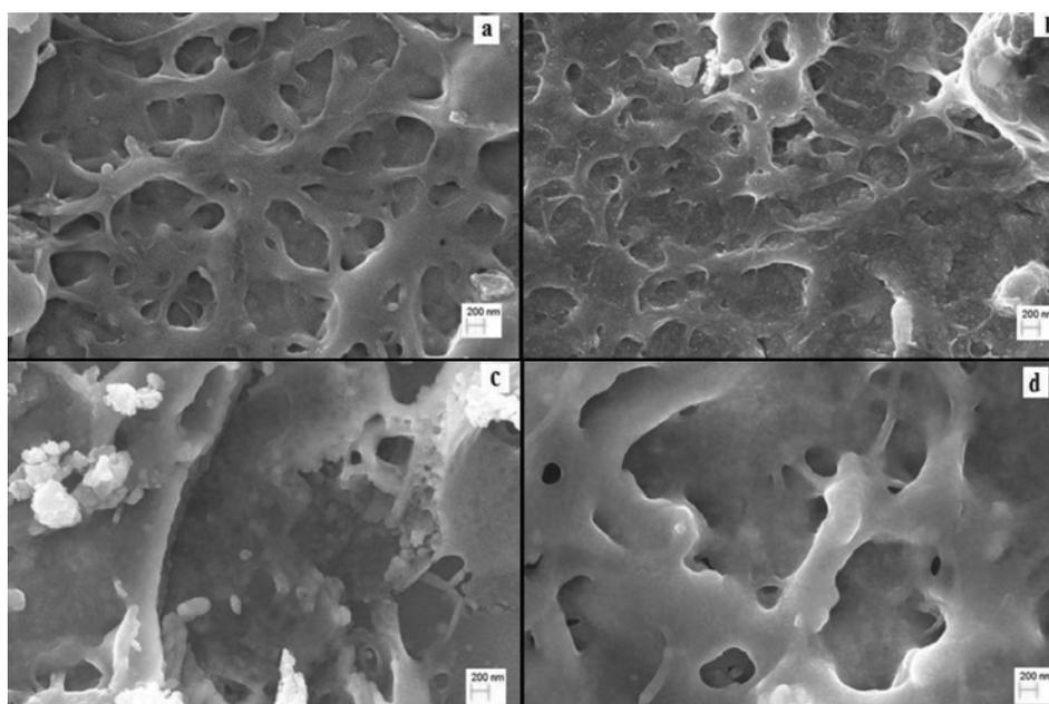
**Figure 5.** SEM images of samples 1, 2, 3 and 4. Images (a), (b), (c) and (d) correspond to samples 1, 2, 3 and 4, respectively i.e. SnO<sub>2</sub> thin films of 0.2, 0.4, 0.6 and 0.8 M precursors.
