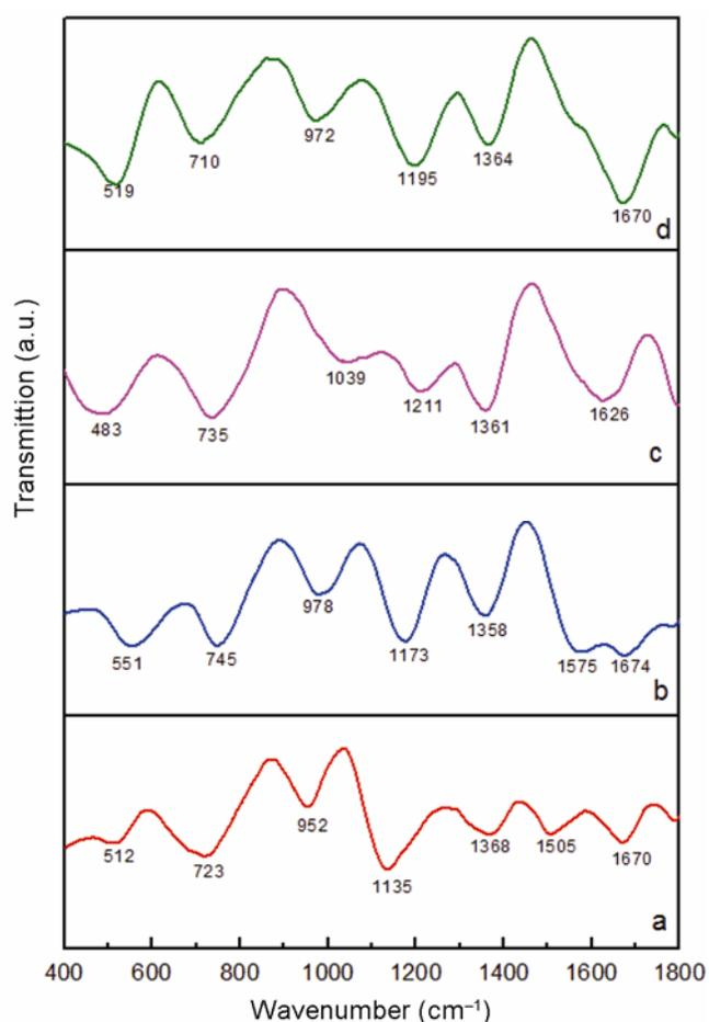
**Figure 6.** FT-IR spectra of samples 1, 2, 3 and 4. Curves (a), (b), (c) and (d) correspond to samples 1, 2, 3, and 4, respectively i.e. SnO<sub>2</sub> thin films of 0.2, 0.4, 0.6 and 0.8 M precursors.
