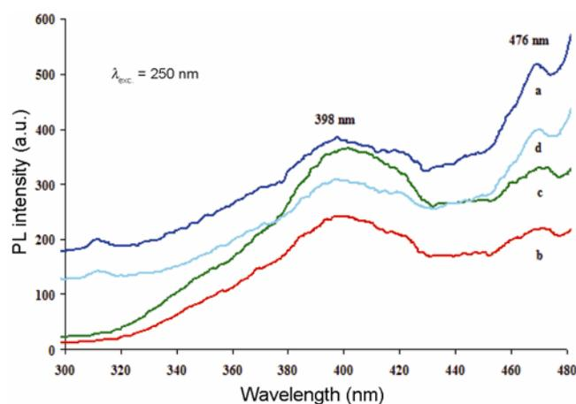
**Figure 8.** PL spectra of samples 1, 2, 3 and 4 at excitation wavelength of 250 nm. Curves a, b, c and d correspond to samples 1, 2, 3 and 4, respectively i.e. SnO<sub>2</sub> thin films of 0.2, 0.4, 0.6 and 0.8 M precursors.
