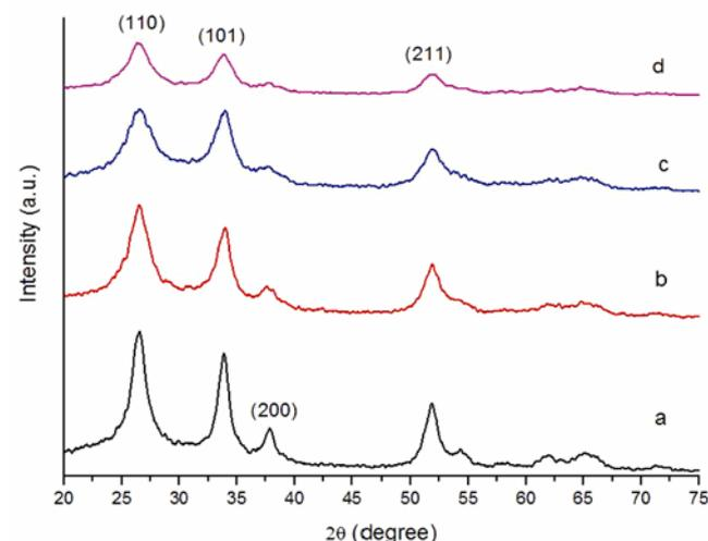
**Figure 1.** XRD spectra of samples 1, 2, 3 and 4. Images (a), (b), (c) and (d) correspond to samples 1, 2, 3 and 4, respectively i.e. SnO<sub>2</sub> thin films of 0.2, 0.4, 0.6 and 0.8 M precursors.
