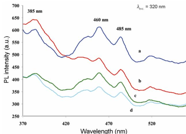
**Figure 9.** PL spectra of samples 1, 2, 3 and 4 at excitation wavelength of 320 nm. Curves a, b, c and d correspond to samples 1, 2, 3 and 4, respectively i.e. SnO<sub>2</sub> thin films of 0.2, 0.4, 0.6 and 0.8 M precursors.
