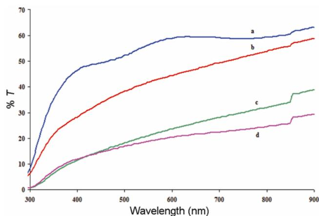
**Figure 7.** Transmission spectra of samples 1, 2, 3 and 4. Curves a, b, c and d correspond to samples 1, 2, 3 and 4, respectively i.e. SnO<sub>2</sub> thin films of 0.2, 0.4, 0.6 and 0.8 M precursors.
