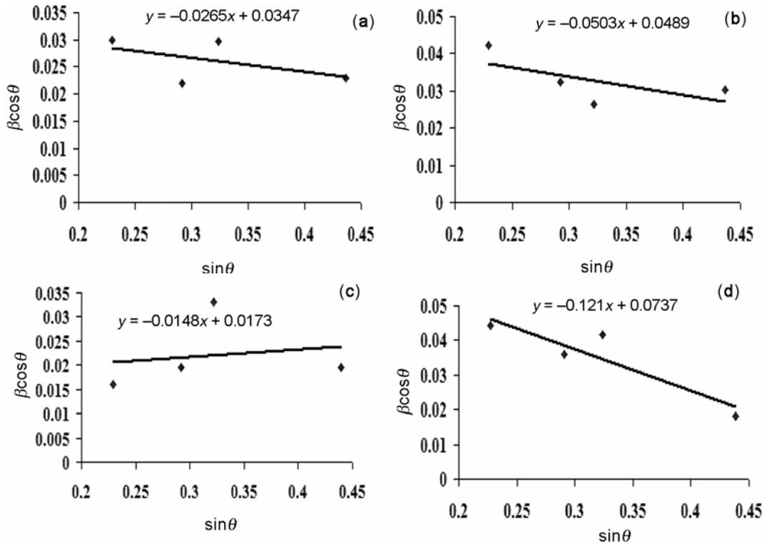
**Figure 2.** Williamson–Hall plots of samples 1, 2, 3 and 4. Images (a), (b), (c) and (d) correspond to samples 1, 2, 3 and 4, respectively i.e. SnO<sub>2</sub> thin films of 0.2, 0.4, 0.6 and 0.8 M precursors.
