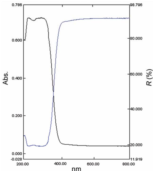
**Figure 1.** UV/DRS spectra of as received TiO<sub>2</sub> NPs showing absorption (black) and reflectance (blue) spectra.
