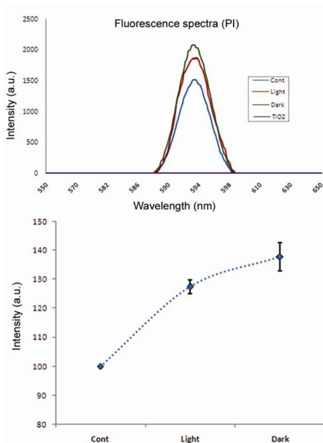
**Figure 8.** Fluorescence spectra of interacted cells under light condition (red), and dark condition (green). More intensity in dark interacted samples suggests presence of more damaged cells.
