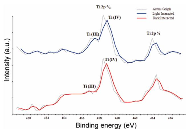
**Figure 5.** XPS Ti 2p spectra of TiO<sub>2</sub> interacted cells under light and dark conditions. Actual graphs are represented as dashed lines (...). Solid lights represent two-period moving average trend lines for light (blue) and dark (red) interacted samples.
