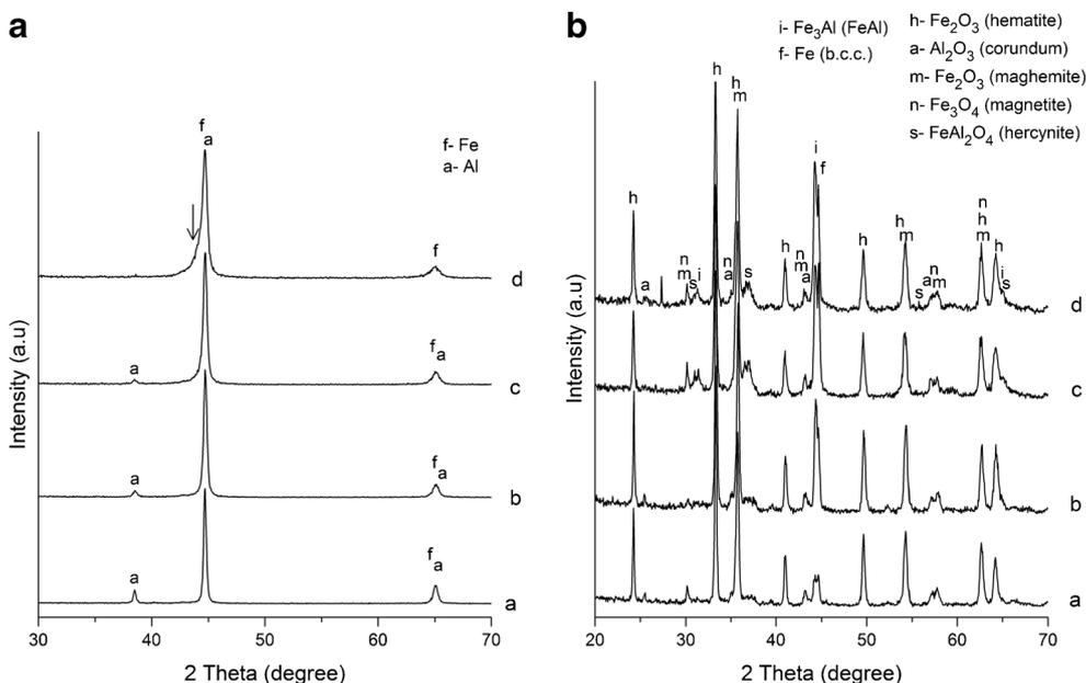
**Figure 1.** (a) XRD patterns of FeAl powders with different times of preliminary mechanochemical activation  $\tau_{\text{MA}}$  (min): a, 2; b, 5; c, 8 and d, -11 and (b) XRD patterns of  $\text{FeAlO}_y/\text{FeAl}_x$  made from FeAl powders with different times of preliminary mechanochemical activation  $\tau_{\text{MA}}$  (min): a, 2; b, 5; c, 8 and d, -11.
