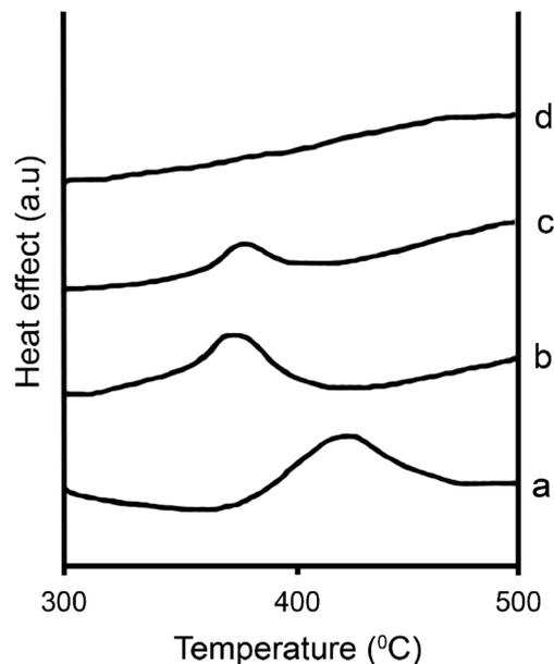
**Figure 4.** Thermal analysis data of Fe–Al precursors after MA and hydrothermal treatment in He flow. MA times: a, 2 min, b, 5 min, c, 8 min and d, 11 min.
