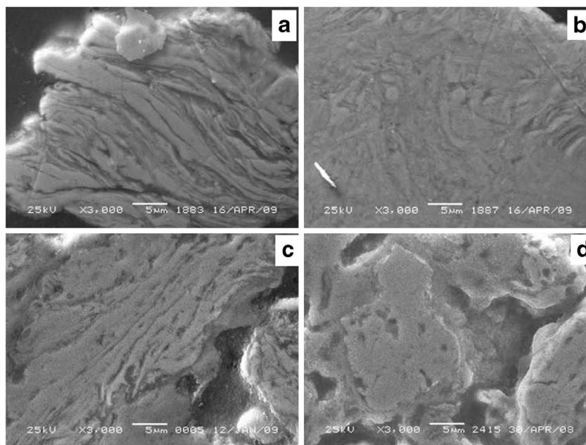
**Figure 2.** SEM micrographs of cores in FeAl powders (a,b) and  $\text{FeAlO}_y/\text{FeAl}_x$  cermets (c,d) prepared from FeAl powder with different MA times (min): a,c, -5 and b,d, -8.
