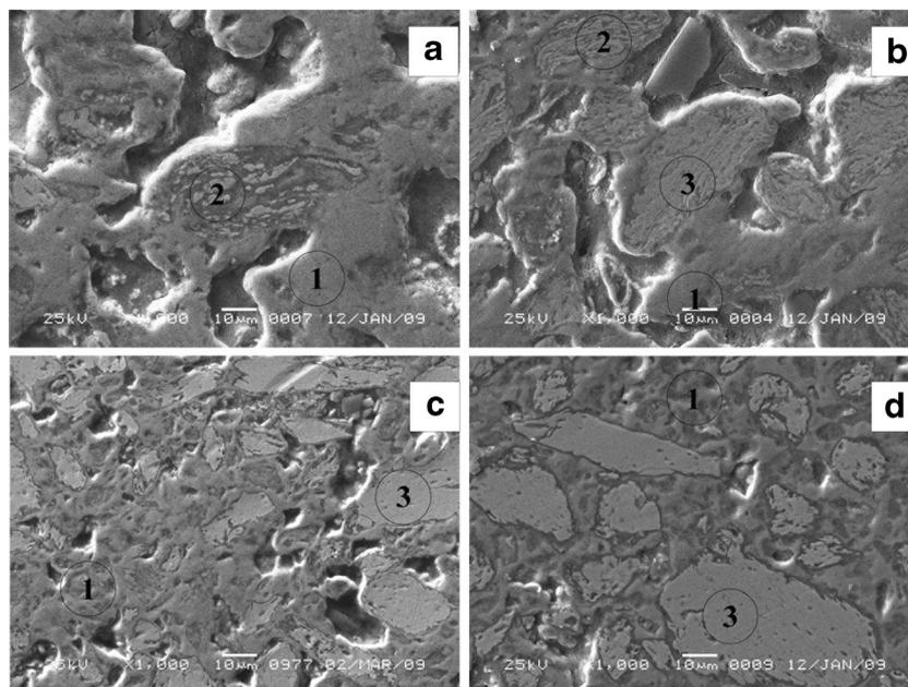
**Figure 5.** SEM micrographs of FeAlO<sub>y</sub>/FeAl<sub>x</sub> cermets prepared from FeAl powder after different MA times (min): a, 2; b, 5; c, 8 and d, -11. Different points were used for EDX analysis: (i) – (Fe<sub>2</sub>O<sub>3</sub>+ Al<sub>2</sub>O<sub>3</sub>); (ii) (Al<sub>2</sub>O<sub>3</sub>+Fe<sub>3</sub>O<sub>4</sub>+Fe<sup>0</sup>) or (Fe<sub>3</sub>O<sub>4</sub>+FeAl) and (iii) (Fe<sub>3</sub>Al or FeAl + Fe<sup>0</sup>).
