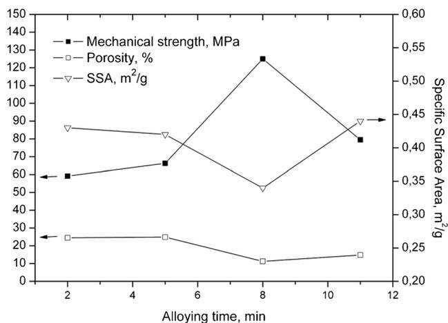
**Figure 6.** Dependence of specific surface area (i), porosity (ii) and crushing strength (iii) of FeAlO<sub>y</sub>/FeAl<sub>x</sub> cermets at time of preliminary mechano-chemical activation.
