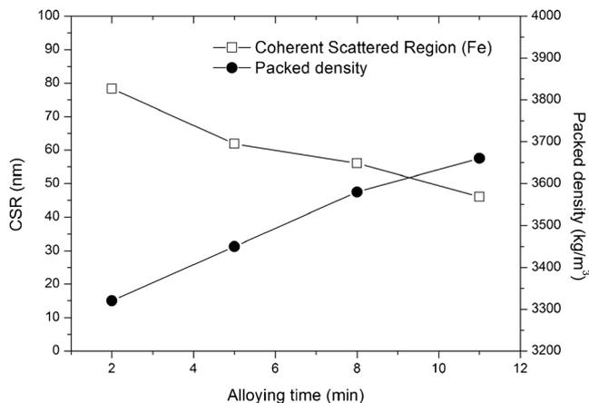
**Figure 3.** Dependence of powder packed density and Fe grain size (CSR) in FeAl powders on time of preliminary mechanochemical activation.
