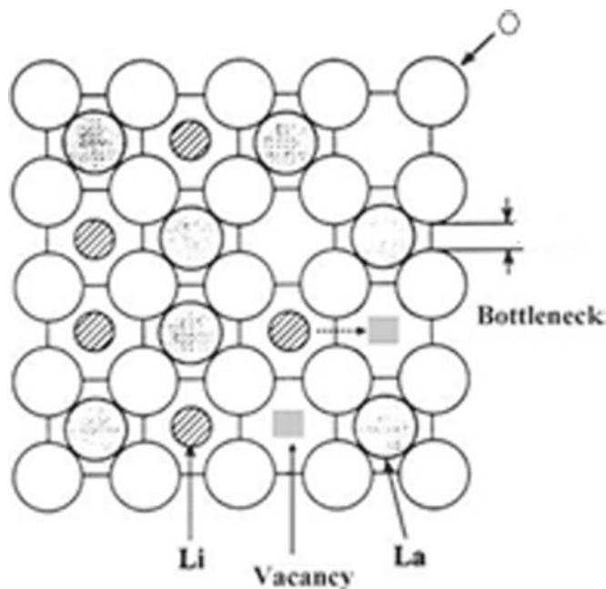
**Figure 1.** Schematic representation of bottleneck for lithium-ion conduction in perovskite-like structure (LLTO).
