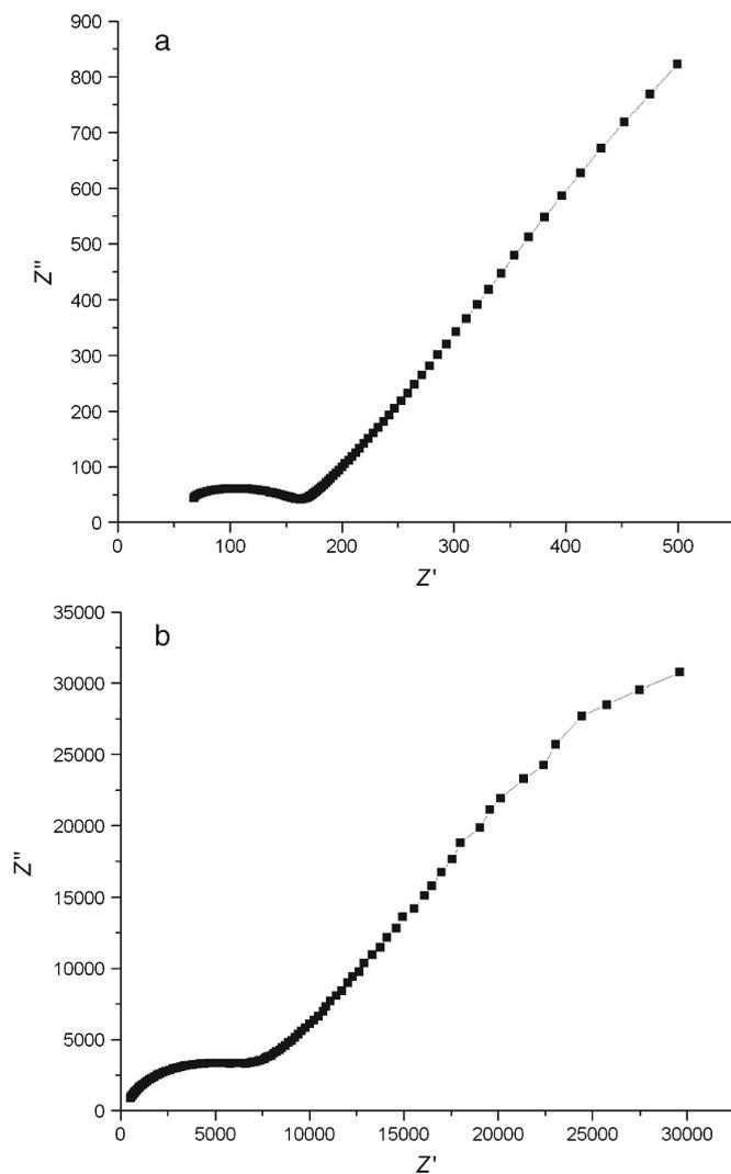
**Figure 7.** Complex impedance plot for (a) bulk conductivity and (b) grain boundary conductivity of  $\text{Li}_{0.29}\text{La}_{0.57}\text{TiO}_3$ .
