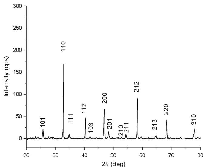
Figure 2. XRD pattern of  $\text{Li}_{0.29}\text{La}_{0.57}\text{TiO}_3$ .
