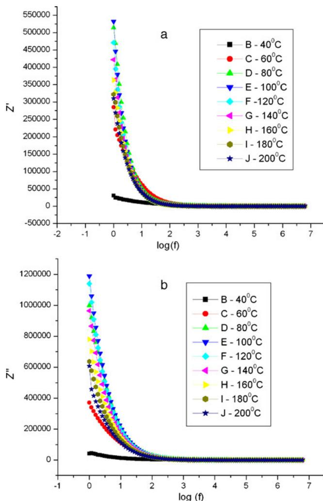
**Figure 9.** Variations of (a) real part of impedance ( $Z'$ ) and (b) imaginary part of impedance ( $Z''$ ) of  $\text{Li}_{0.29}\text{La}_{0.57}\text{TiO}_3$ .
