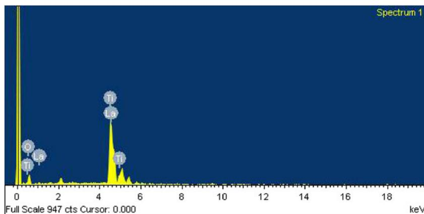
**Figure 4.** Energy dispersive spectrum of  $\text{Li}_{0.29}\text{La}_{0.57}\text{TiO}_3$ .
