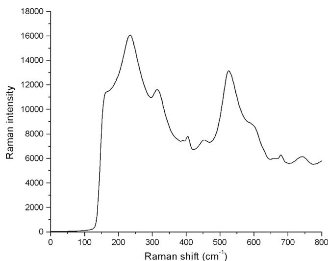
**Figure 6.** Raman spectrum of  $\text{Li}_{0.29}\text{La}_{0.57}\text{TiO}_3$ .
