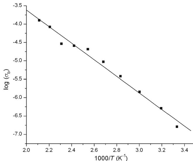
**Figure 8.** Arrhenius plot of bulk conductivity of  $\text{Li}_{0.29}\text{La}_{0.57}\text{TiO}_3$ .
