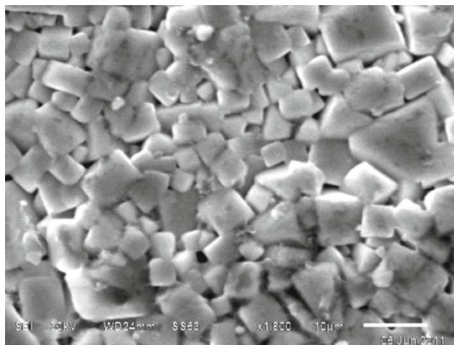
Figure 3. SEM micrograph of  $\text{Li}_{0.29}\text{La}_{0.57}\text{TiO}_3$ .
