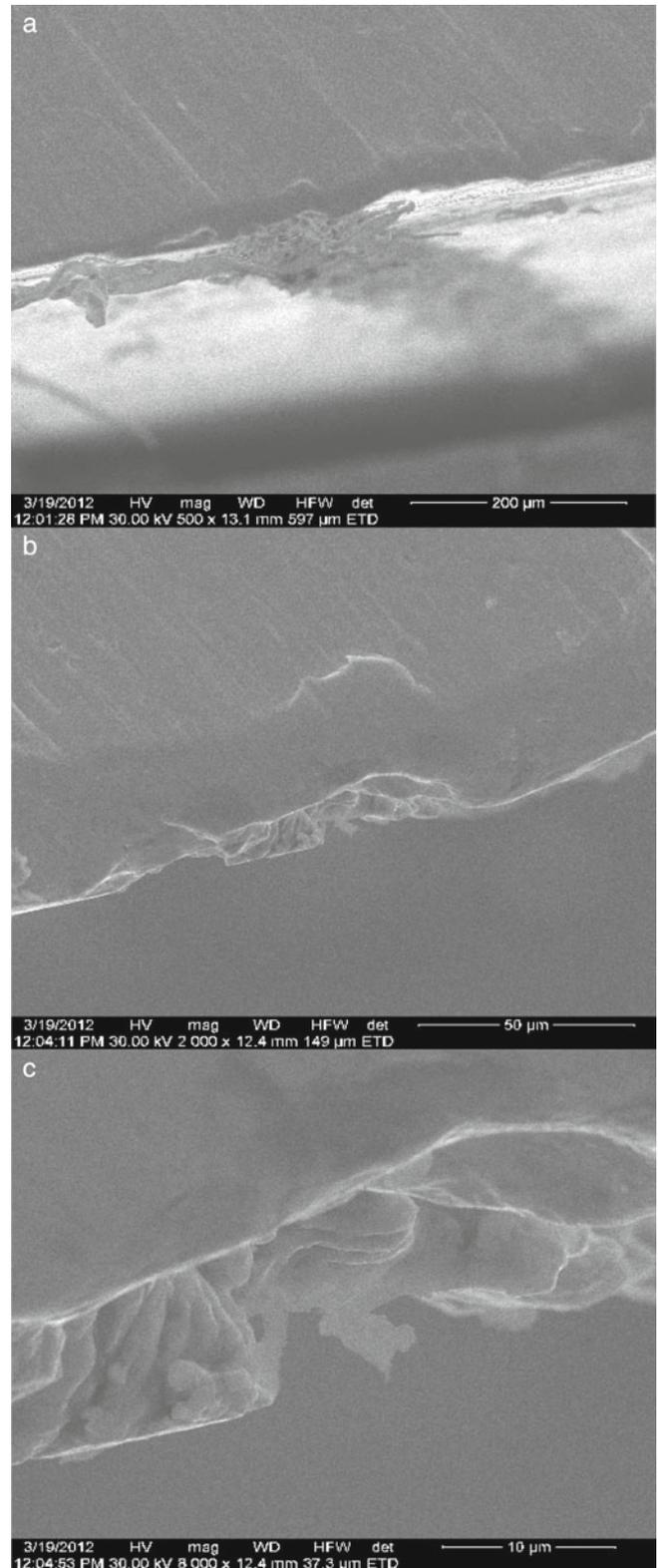
**Figure 4.** Mark cross-section SEM images: (a) general cross-section view of nanolaser mark ( $\times 500$ ); (b) profile of lower part of laser-created channel, which has a depth of  $\sim 25 \mu\text{m}$  ( $\times 2000$ ) and (c) detail showing bottom profile and sidewalls of mark segment ( $\times 8000$ ).
