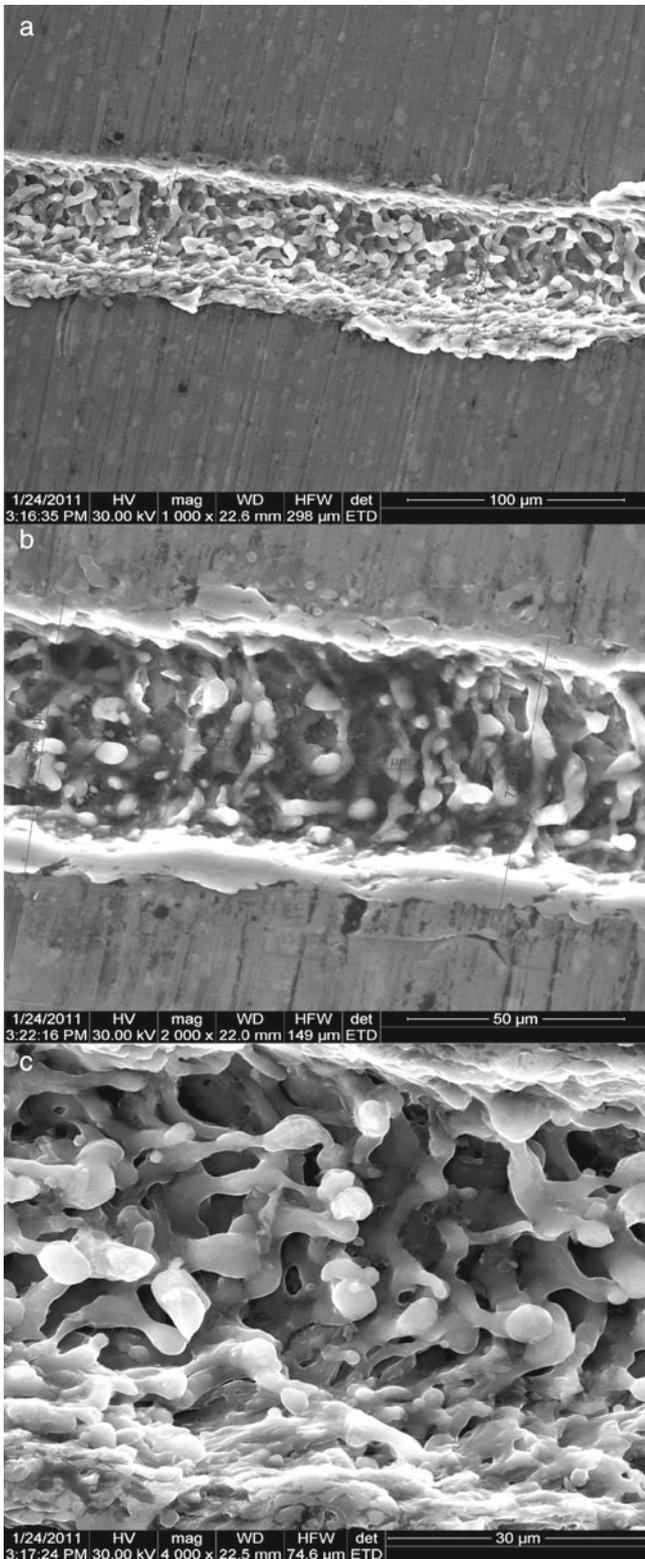
**Figure 3.** SEM micrographs of superimposed laser scans mark: (a) width of engraved segment and massive Al oxide deposits which follow scanning direction ( $\times 1000$ ); (b) molten material features and alloy dissipation within processed area, as droplets ( $\times 2000$ ) and (c) detail image showing ejected molten material from cavity and droplet form solidification of super-cooled Al alloy ( $\times 4000$ ).
