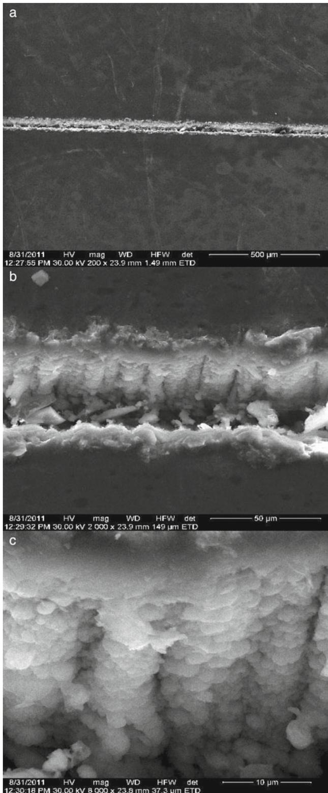
**Figure 5.** SEM micrographs of femtosecond laser mark: (a) general appearance of femtolaser mark, showing discontinuous and massive amorphous Al oxide deposits on each side of central molten area ( $\times 200$ ); (b) sidewalls of mark show a consistent depth of penetration ( $\times 2000$ ) and (c) details of solidification structure of sidewalls which bound channel ( $\times 8000$ ).
