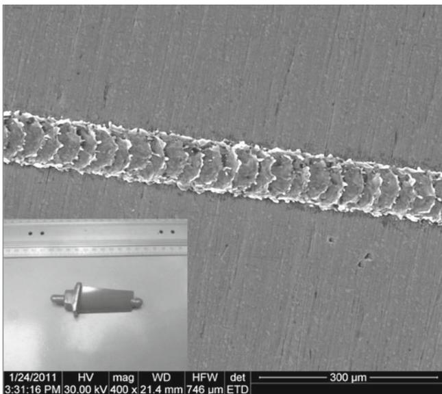
**Figure 1.** Mark's discontinuous and pulsed character, determined by formation of molten material areas ( $\times 400$ ). Figure includes an image of blade.
