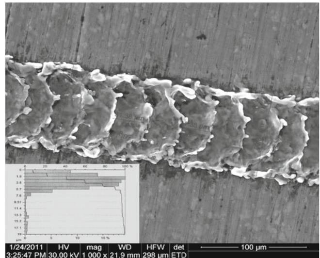
**Figure 2.** SEM image which shows a general view of nanolaser mark. Figure includes superimposing of Abbott–Firestone bearing area curve and surface roughness data.
