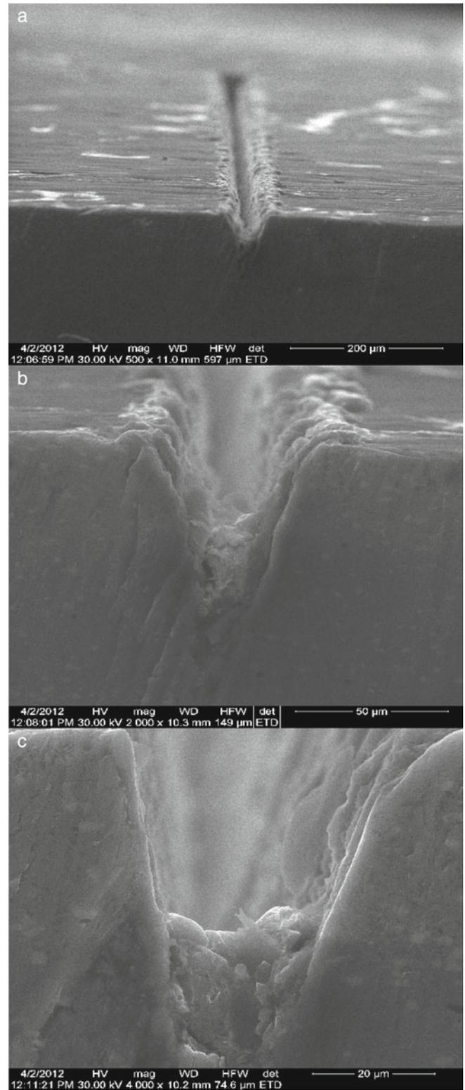
**Figure 6.** Cross-section SEM images of femtosecond laser mark: (a) general cross-section view of femtolaser mark ( $\times 500$ ); (b) sectioning profile and laser treatment resultant deposits ( $\times 2000$ ) and (c) detail showing bottom profile of mark segment. There are no cracks in analysed areas ( $\times 4000$ ).
