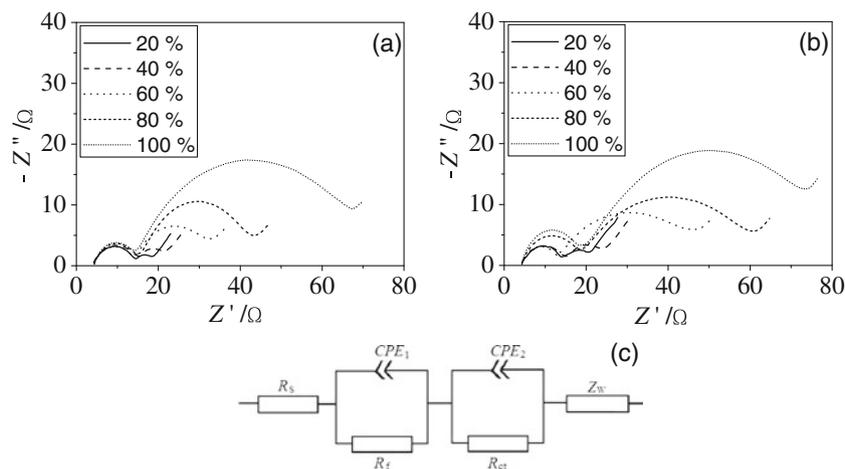
**Figure 7.** Electrochemical impedance spectra of  $\text{LiMn}_{1.95}\text{Al}_{0.05}\text{O}_4$  cathode at different depths of discharge containing 15 wt% PAN (a) and AB (b) and equivalent circuit (c).
