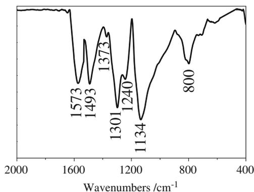
Figure 2. FTIR spectrum of PAN.
