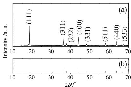
**Figure 1.** XRD pattern of  $\text{LiMn}_{1.95}\text{Al}_{0.05}\text{O}_4$  (a) and standard  $\text{LiMn}_2\text{O}_4$  (b).
