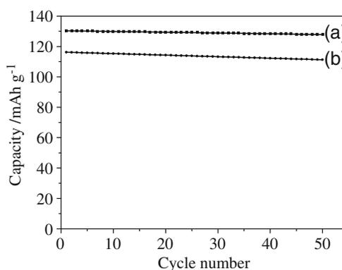
**Figure 8.** Discharge capacity of  $\text{LiMn}_{1.95}\text{Al}_{0.05}\text{O}_4$  cathode using 15 wt% PAN (a) and AB (b) as a function of cycle number.
