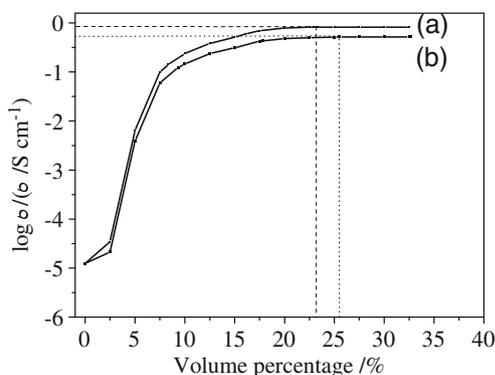
**Figure 4.** Dependence of conductivities of  $\text{LiMn}_{1.95}\text{Al}_{0.05}\text{O}_4$  cathode composite on volume percentage of PAN (a) and AB (b).
