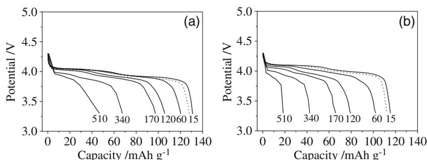
**Figure 6.** Discharge curves of  $\text{LiMn}_{1.95}\text{Al}_{0.05}\text{O}_4$  cathode composite in third cycle under different current densities containing 15 wt% PAN (a) and AB (b). Numbers in figures are their corresponding current density with unit of  $\text{mA g}^{-1}$ .
