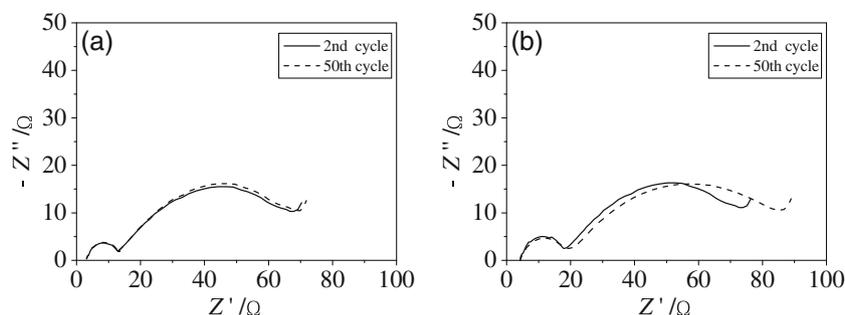
**Figure 9.** Electrochemical impedance spectra of  $\text{LiMn}_{1.95}\text{Al}_{0.05}\text{O}_4$  cathode in full charge state using 15 wt% PAn (a) and AB (b) as conductive additives.
