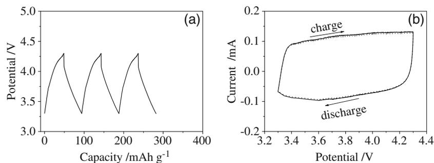
Figure 3. Galvanostatic charge and discharge curves (a) and cyclic voltammograms (b) of PAN in 1st cycle (solid line) and 20th cycle (dotted line).
