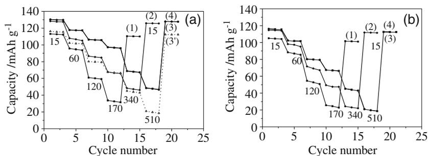
**Figure 5.** Discharge capacities of  $\text{LiMn}_{1.95}\text{Al}_{0.05}\text{O}_4$  cathode composite under different current densities using various mass content of PAN (a) and AB (b) as conductive additive. Dotted line (3') in (a) is that of  $\text{LiMn}_{1.95}\text{Al}_{0.05}\text{O}_4$  cathode composite containing 15 wt% AB. (1) 5 wt%; (1) 10 wt%; (3) 15 wt% and (4) 20 wt%. Numbers in figures are their corresponding current density with unit of  $\text{mA g}^{-1}$ .
