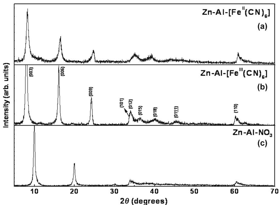
**Figure 1.** PXRD patterns of (a) Zn-Al-NO<sub>3</sub>, (b) Zn-Al-[Fe<sup>III</sup>(CN)<sub>6</sub>] and (c) Zn-Al-[Fe<sup>II</sup>(CN)<sub>6</sub>] LDHs.
