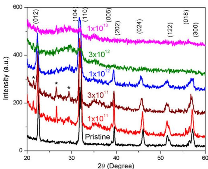
**Figure 1.** Evolution of XRD pattern with 200 MeV Ag ion irradiation fluence for BiFeO<sub>3</sub> thin films grown on Si(100) substrate. Impurity peaks corresponding to Bi<sub>2</sub>Fe<sub>4</sub>O<sub>9</sub> (\* marked) appeared in intermediate ion fluences ( $1 \times 10^{11}$  and  $3 \times 10^{11}$  ions cm<sup>-2</sup>).
