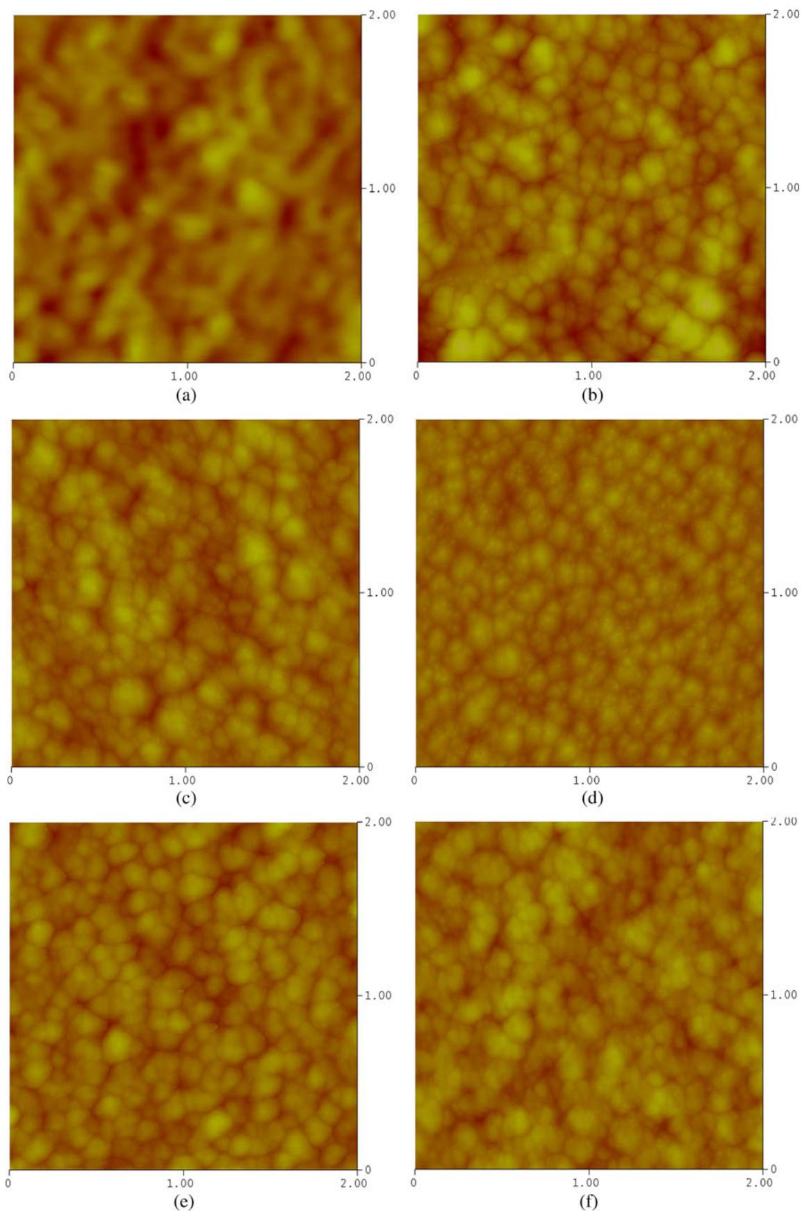
**Figure 3.**  $2 \times 2 \mu\text{m}$  two-dimensional AFM images of (a) pristine film and films irradiated with (b)  $1 \times 10^{11}$ , (c)  $3 \times 10^{11}$ , (d)  $1 \times 10^{12}$ , (e)  $3 \times 10^{12}$  and (f)  $1 \times 10^{13}$  ions  $\text{cm}^{-2}$ .
