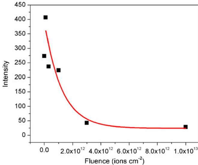
**Figure 2.** Variation of intensity of [110] XRD peak of BFO with ion fluence. Line represents fitting of data points to Poisson equation (1) yielding ion track diameter of 10 nm. Other peaks also show similar variation with ion fluence.
