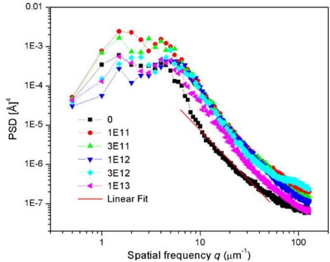
**Figure 5.** Variation of power spectral density (PSD) with spatial frequency,  $q$ , of surfaces for pristine as well as 200 MeV Ag ion irradiated BiFeO<sub>3</sub> films.
