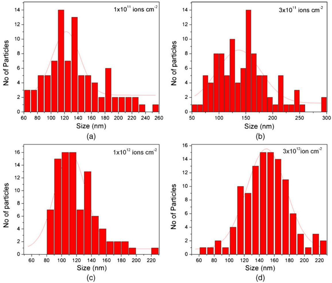
**Figure 4.** Size distribution of surface structures obtained from AFM images of films irradiated with (a)  $1 \times 10^{11}$ , (b)  $3 \times 10^{11}$ , (c)  $1 \times 10^{12}$  and (d)  $3 \times 10^{12}$  ions  $\text{cm}^{-2}$ .
